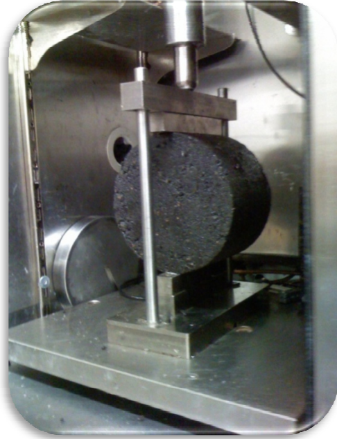
Figure 21 Indirect Tensile Strength Testing Setup
