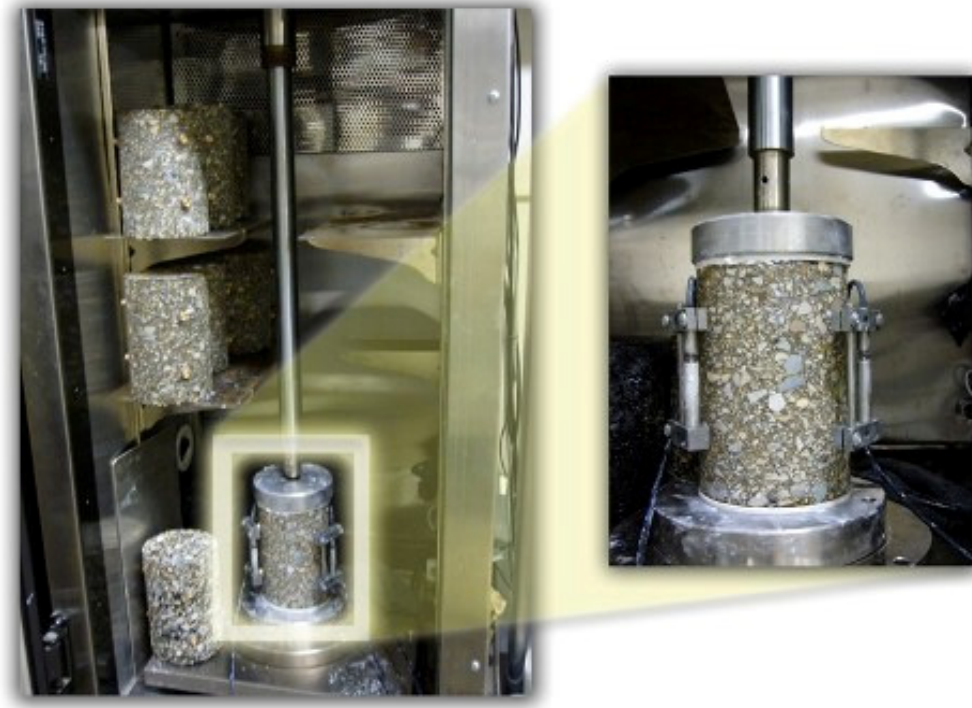
Figure 14 Dynamic Modulus Test Setup
