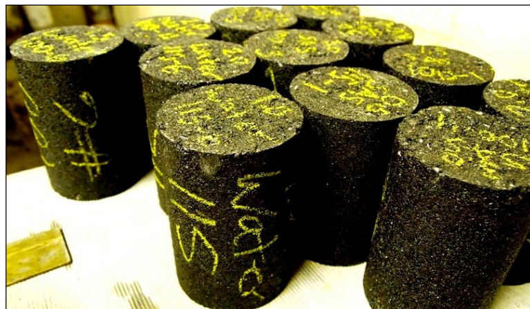
Figure 33 Warm Asphalt Mixture Produced using the Water Foaming Method
