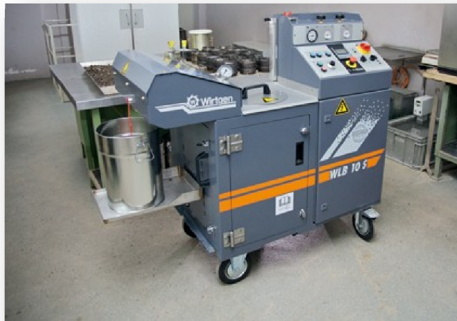
Figure 28 Wirtgen WLB 10 Foaming Nozzle
