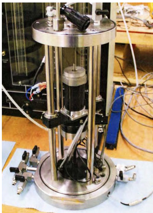
Resonant column apparatus during calibration.
