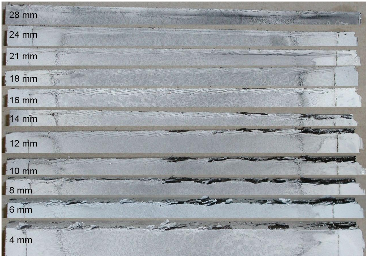
Figure 5. Shelling of a Rail; Shown Are Longitudinal Sections Machined Vertically (parallel to the rail web) at Distances Ranging from 4 to 28 mm from the Gauge Side of the Rail; The Steel Is a 1984 CC CFI Rail Steel
