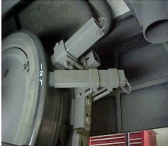
Friction modifier sticks apply products directly to the running surface of the wheel.
