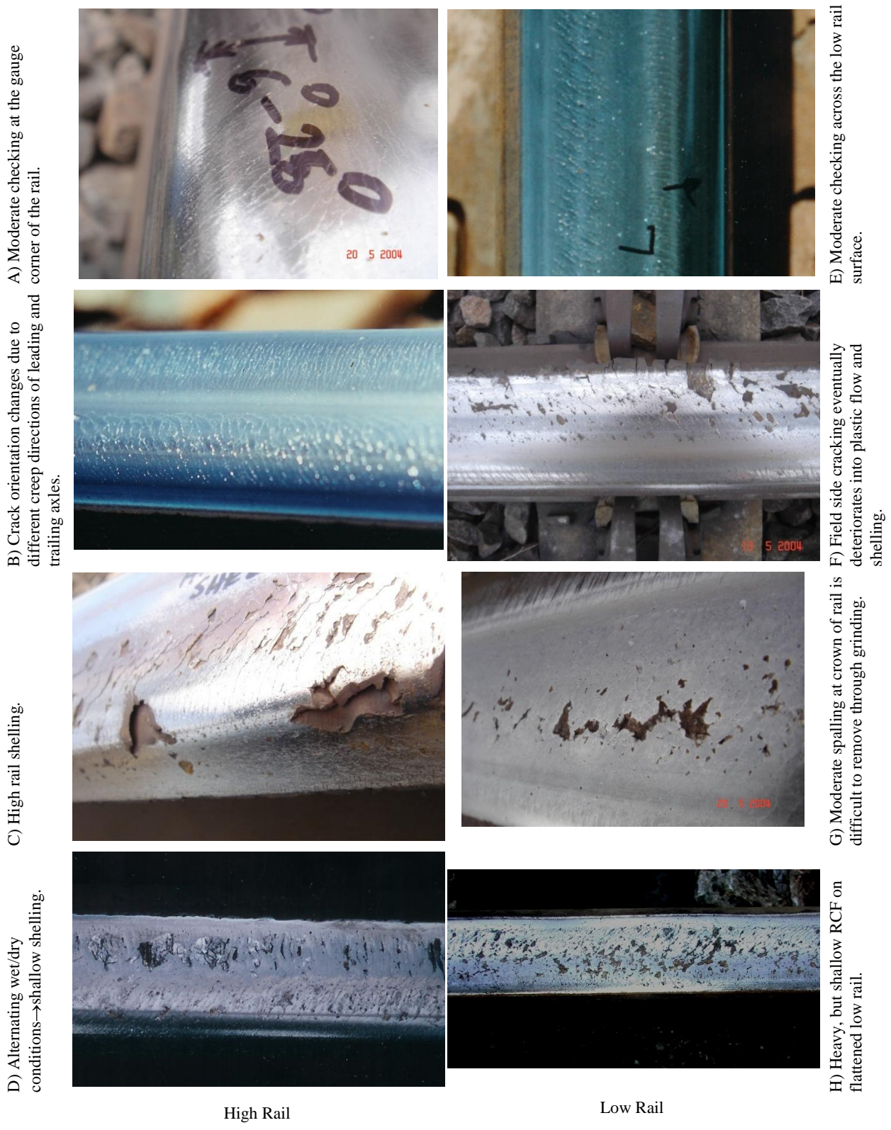
Figure 3. Examples of Typical High and Low Rail Checking and Shelling
