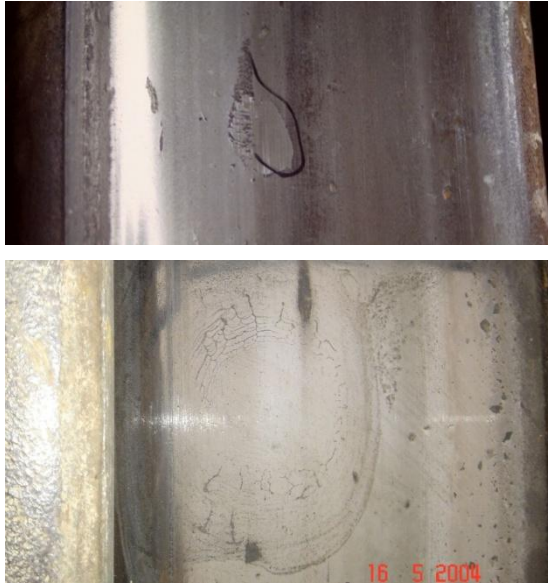
A light martensitic contact patch at a wheel slide location with cracking starting.
