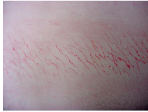
B) Microcracks on the field/rim side of the high-speed wheel.
