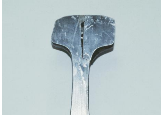
Figure 11. Vertical Split Head Defect
