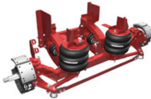
Figure 2-2 Hendrickson Compositelite SC20 ( http://www.hendrickson-intl.com )
