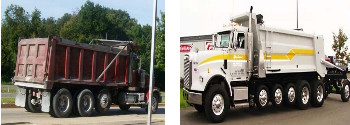
Figure 2-1 Four-axle Dump Truck with Lift Axle (L) and Seven-axle Truck with Triple Lift Axles with a Tag-Along (R)
