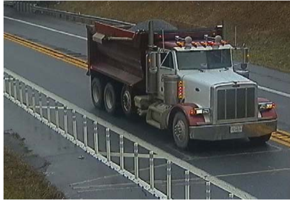
Figure 4-8 Lift Axle truck from Weigh-In-Motion data
