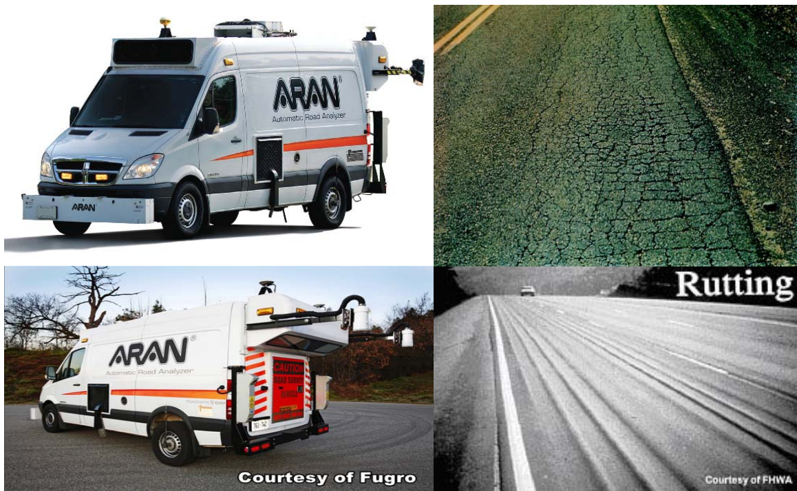
Figure 5 Automatic road analyzer (ARAN) van
