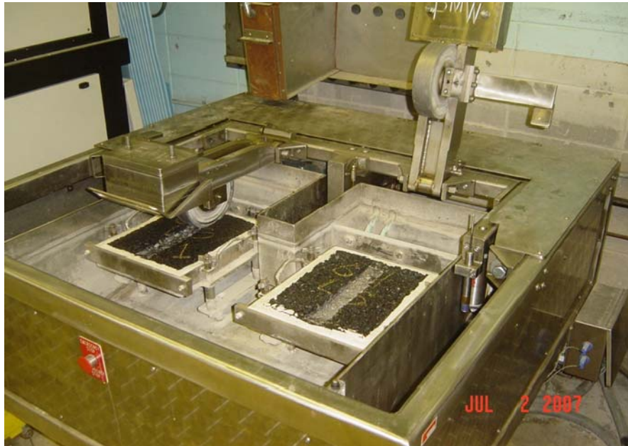
Figure A.2 Hamburg loaded wheel tracking device
