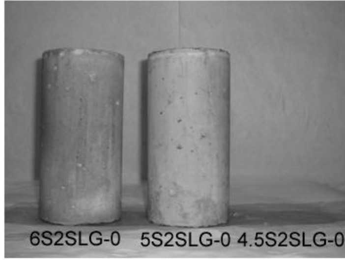
Figure 35: Cylinders to represent the 564 and 470 lbs/yd 3 cementitious content mixes (from left to right) produced during Phase 2 using the Southern aggregate source, St Marys portland cement, and Holcim GGBFS. The 423 lbs/yd 3 cylinder is not pictured.
