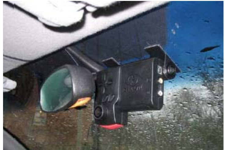
A DriveCam event recorder will record unsafe driving actions. Abrupt accelerations or braking or erratic steering will trigger the system to record 20-second before-and-after video and audio clips to determine what happens immediately before an incident.
