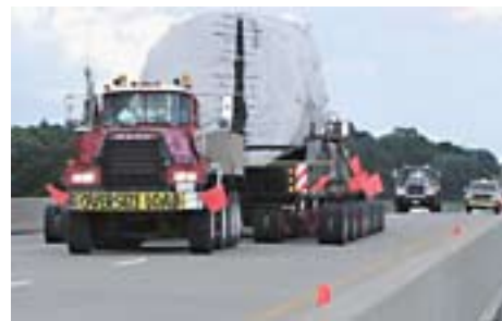
Figure 6 - A permitted vehicle crosses a bridge on U.S. 18 in Cerro Gordo County during bridge testing.
