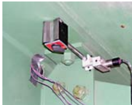
Figure 1 - Conventional electronic-based displacement and foil-strain gauges used to evaluate structural connection response.
