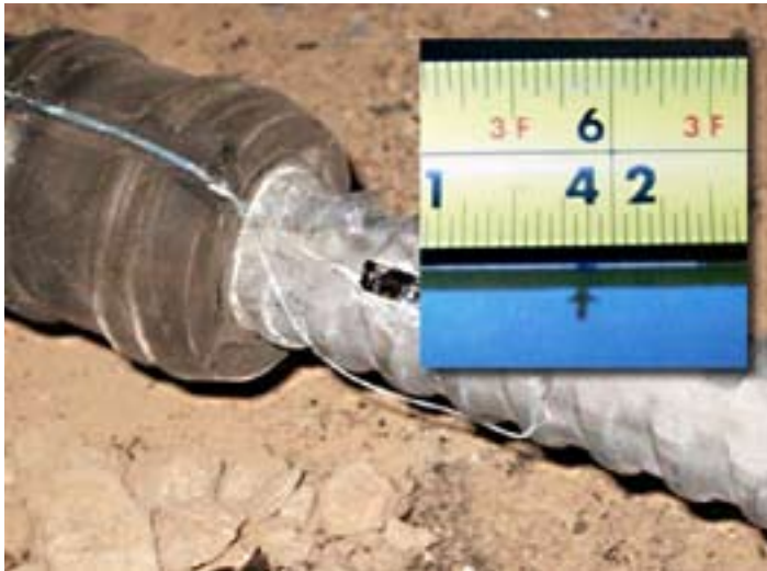
Figure 3 - Uncoated fiber on hanger rod with sensor (in black package) bonded to the specimen; the actual fiber-optic sensor within the fiber is extremely small (designated by arrow pointing to blue region)
