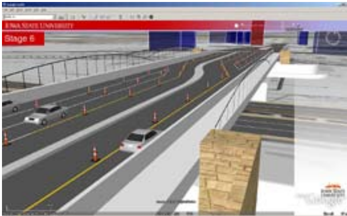
Figure 8 – Actual work zone configuration for the final stage of construction
