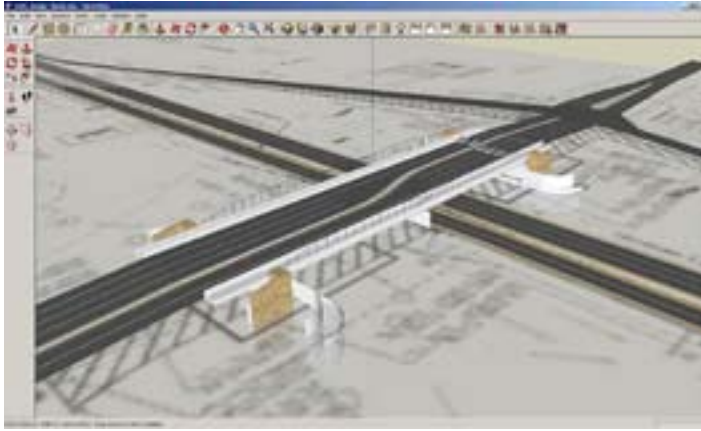
Figure 2 – Completed 3-D model of a six-lane bridge over the base 2-D drawings
