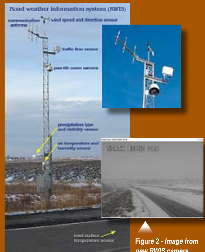
Figure 1 - RWIS tower (with labels) and camera close-up
