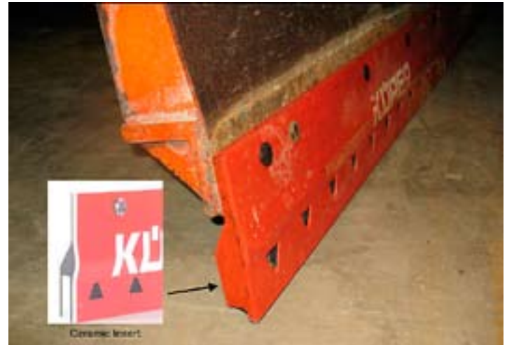
Figure 20 - Experimental blade by Gummi-Küper (Germany) with ceramic insert
