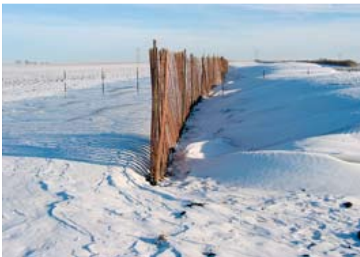
Figure 28 - Field testing using lath snow fence
