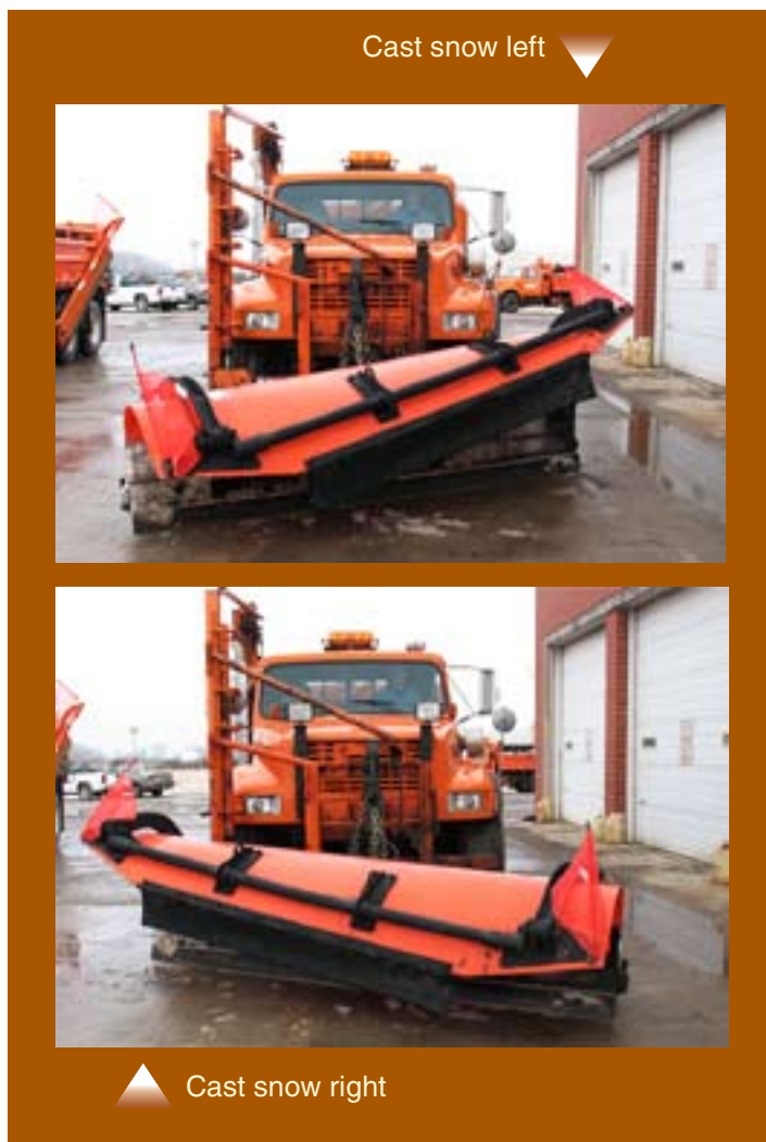
Figure 19 - Demonstration showing the reverse-a-cast plow adjusted to control snow discharge
