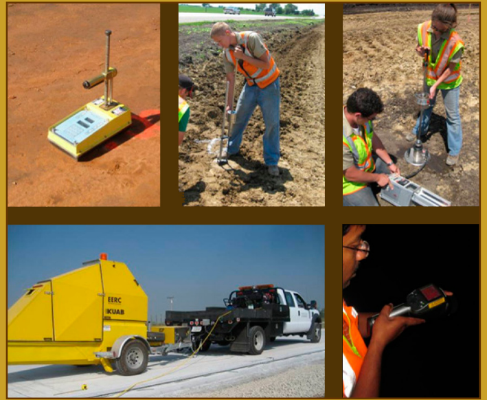
Figure 6 – Different in situ testing methods employed on the demonstration projects – (from top left to bottom right) nuclear density gauge, dynamic cone penetrometer, lightweight deflectometer, falling weight deflectometer and thermal camera
