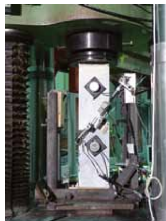
Figure 19 – Setup used for UHPC- NC shear-friction interface testing
