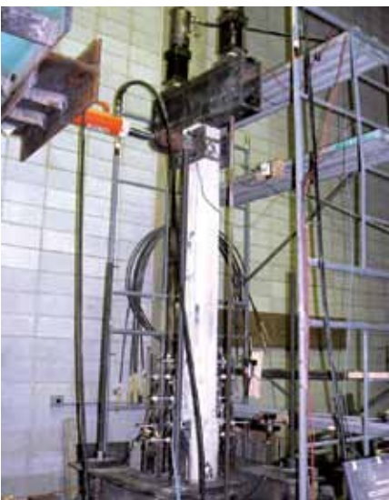
Figure 11 – Setup of UHPC test unit with a length of 10 feet and full-scale section properties; the tests allowed validation of the moment-curvature behavior of the UHPC pile
