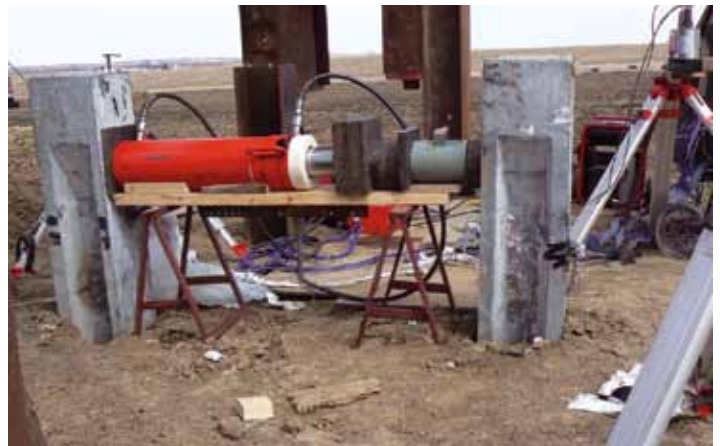
Figure 13 – Testing of a full-scale beam and small-scale shear beams
