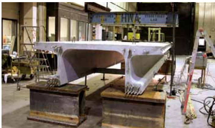
Figure 5 – Second generation pi-shaped girder specimen prior to test (25 foot long, full scale) at the FHWA Turner-Fairbank Laboratory. The girder testing program was done in conjunction with the research and testing at ISU.
