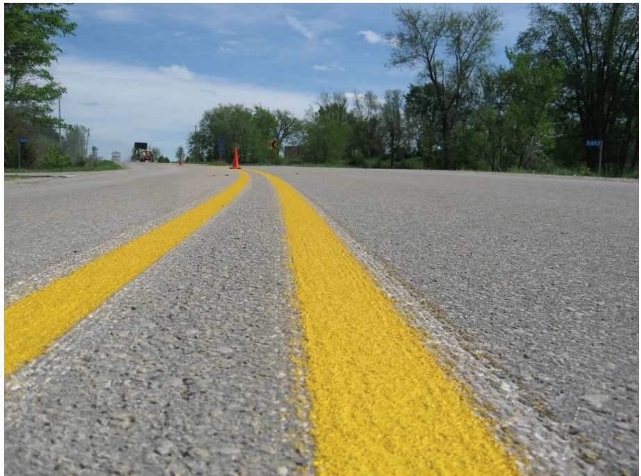
A pavement marking test deck in Dallas County evaluating experimental centerline markings placed within a groove - Photo: Neal Hawkins, Iowa State University/CTRE
