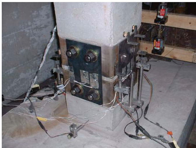
Segmented column joint and foundation prior to testing
