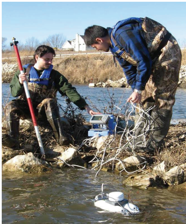
Students use an Eagle Fish Elite 480 fish-finding sonar/GPS mounted to a tow fish for depth measurements on the Raccoon River near Adel, Iowa.
