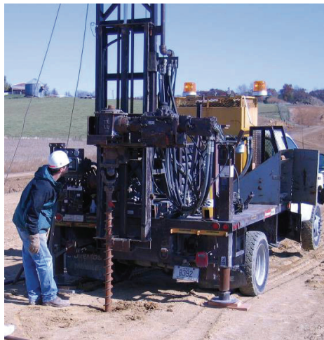
Shelby tube soil sampling in the field
