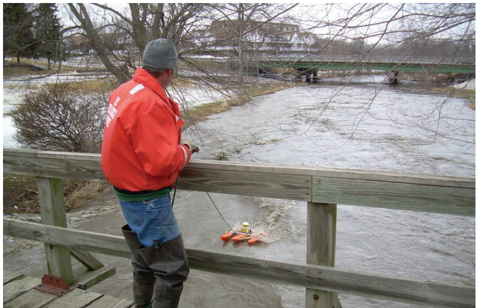
Acoustic Doppler Current Profiler (ADCP) in use at Duck Creek during Davenport flood in March, 2007 - Photo: U.S. Geological Survey
