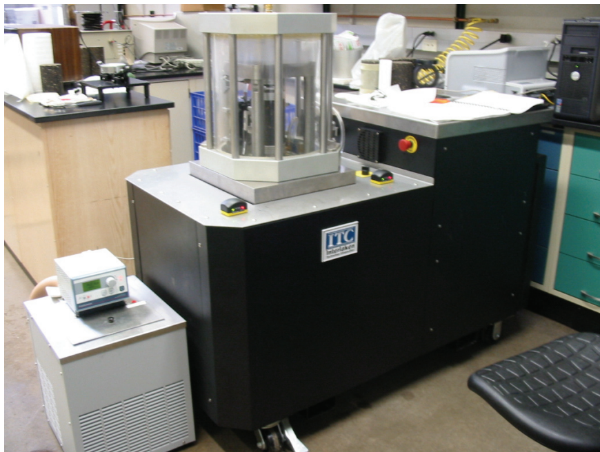
CIR-emulsion mixtures are tested using Interlaken Performance Testing Equipment
