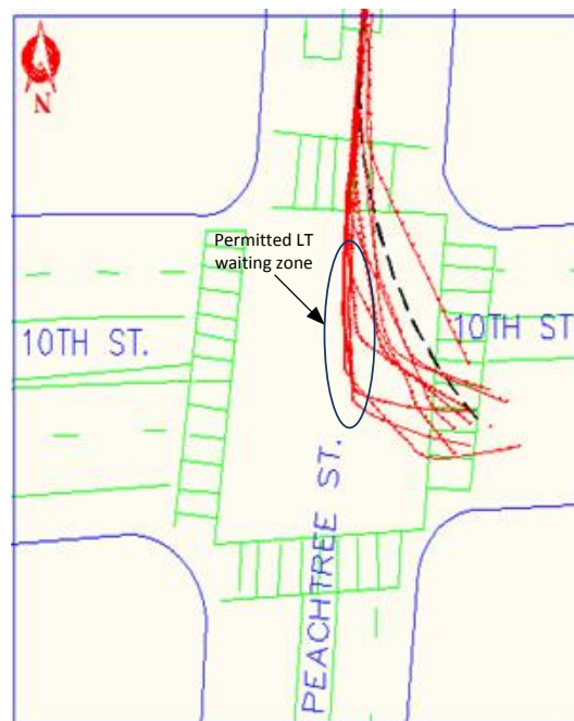
Figure 2: Turning path for left-turning vehicles - permitted LT mode SB Peachtree Street at 10 th Street intersection (12:45 PM - 1:00 PM).
