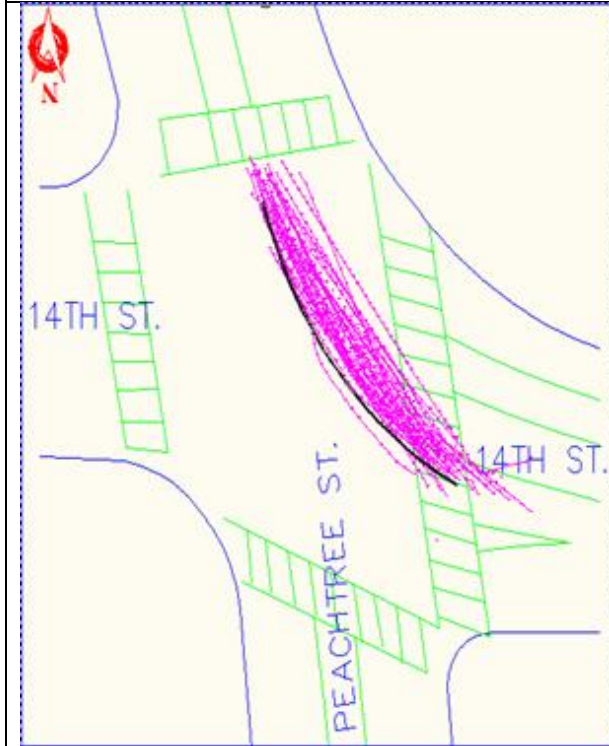
Peachtree Street and 14th Street Intersection (SB) Protected LT mode – 12:45 PM – 1:00 PM
