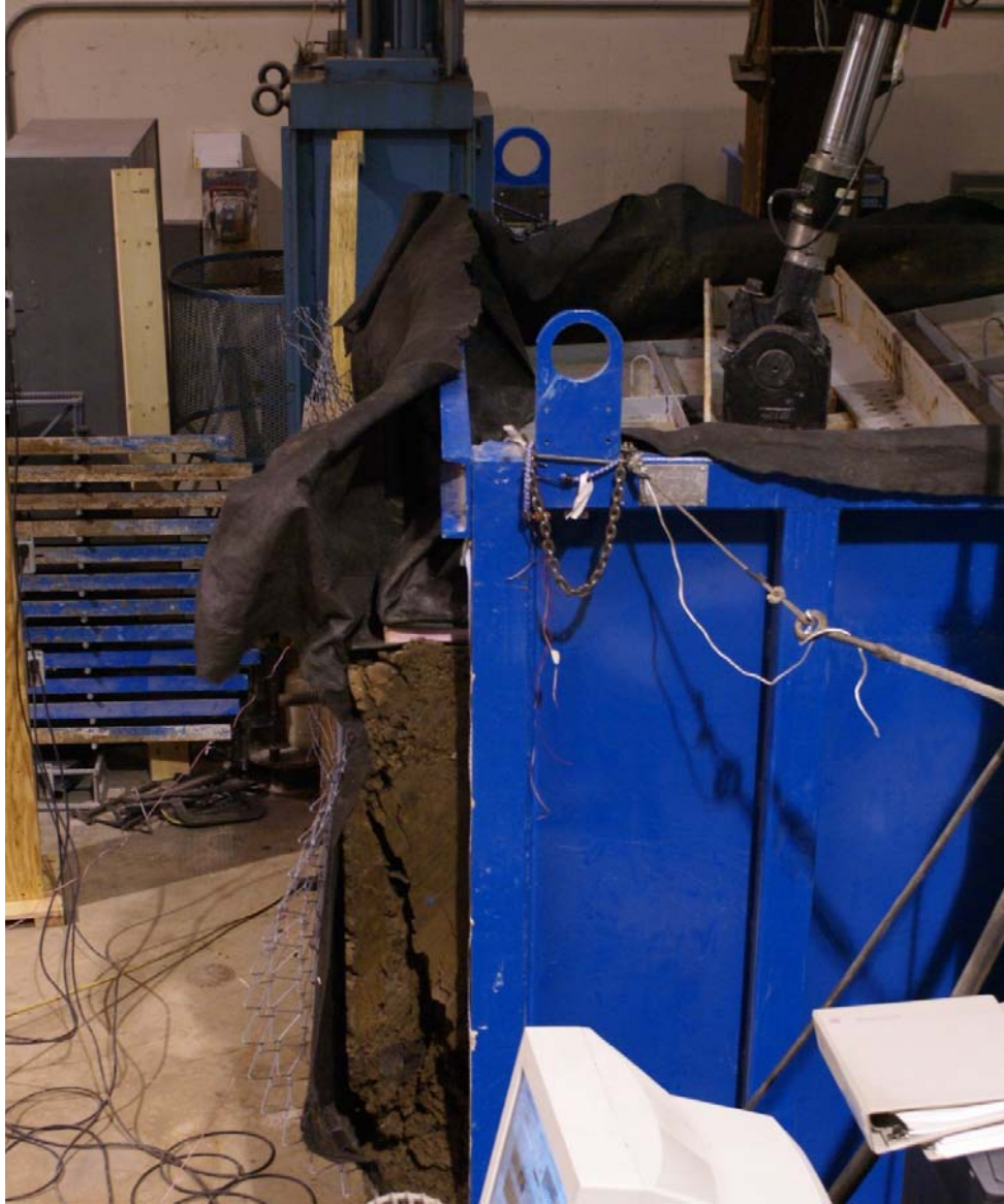
FIGURE 5.13 Side view after failure of nail connections
