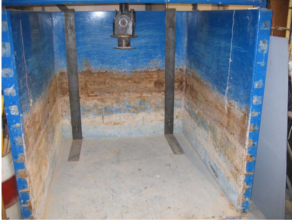
FIGURE 4.12 Large geotechnical test box
