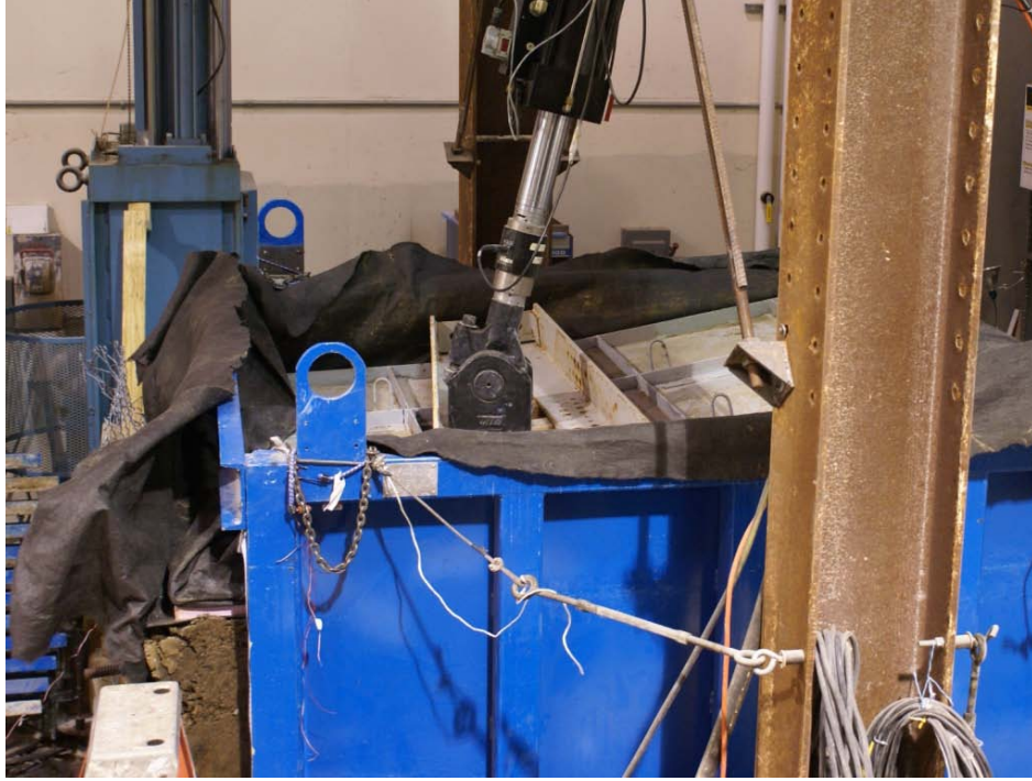
FIGURE 5.11 Side view after failure of nail connections
