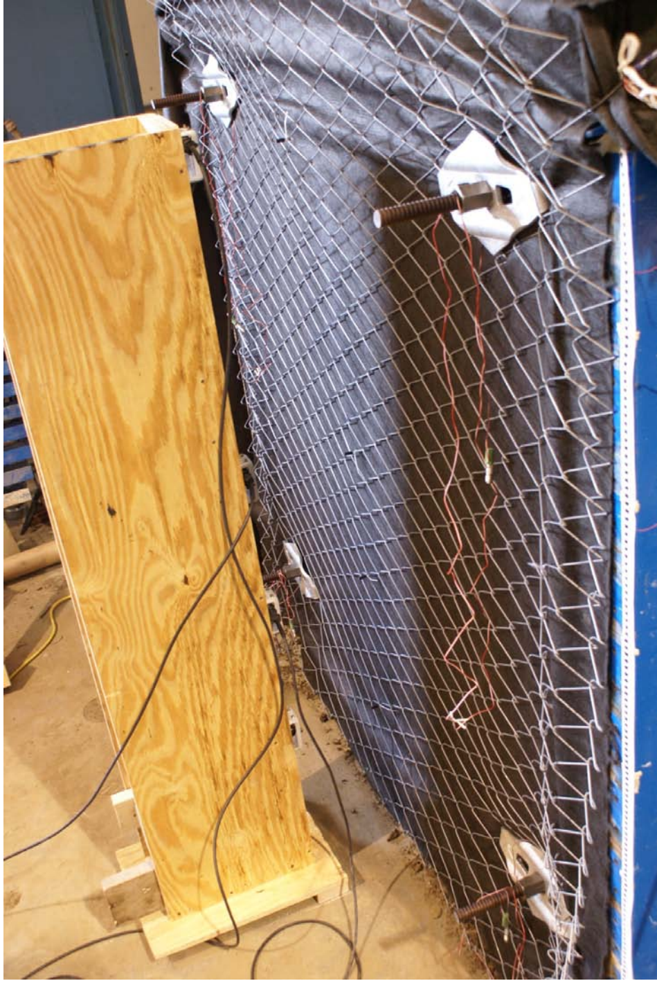
FIGURE 5.6 String pots on the soil face
