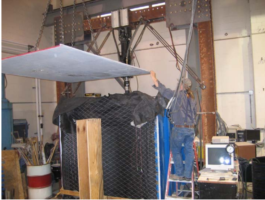
FIGURE 5.7 Installing the steel plate on the top of the soil-nailed wall
