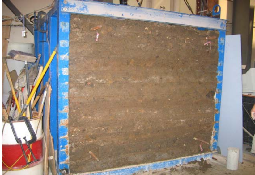
FIGURE 5.4 Completed soil wall—the front face
