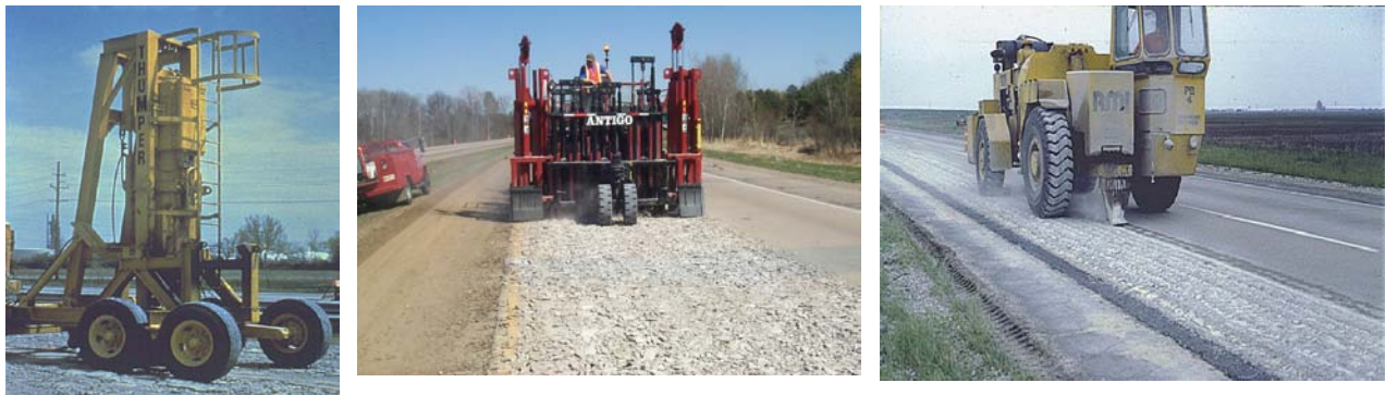
Figure 1. Pavement demolition equipment: a) diesel hammer, b) multi-head pavement breaker, and c) resonant breaker (Hoerner et al. 2001).
