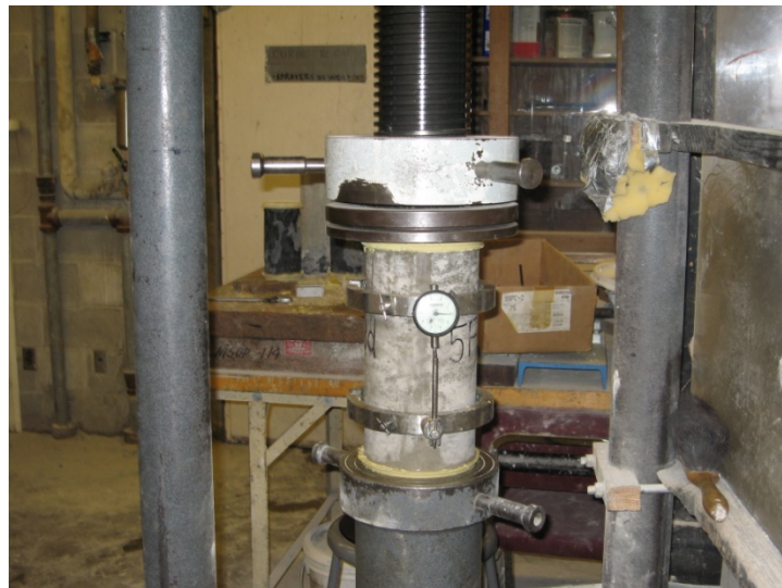
Figure 5.7 Ultimate Strength/Stiffness Test Apparatus
