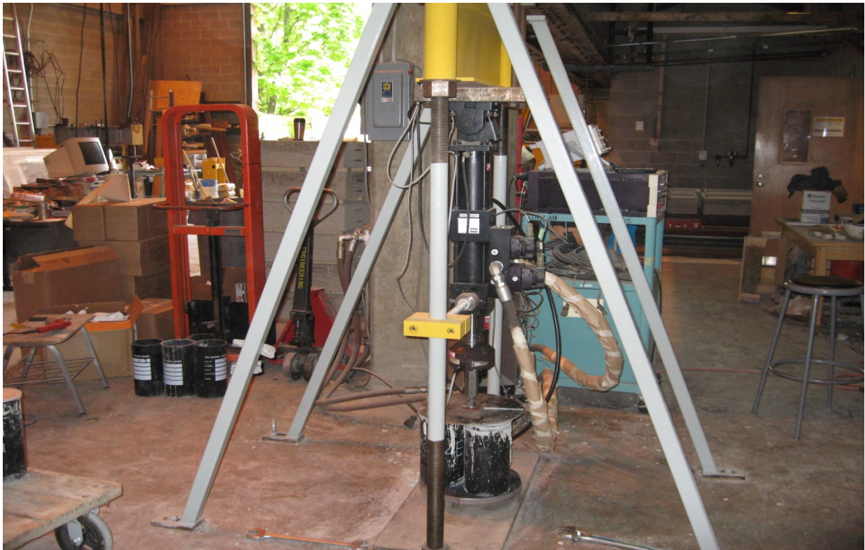
Figure 5.4 Laboratory Vibration Test Apparatus (for Cylindrical Specimens)
