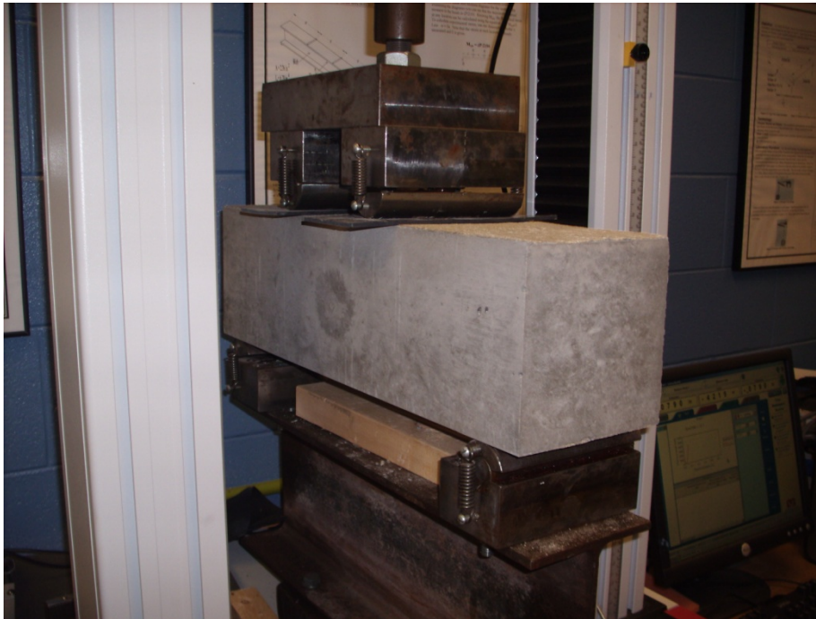
Figure 5.15: Simple beam with third-point loading (close-up)
