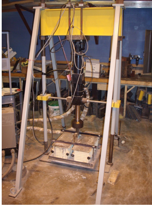
Figure 5.12: Laboratory Vibration Test Apparatus (for Beam Specimens)
