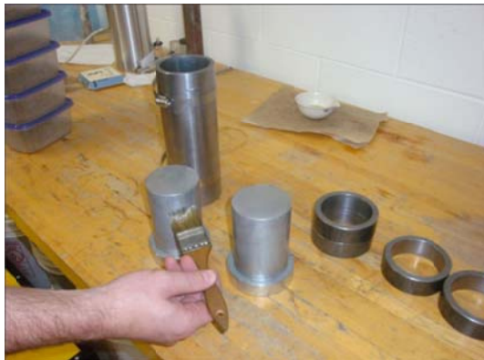
(c) Lubricating split mold
