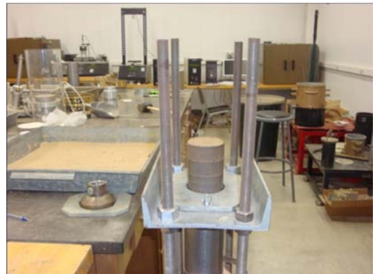
(f) Jacking soil specimen
