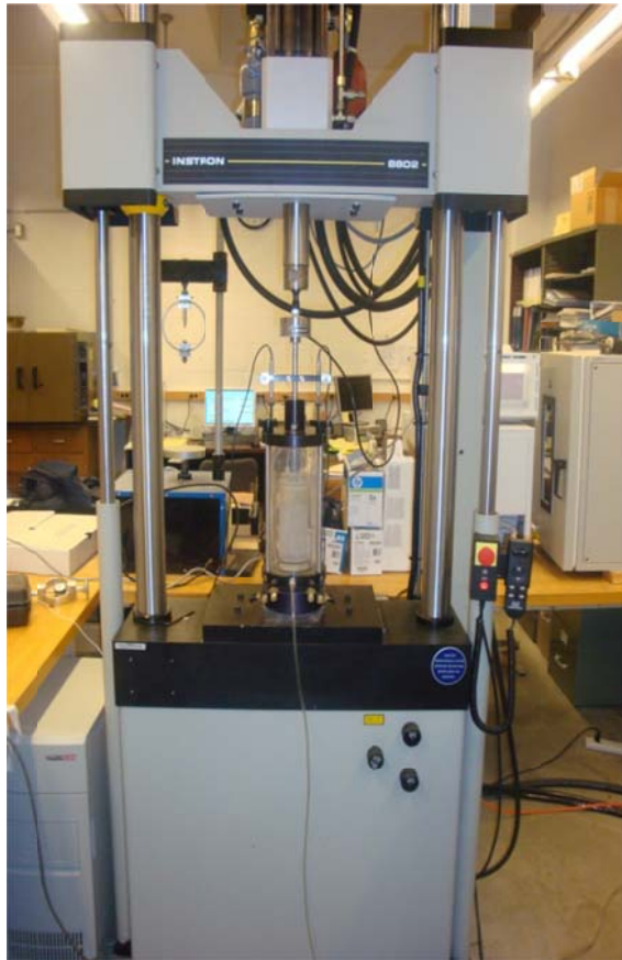
Figure 2.2: Repeated load triaxial test set up and Instron 8802
