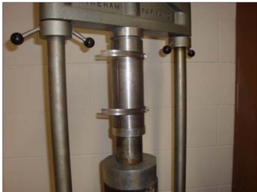
(e) Applying static compaction
