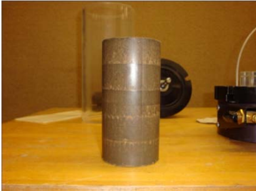
(a) Compacted specimen
