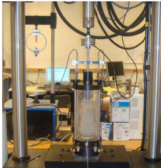
(c) Seating soil specimen on base
