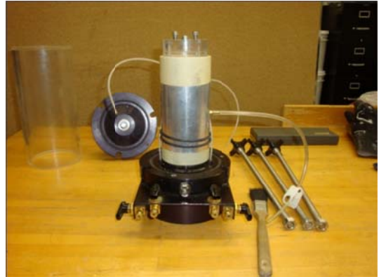
(b) Housing specimen in a membrane
