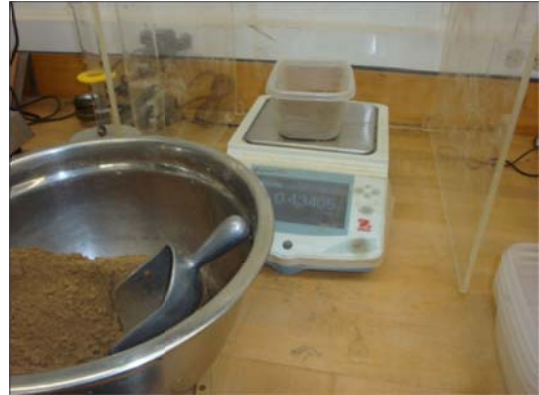
(b) Weighing soil lift for compaction
