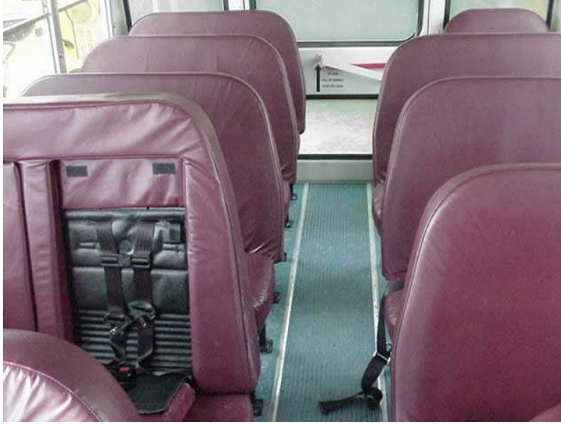
Figure 4. Type A school bus interior with child seat (courtesy of Ankeny School District)
