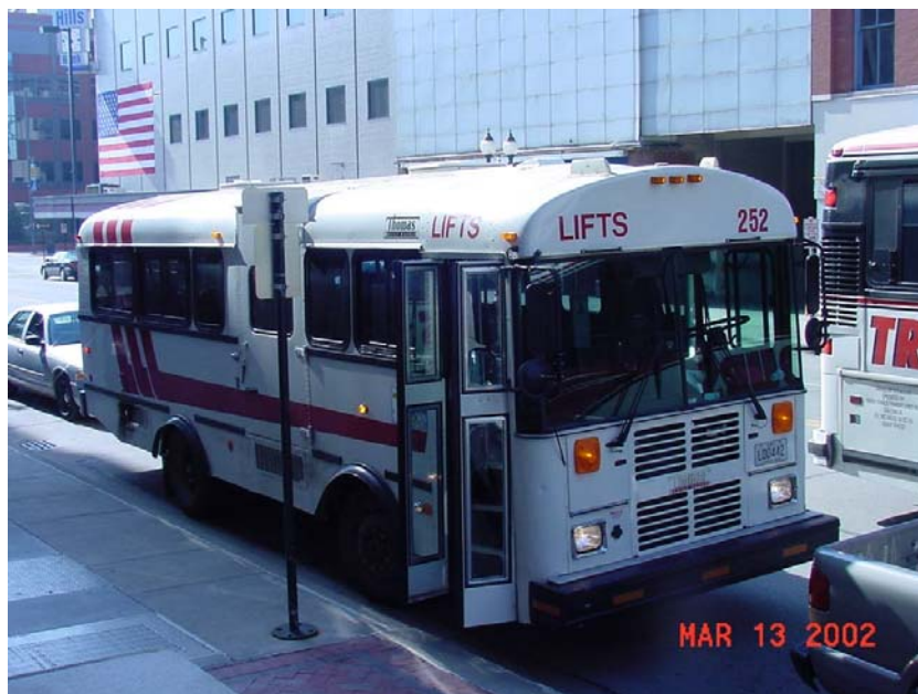
Figure 18. Medium-duty transit bus similar to Type D school bus (courtesy of Linn County LIFTS)
