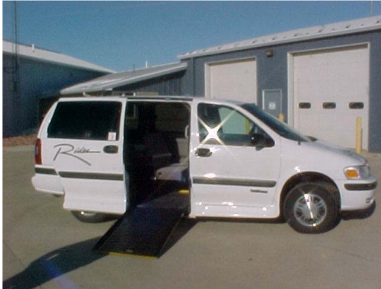
Figure 23. Transit minivan equipped with wheelchair ramp in conformance with ADA accessibility standards (courtesy of Region 3)
