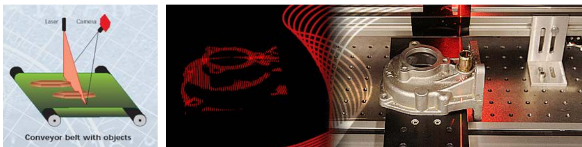
Figure 4 Laser Line based 3D Imaging Technique on a Conveyor Belt ( http://www.adept.net.au/news/newsletter/200810-oct/3D_Camera.shtml )
