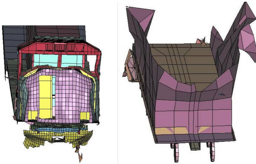
Figure 23. Locomotive and Hopper Car Damage from Simulation
