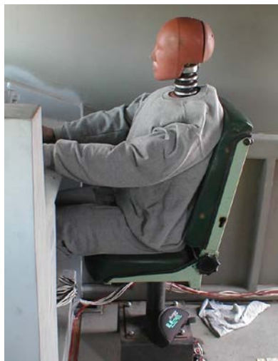
Figure 37. ATD Position in Cab of Locomotive
