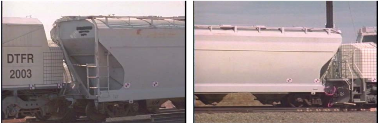
Figure 12. Locomotive Nose Contacts Covered Hopper Body
