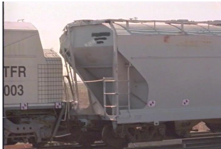
Figure 11. Locomotive Vertical End Plate Contacts Front Truck
