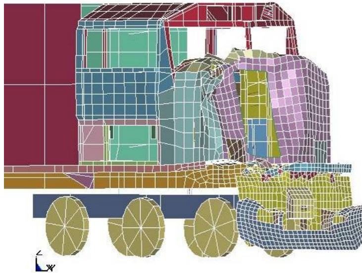
Figure 14. Simulated Damage to Locomotive
