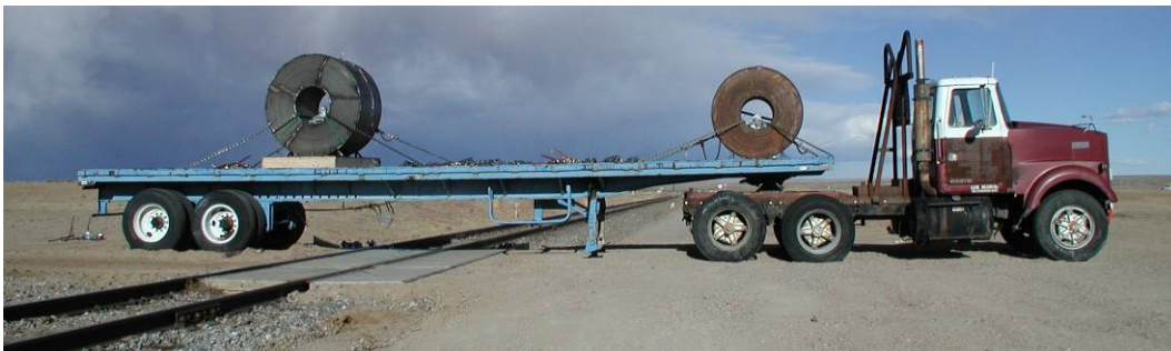
Figure 9. Loaded Trailer with Steel Coils before Collision
