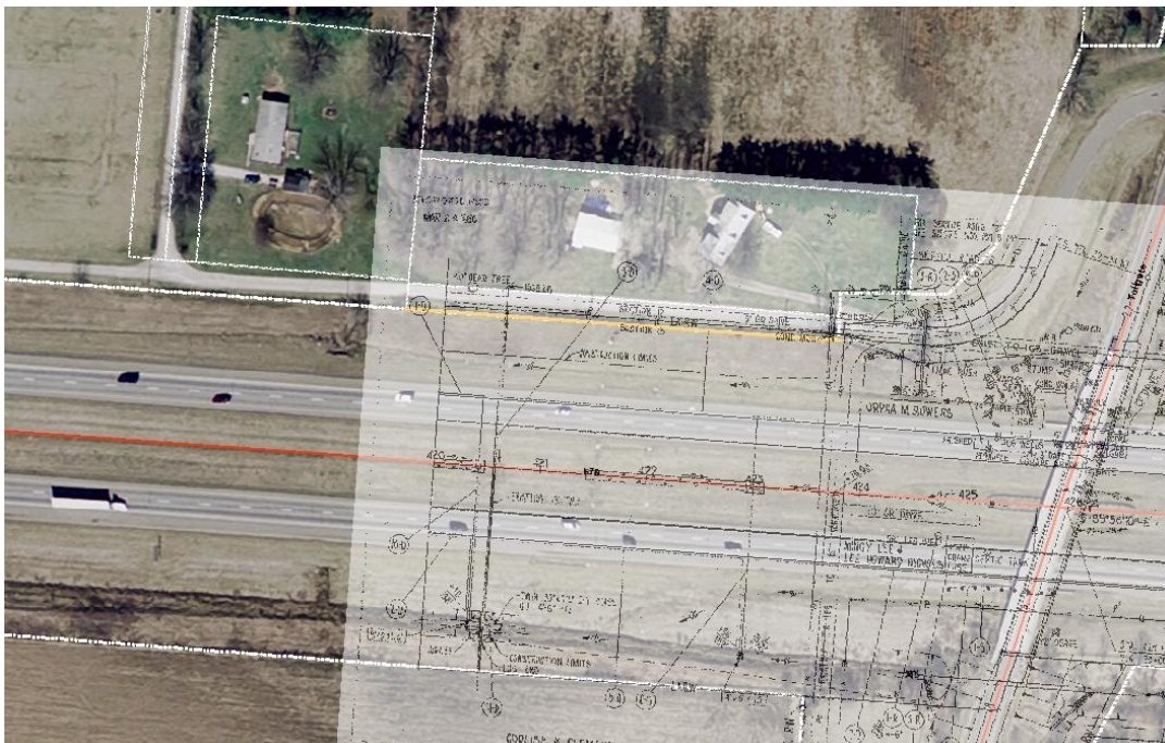
Figure 9.3: Original Plans Overlaid Recent Aerial Photo with Highway Centerlines and Barrier Baseline
