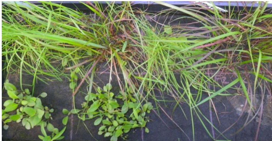
Figure 8.3: Emergence of Grasses and Forbs on Deltalok Bag Sections in Tray Studies
