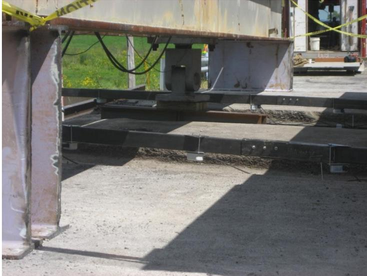
**Figure 37: Steel Tubes with String Potentiometers**
