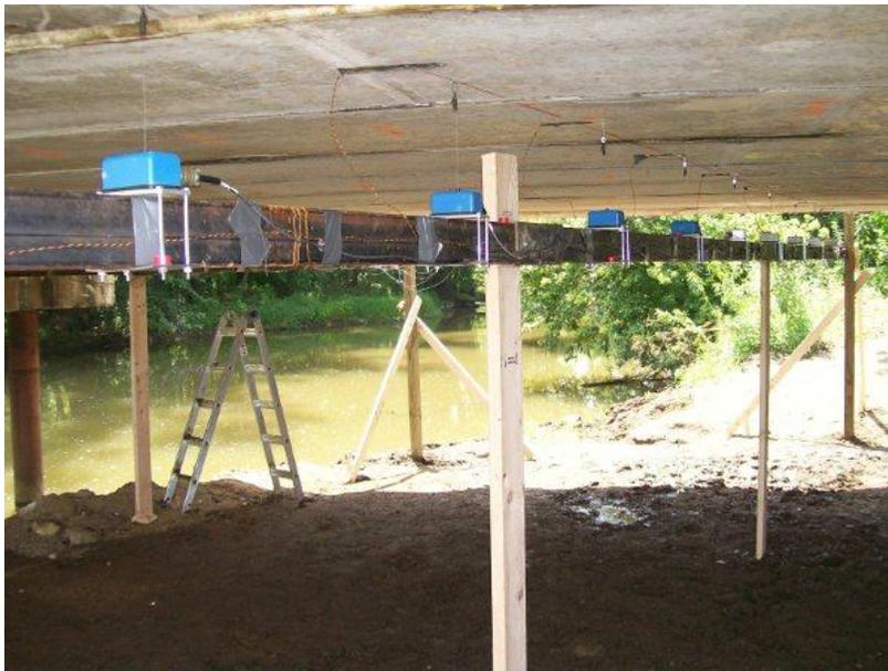
**Figure 21: Instrumentation and Supporting Frame**
