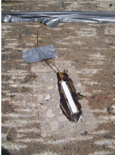
**Figure 18: Installed Strain Gage**
