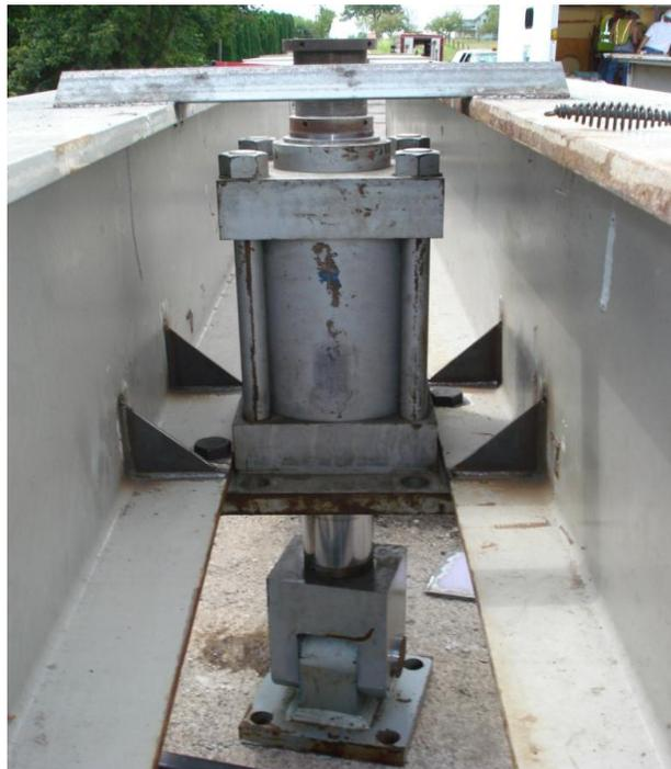
**Figure 32: Hydraulic Cylinder**
