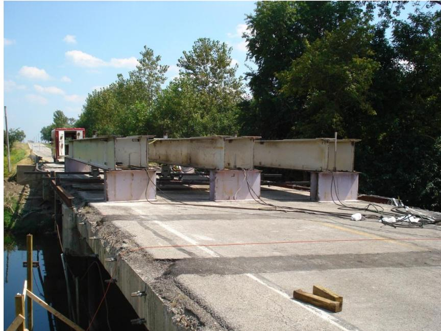
**Figure 31: Test Frames on Span 1**
