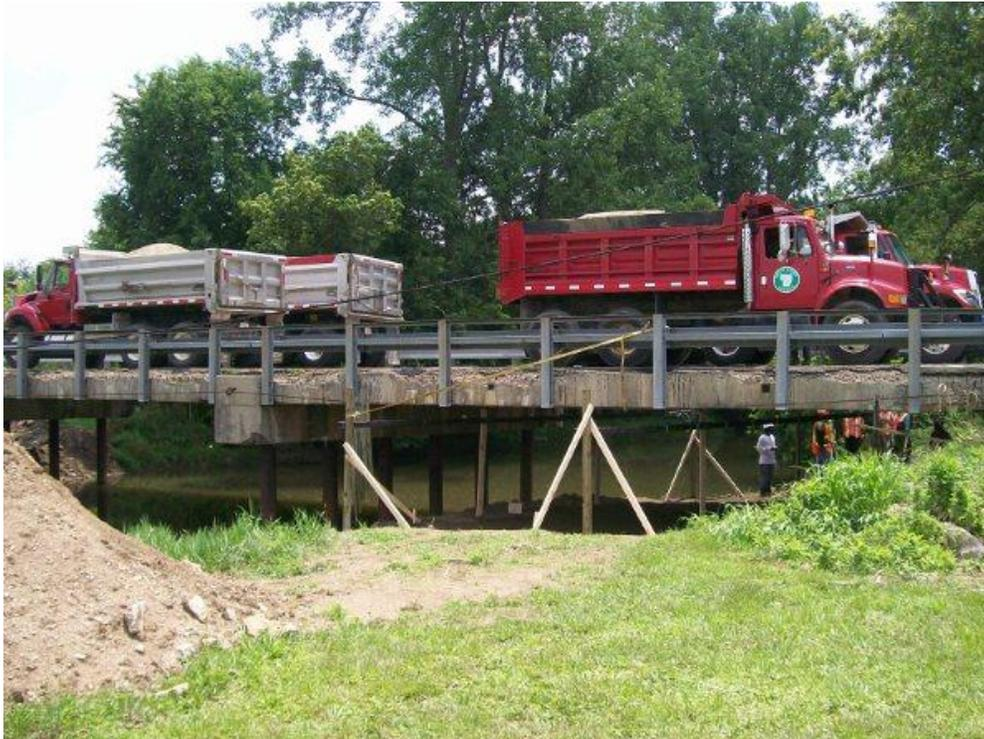
**Figure 27: Truck Loading (Max -M)**
