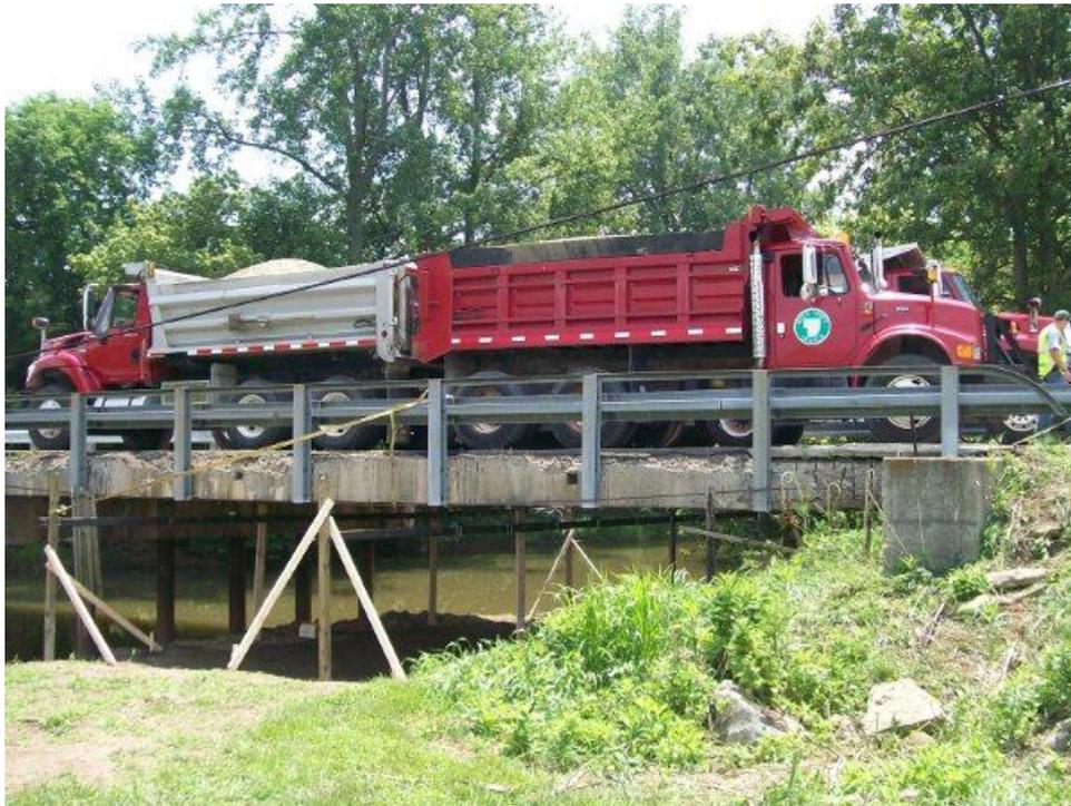
**Figure 25: Truck Loading (Max +M)**
