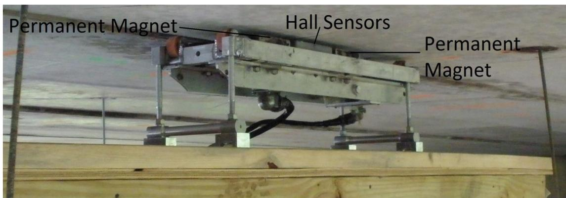
**Figure 15: MFL Sensing Equipment**
