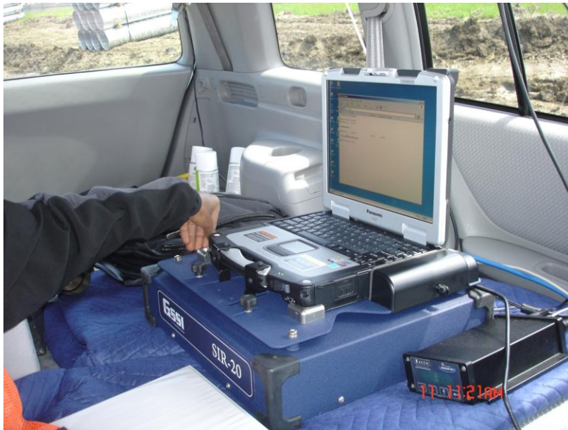
Figure 17. Control Unit, Data Acquisition System and GPS Receiver
