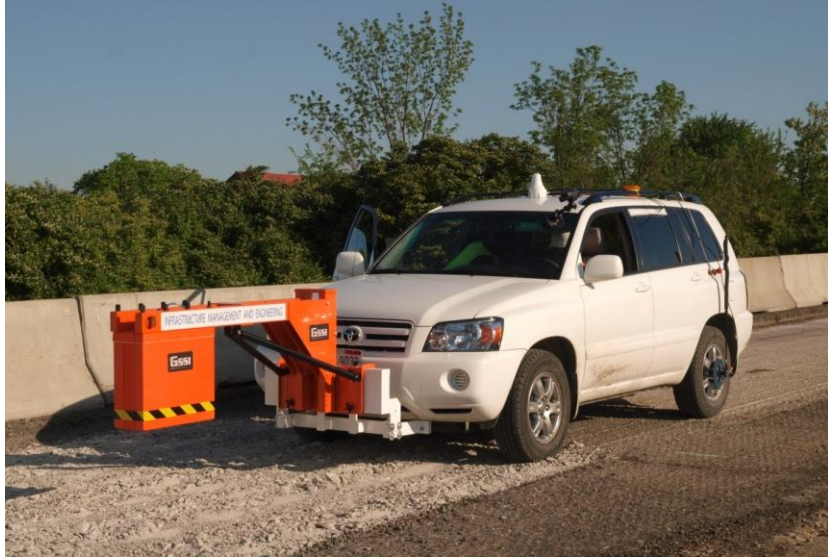
Figure 16. GPR Device in Operation on R/R Project
