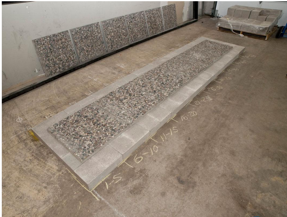
Figure 33. Gravel Paver Block Representing Fully Rubblized Layer
