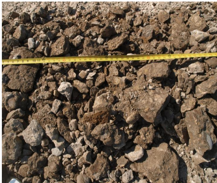
Figure 26. Observed Particle Sizes at the Bottom on Concrete Slab in a Test Pit
