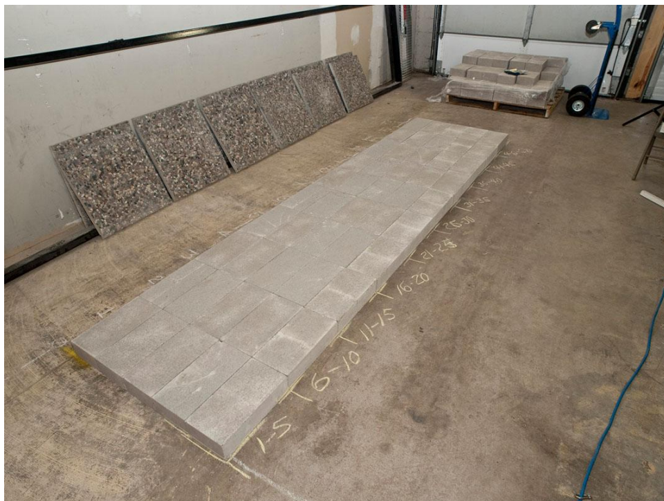
Figure 32. Concrete Blocks Representing Partially Rubblized Fragments
