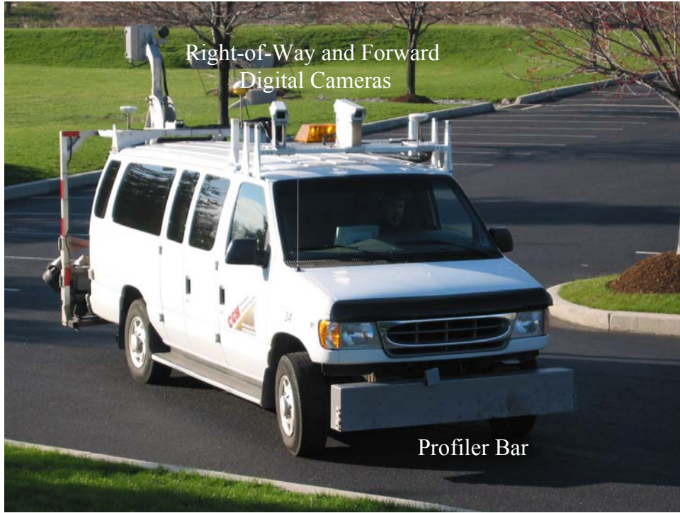
Figure 2-2. Front view of digital survey vehicle
