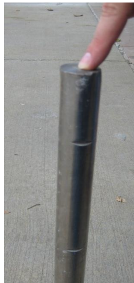
Figure 4.2.1.2 – Dowel bar for bearing systems
