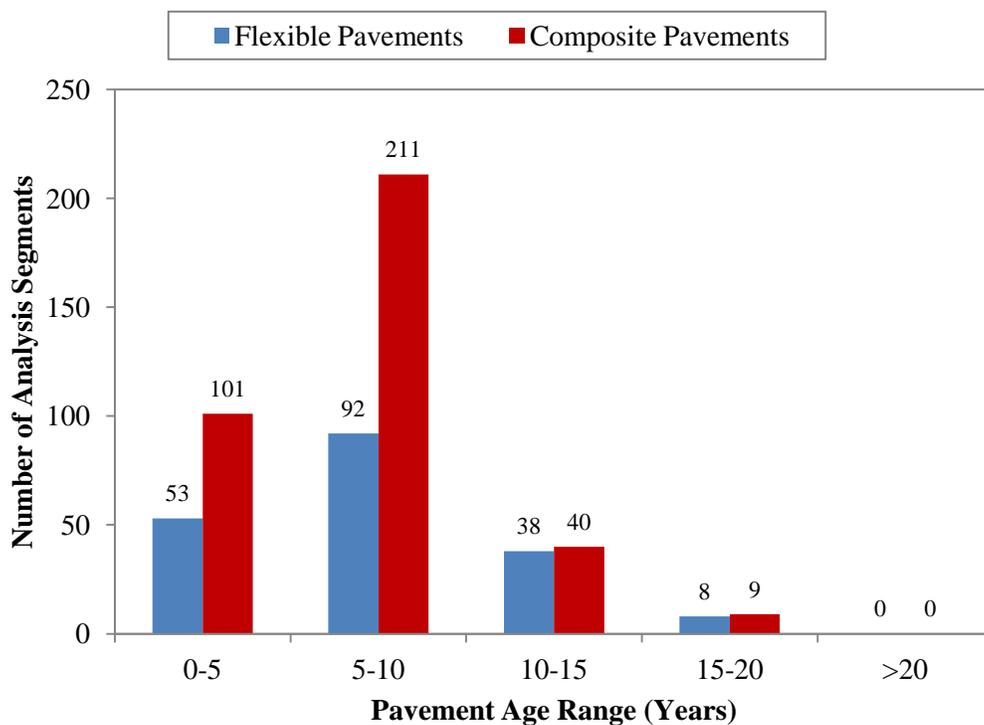
Figure 4.13. Pre-treatment pavement age distribution for double microsurfacing treatments.
