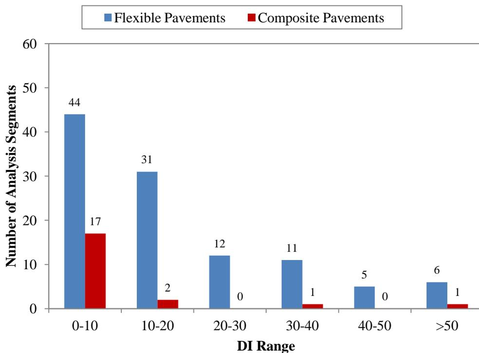
Figure 4.3. Pre-treatment pavement condition distribution for single chip seals.
