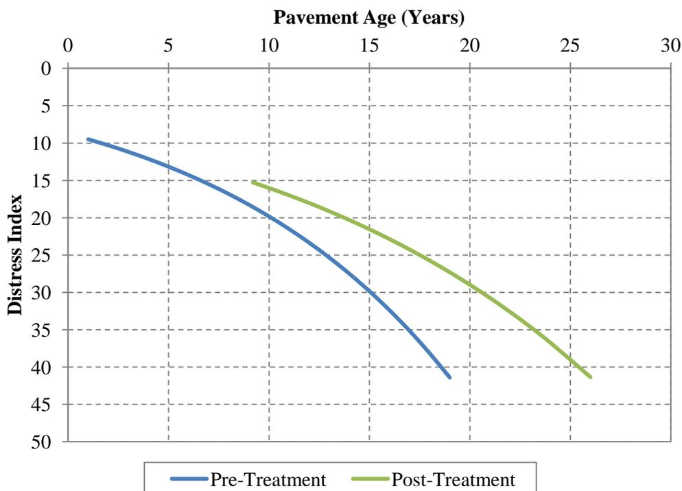
Figure 4.10. Pre- and post-treatment pavement performance – double chip seal on flexible pavements (all zones).
