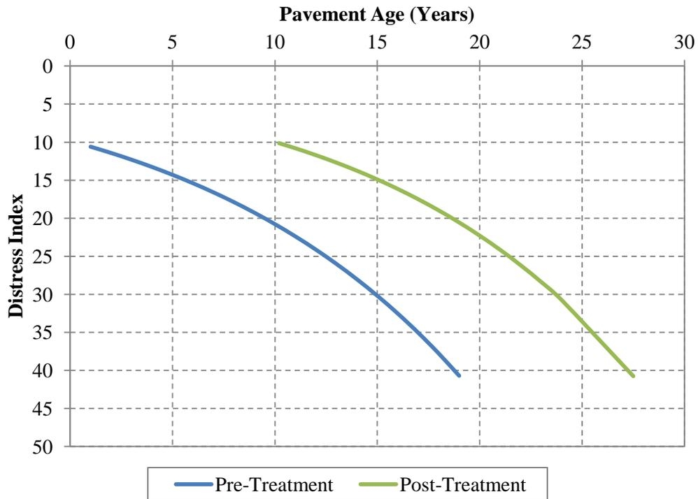
Figure 4.36. Pre- and post-treatment pavement performance – HMA mill and overlay on composite pavement (Zone 1).
