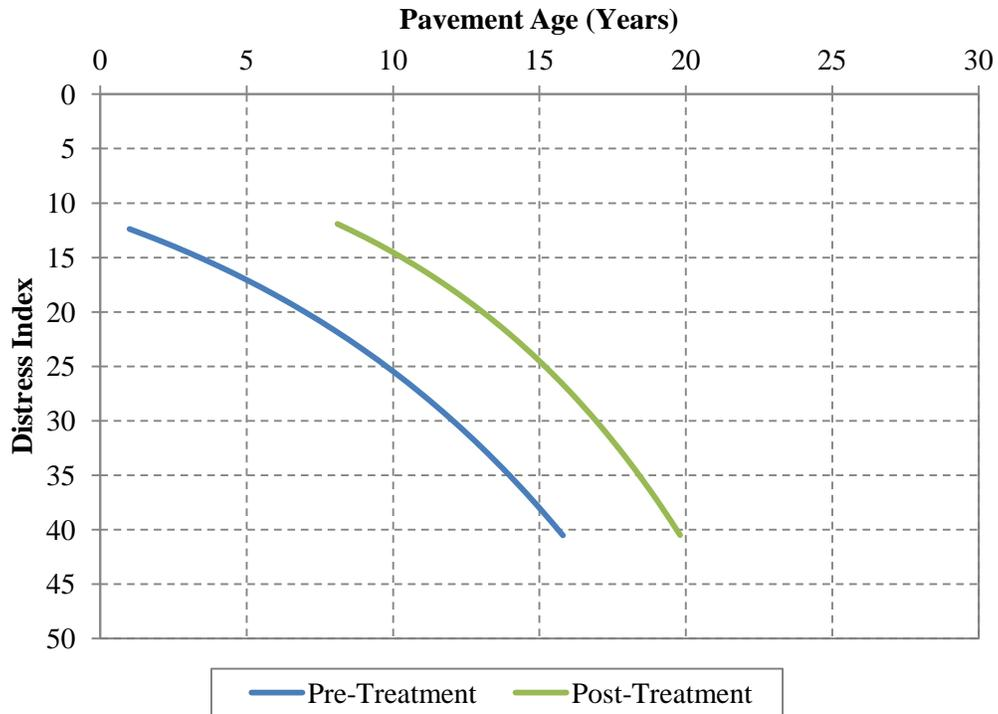
Figure 4.41. Pre- and post-treatment pavement performance – HMA overlay on flexible pavement (Zone 2).
