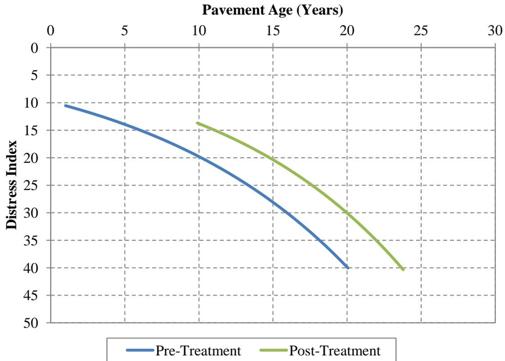
Figure 4.35. Pre- and post-treatment pavement performance – HMA mill and overlay on composite pavement (all zones).
