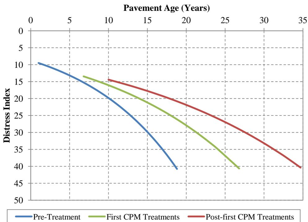
Figure 5.10. Pre- and post-treatment pavement performance on flexible pavement (all zones).
