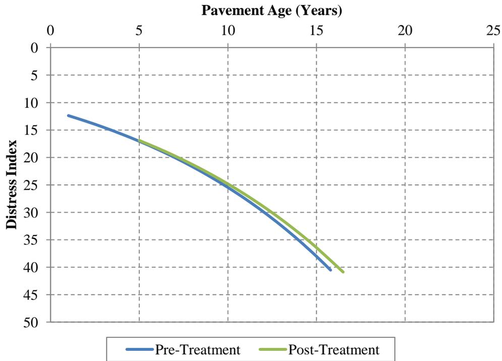
Figure 4.25. Pre- and post-treatment pavement performance – HMA crack treatment on flexible pavement (Zone 2).
