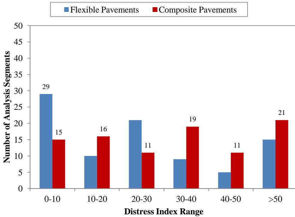
Figure 4.38. Pre-treatment pavement condition distribution for HMA overlay.
