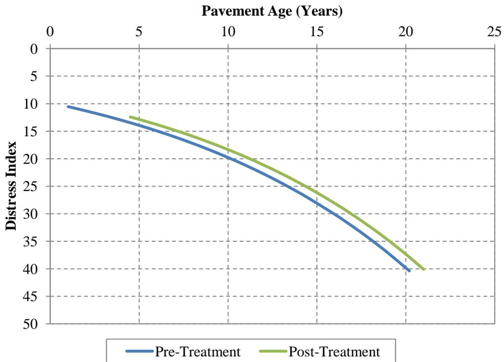
Figure 4.26. Pre- and post-treatment pavement performance – HMA crack treatment on composite pavement (all zones).
