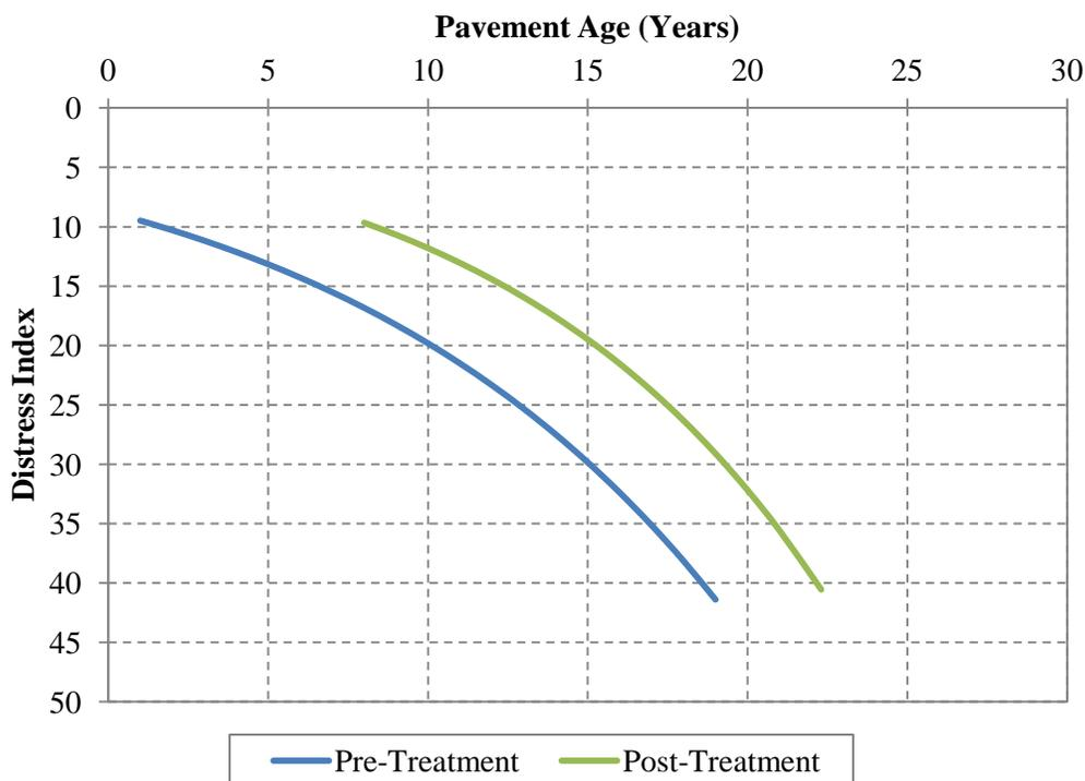
Figure 4.40. Pre- and post-treatment pavement performance – HMA overlay on flexible pavement (all zones).
