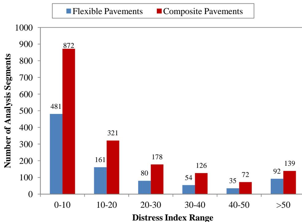
Figure 5.1. Distribution of pre-treatment pavement conditions (DI) for first CPM treatments.
