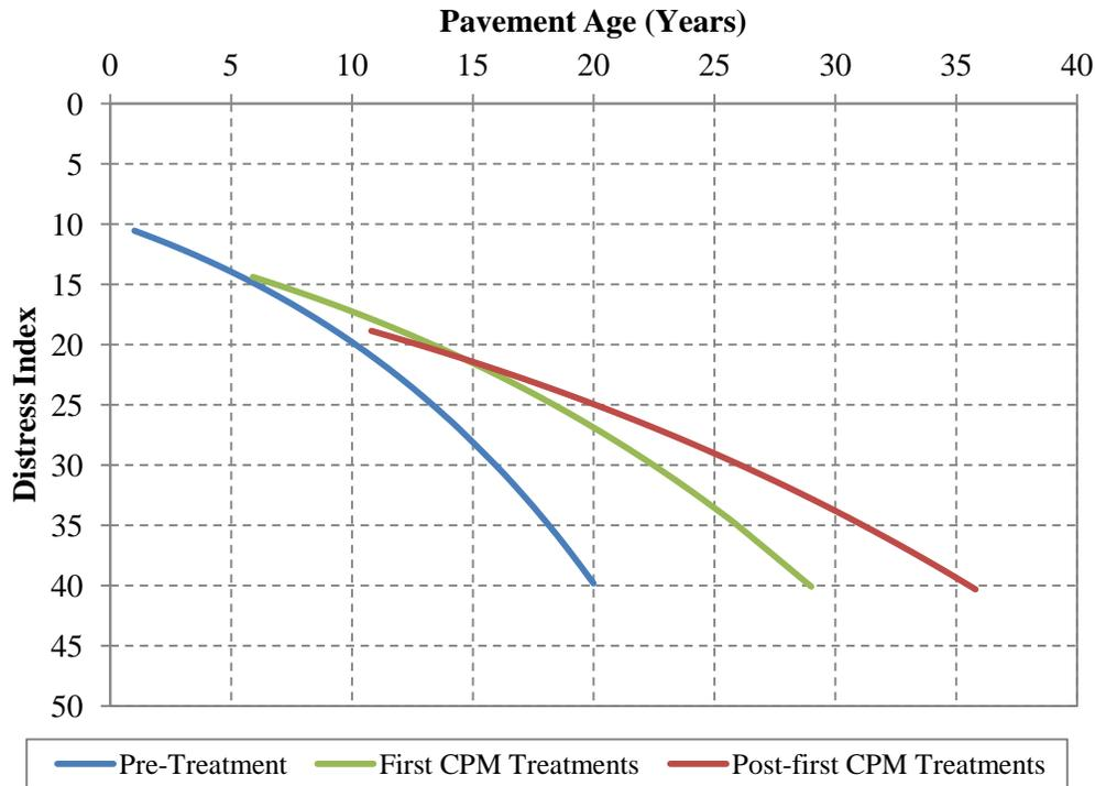
Figure 5.11. Pre- and post-treatment pavement on composite pavement (all zones).
