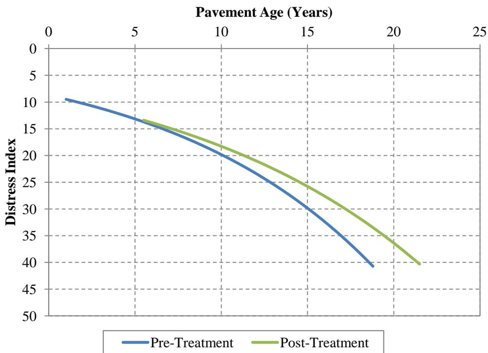
Figure 4.23. Pre- and post-treatment pavement performance – HMA crack treatment on flexible pavement (all zones).
