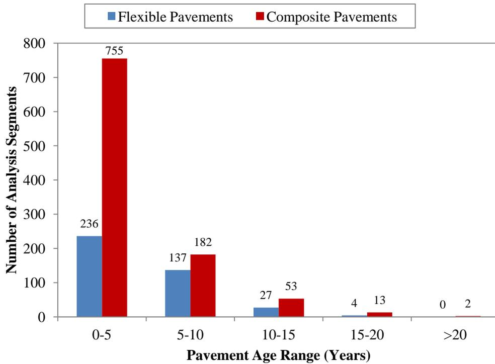
Figure 4.22. Pre-treatment pavement age distribution for HMA crack treatments.
