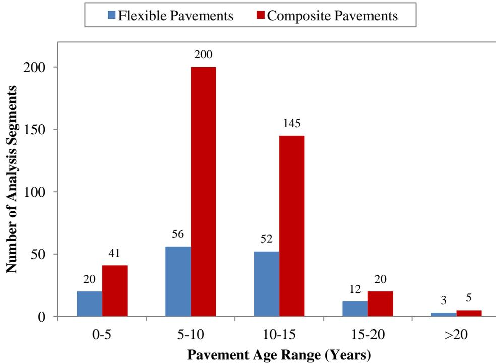
Figure 4.32. Pre-treatment pavement age distribution for HMA mill and overlay treatments.
