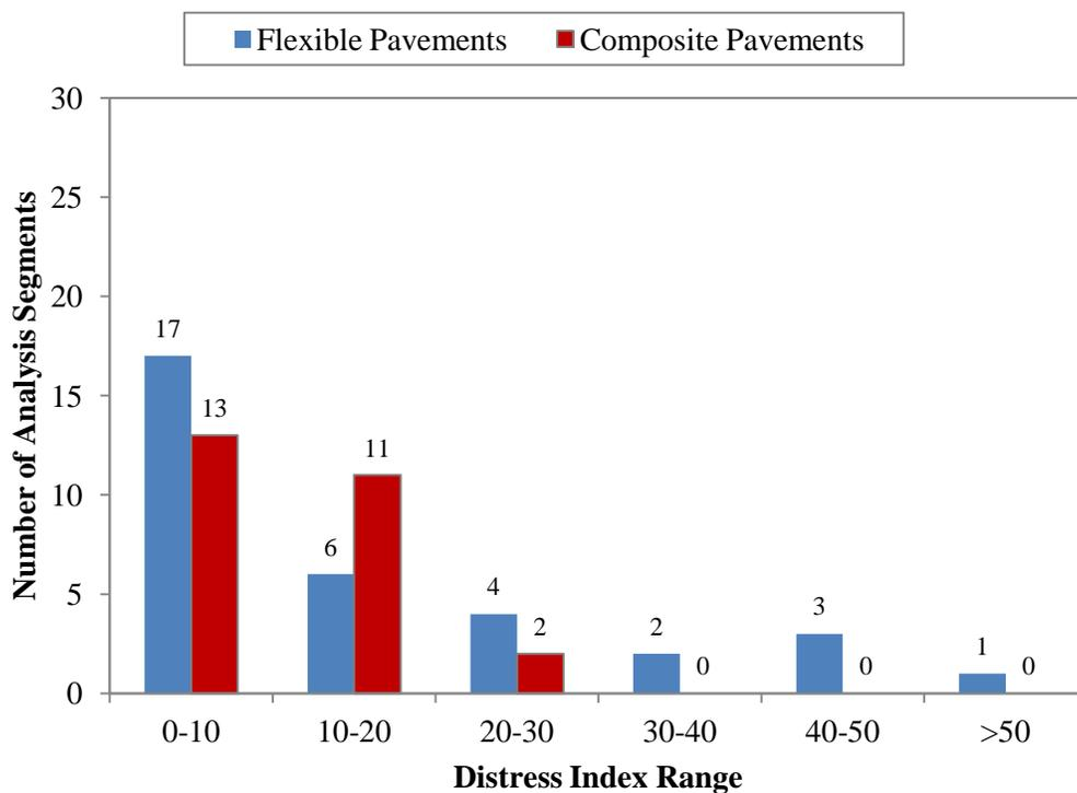
Figure 4.29. Pre-treatment pavement condition distribution for ultra-thin HMA OL.
