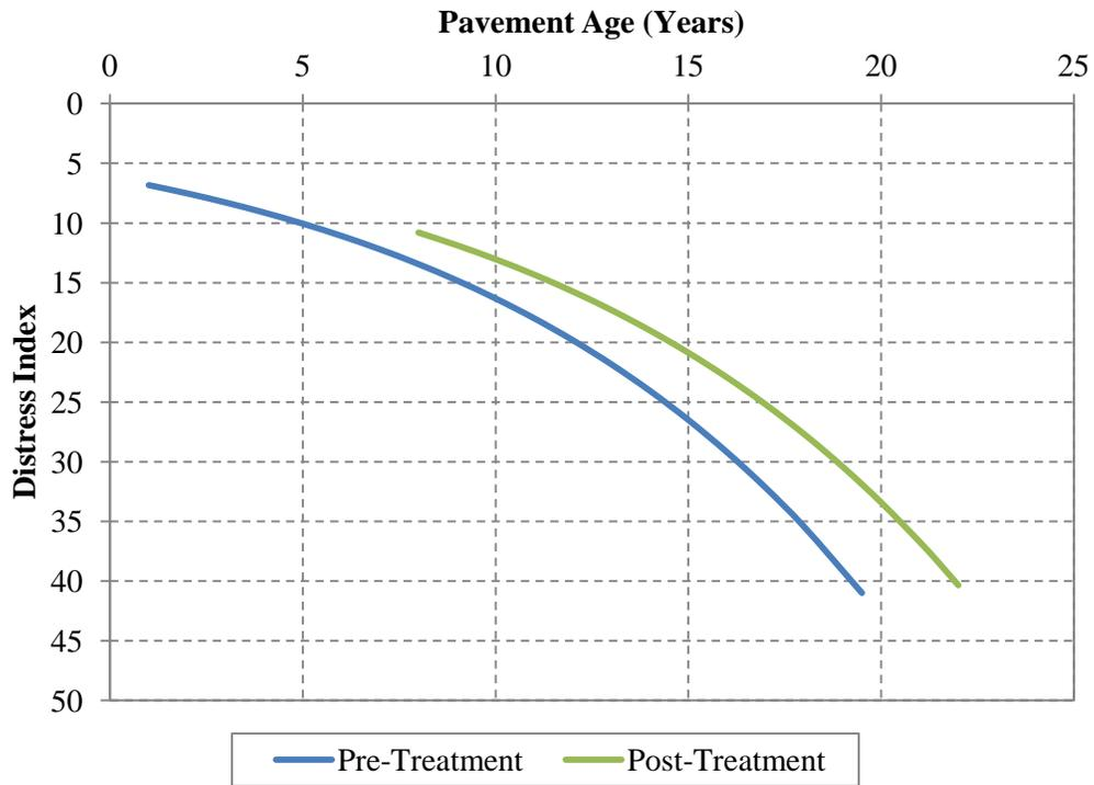
Figure 4.6. Pre- and post-treatment pavement performance – single chip seal on flexible pavement (Zone 1).
