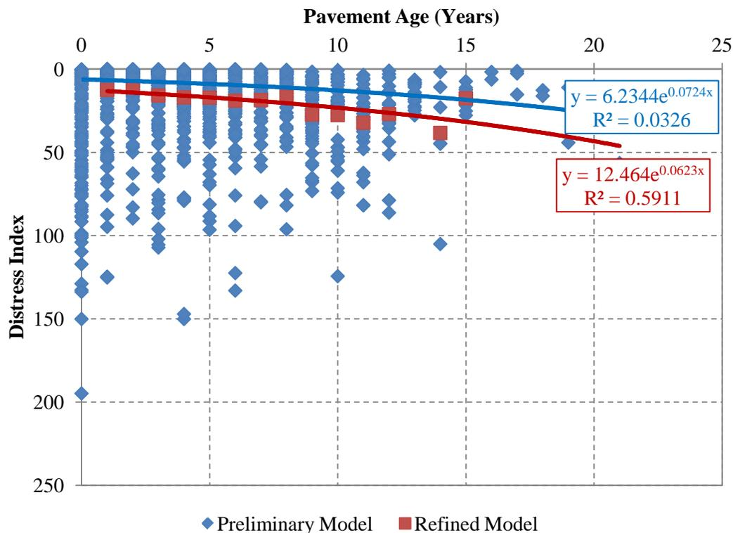
Figure 4.2. Sample comparison between preliminary and refined performance models.
