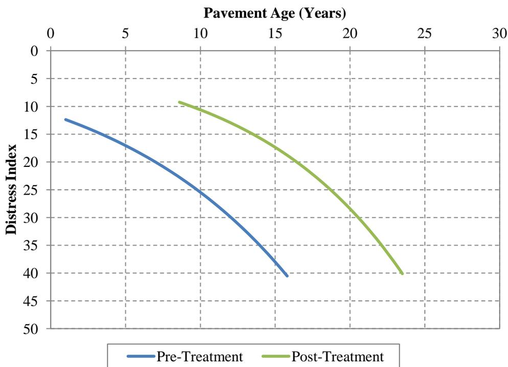
Figure 4.34. Pre- and post-treatment pavement performance – HMA mill and overlay on flexible pavement (Zone 2).
