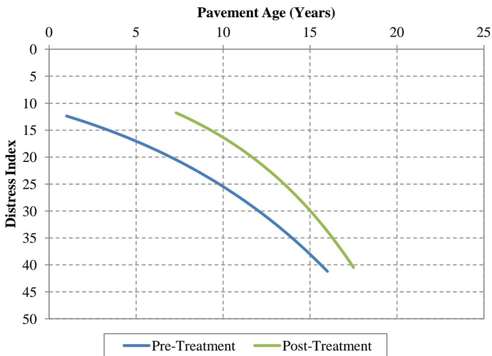
Figure 4.16. Pre- and post-treatment pavement performance – double microsurfacing on flexible pavement (Zone 2).
