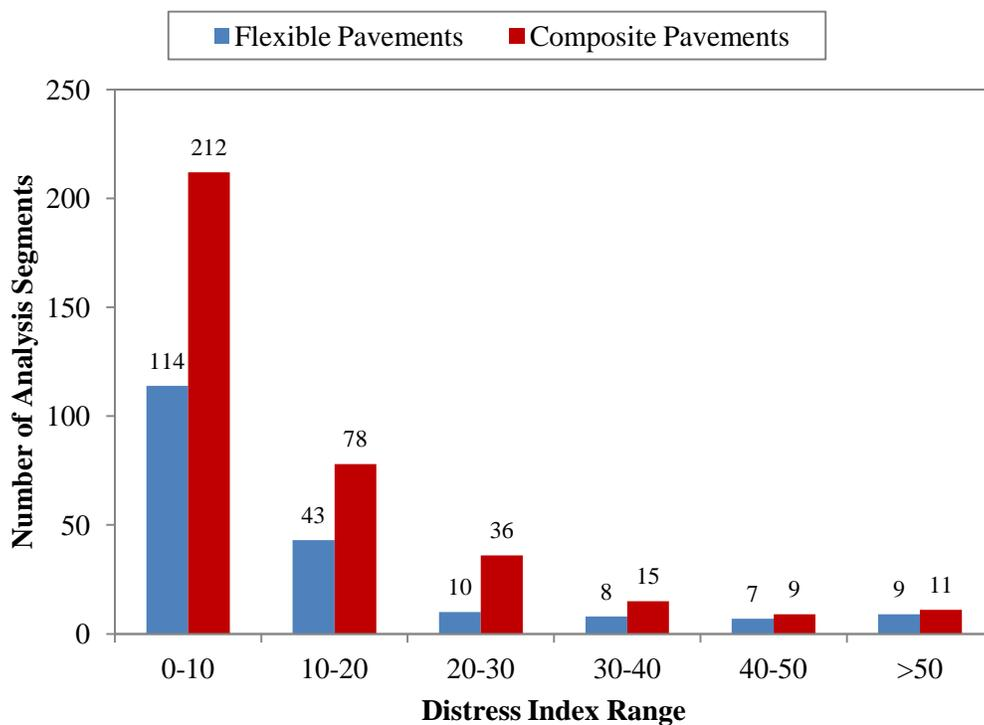
Figure 4.12. Pre-treatment pavement condition distribution for double microsurfacing treatments.
