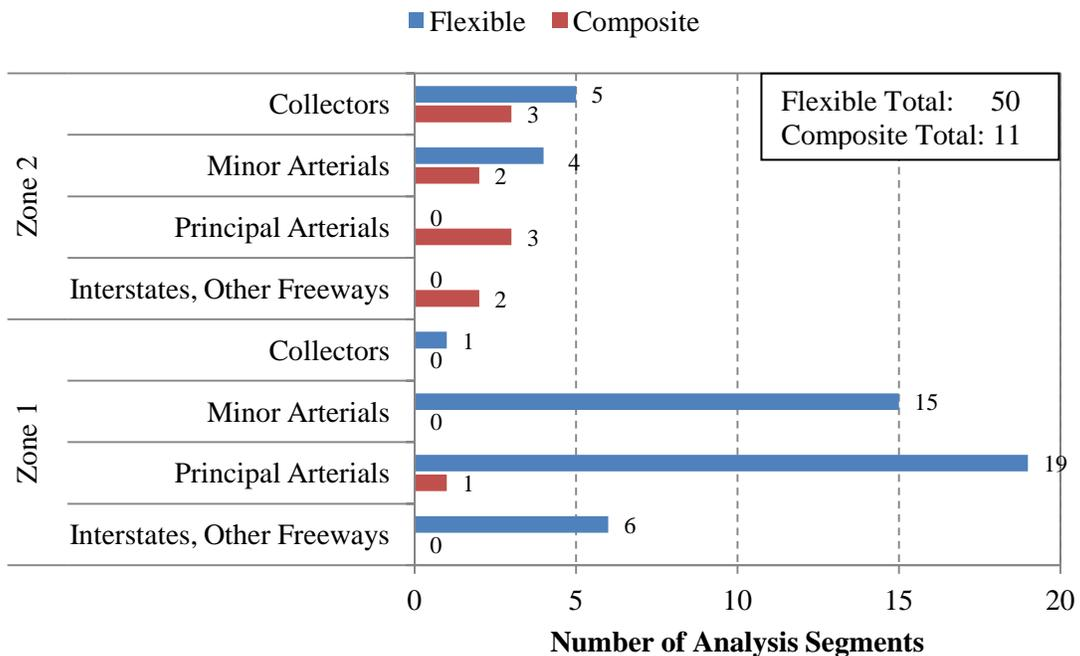
Figure 3.14. Number of ultra-thin HMA OL segments used in the analysis (post-first treatment).
