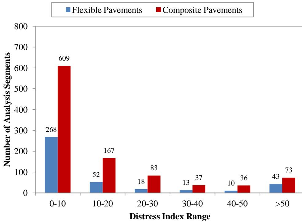
Figure 4.21. Pre-treatment pavement condition distribution for HMA crack treatments.
