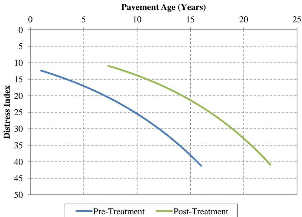
Figure 4.7. Pre- and post-treatment pavement performance – single chip seal on flexible pavement (Zone 2).
