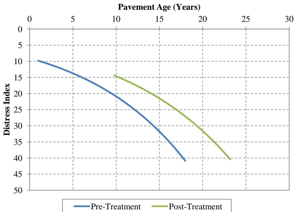
Figure 4.37. Pre- and post-treatment pavement performance – HMA mill and overlay on composite pavement (Zone 2).
