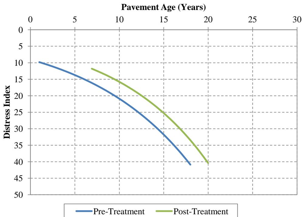
Figure 4.43. Pre- and post-treatment pavement performance – HMA overlay on composite pavement (Zone 2).
