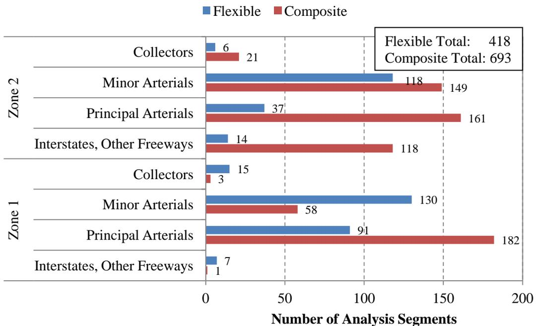
Figure 3.12. Number of HMA crack seal segments used in the analysis (post-first treatment).
