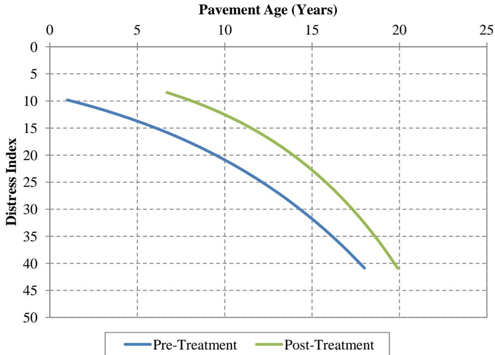
Figure 4.11. Pre- and post-treatment pavement performance – double chip seal on composite pavements (Zone 2).
