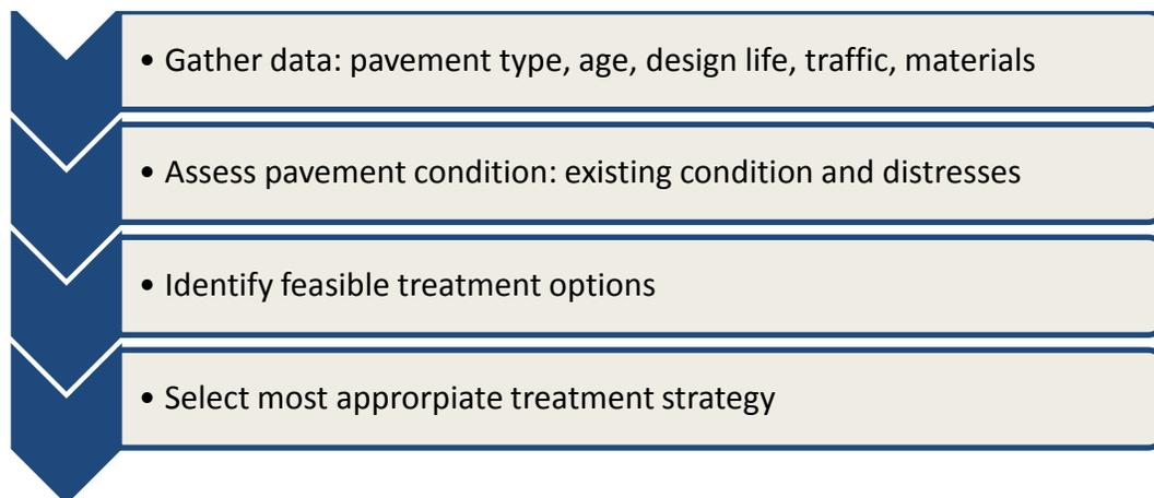
Figure 6.1. Flowchart illustrating steps in selecting an appropriate preventive maintenance treatment.
