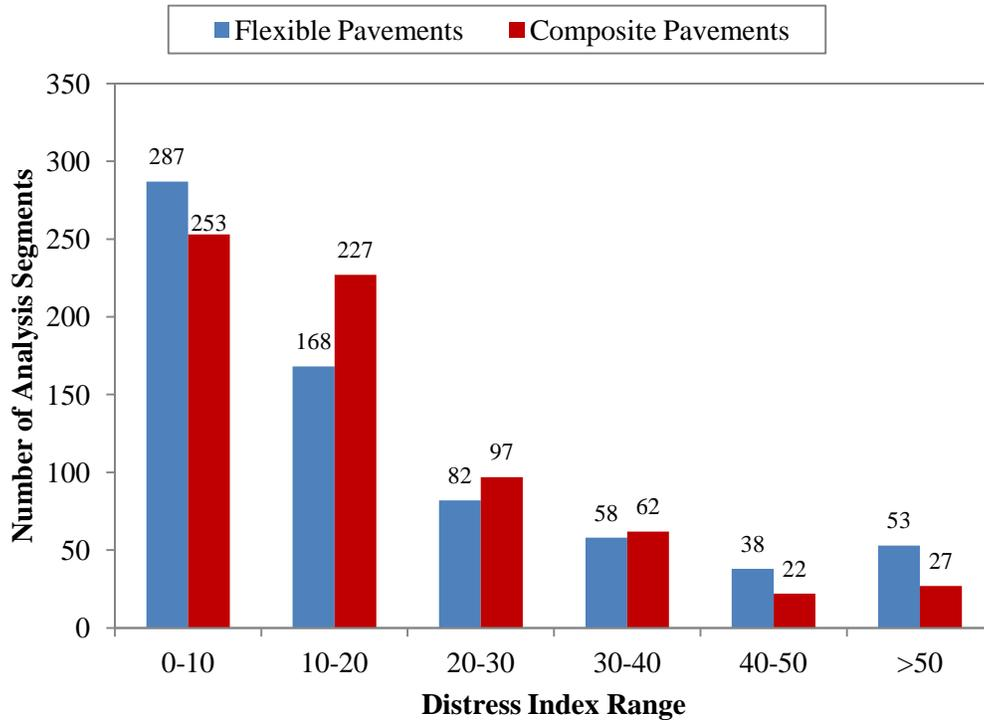
Figure 5.8. Pre-treatment pavement condition distribution for post-first CPM treatments.
