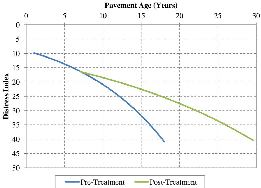
Figure 4.18. Pre- and post-treatment pavement performance – double microsurfacing on composite pavement (Zone 2).
