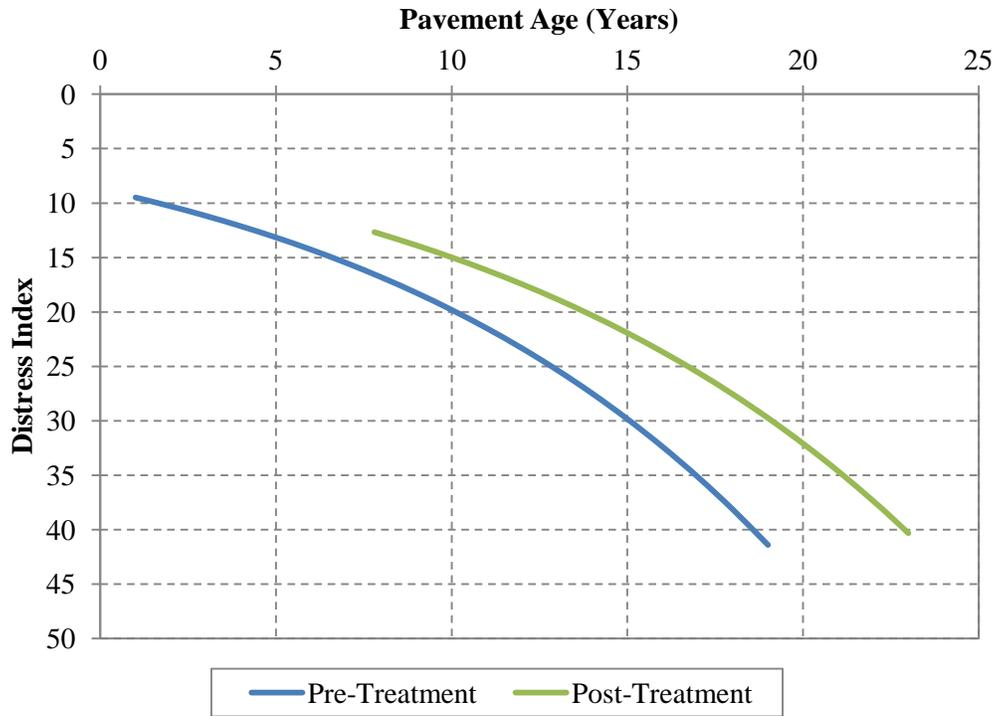
Figure 4.5. Pre- and post-treatment pavement performance – single chip seal on flexible pavement (all zones).
