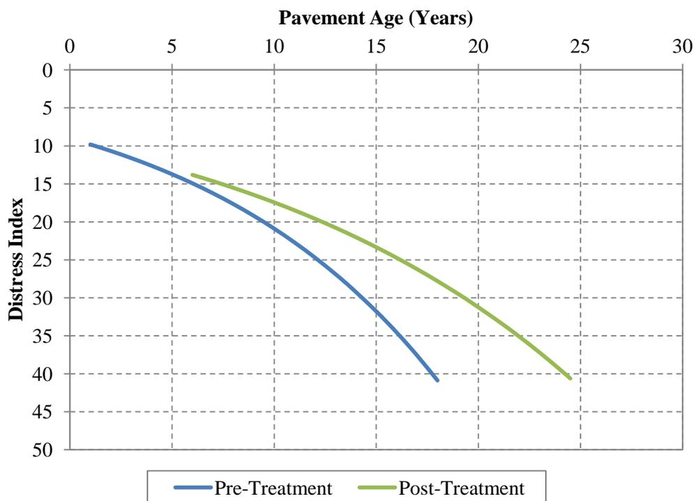
Figure 5.7. Pre- and post-treatment pavement performance – first CPM treatments on composite pavements (Zone 2).
