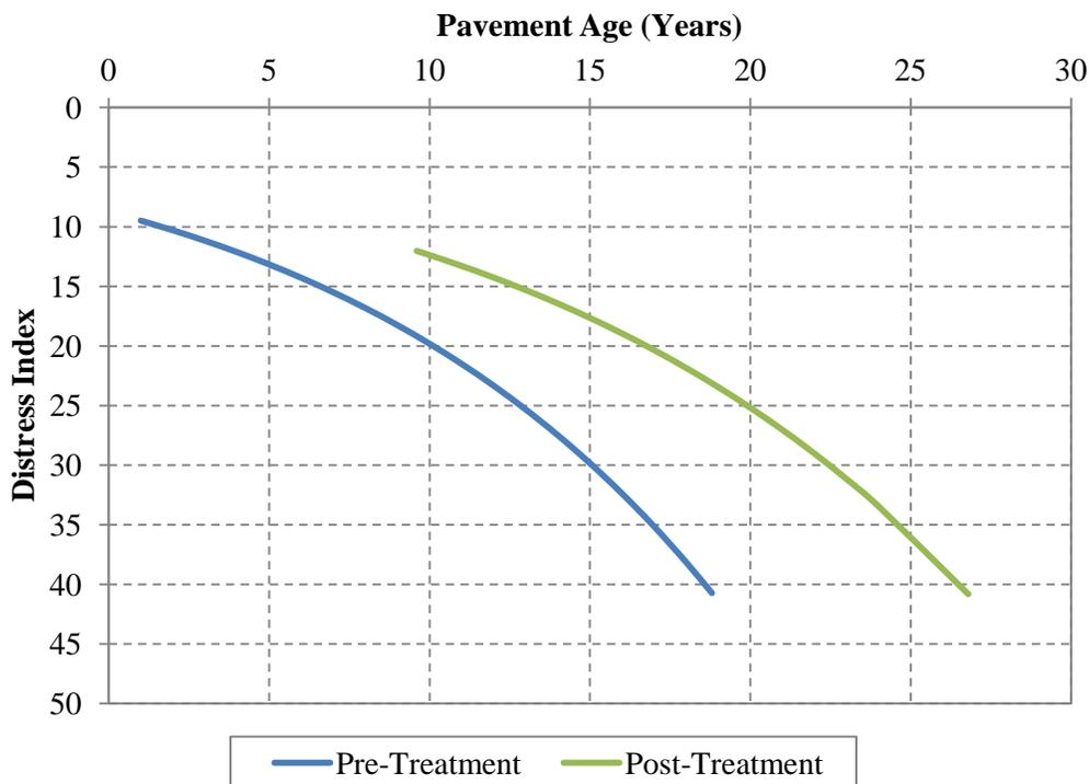
Figure 4.33. Pre- and post-treatment pavement performance – HMA mill and overlay on flexible pavement (all zones).
