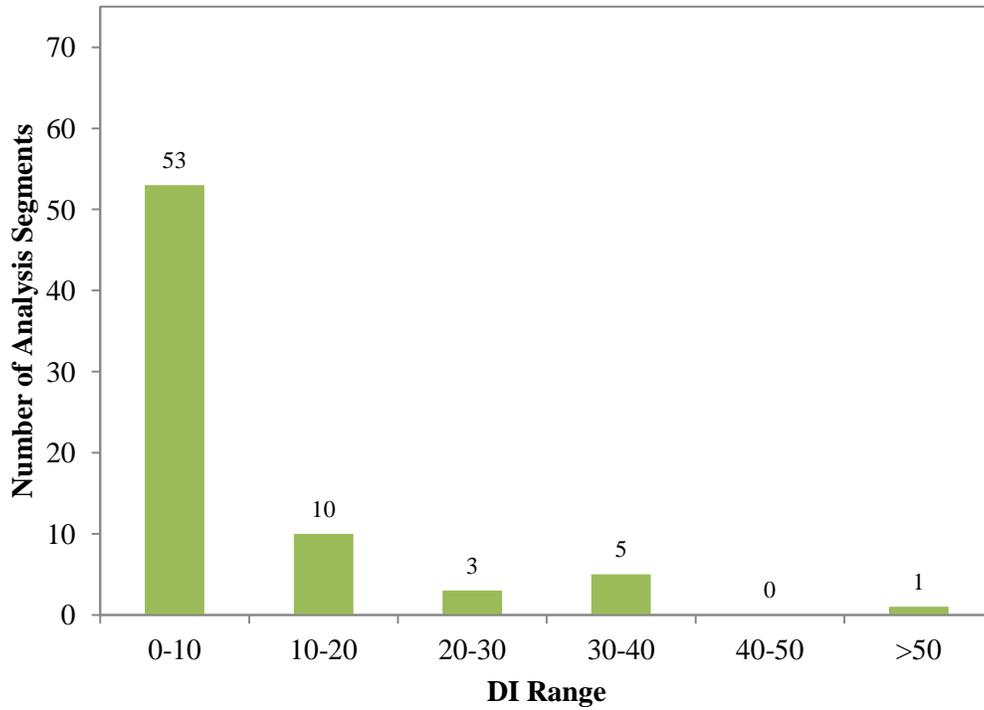
Figure 4.44. Pre-treatment pavement condition distribution for PCC joint and crack seals.
