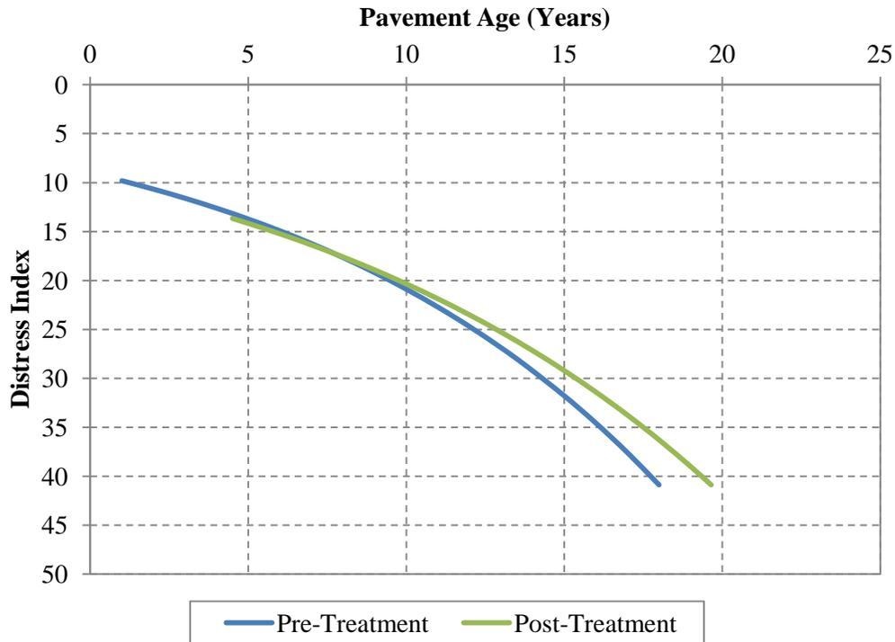
Figure 4.28. Pre- and post-treatment pavement performance – HMA crack treatment on composite pavement (Zone 2).
