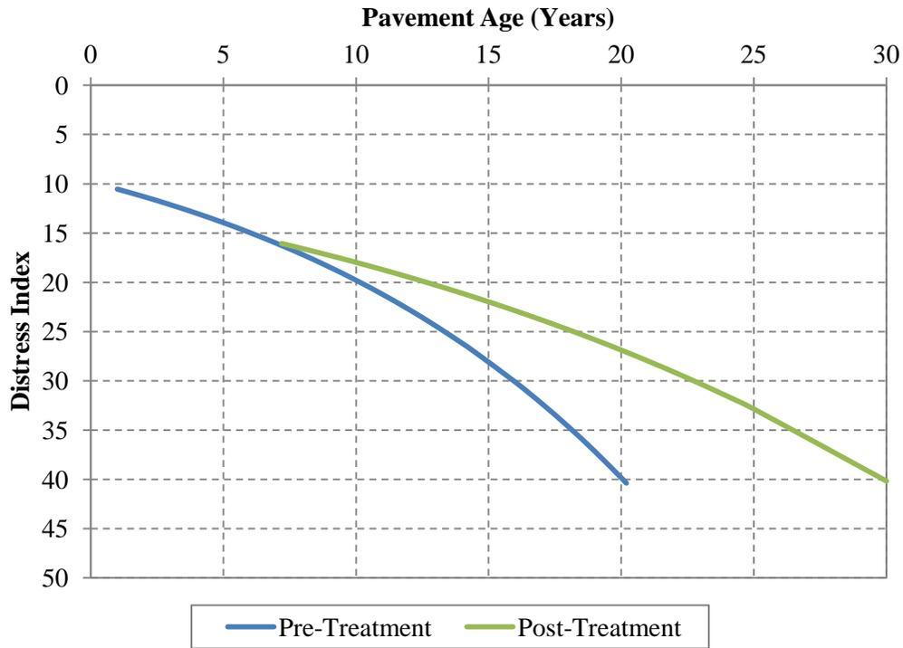
Figure 4.17. Pre- and post-treatment pavement performance – double microsurfacing on composite pavement (all zones).
