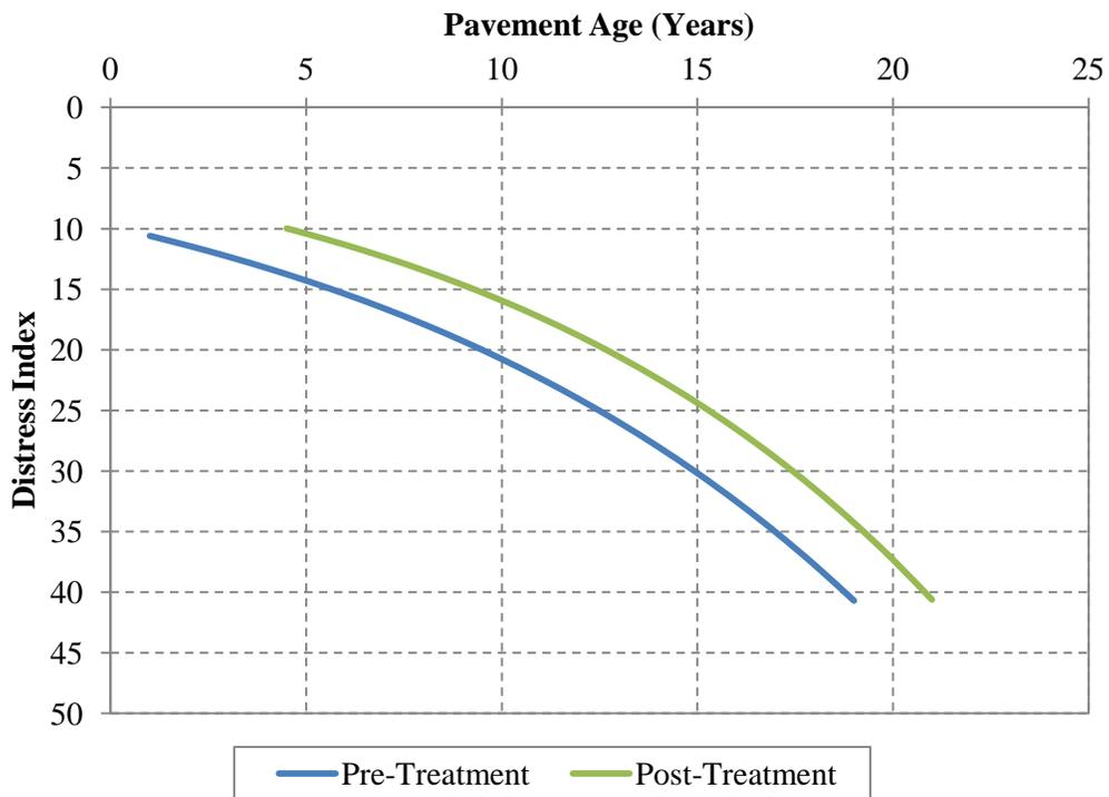
Figure 4.27. Pre- and post-treatment pavement performance – HMA crack treatment on composite pavement (Zone 1).
