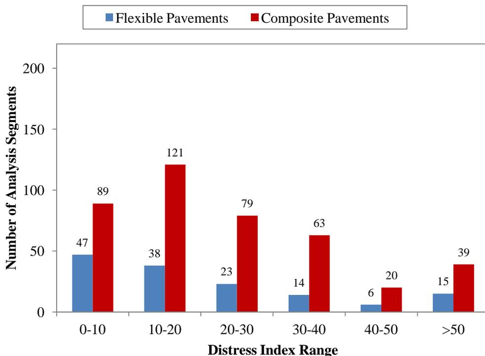
Figure 4.31. Pre-treatment pavement condition distribution for HMA mill and overlay treatments.
