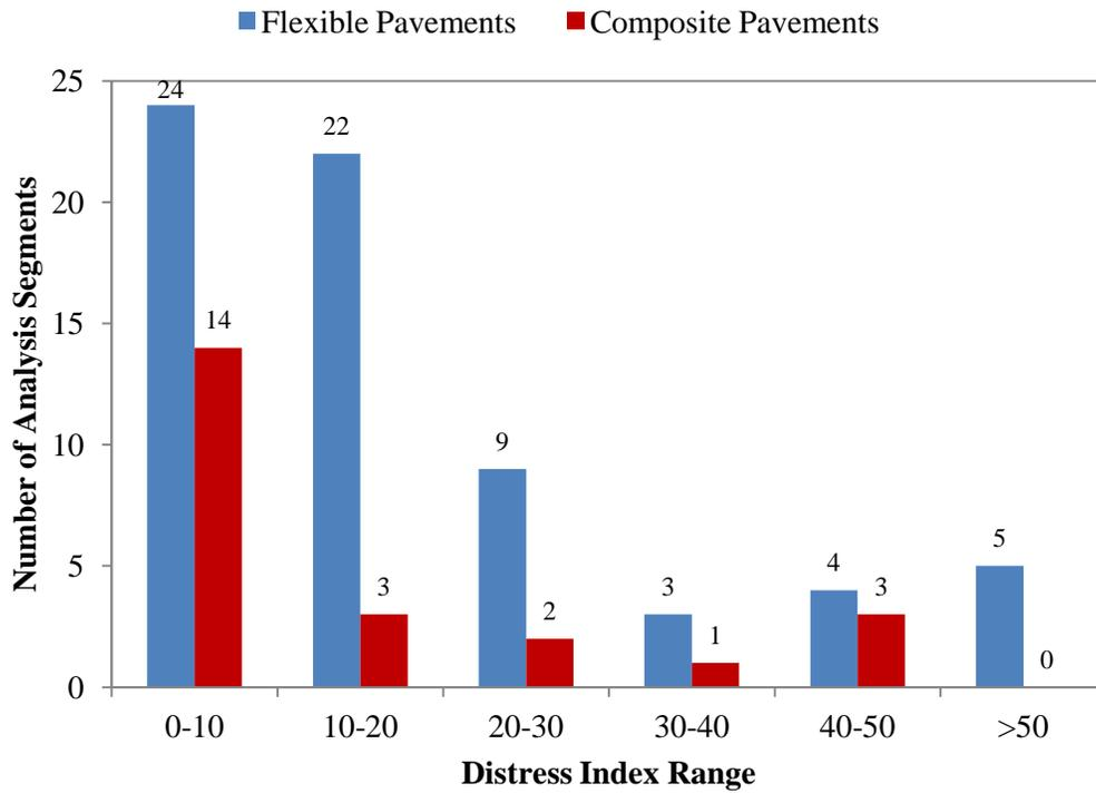
Figure 4.8. Pre-treatment pavement condition distribution for double chip seals.
