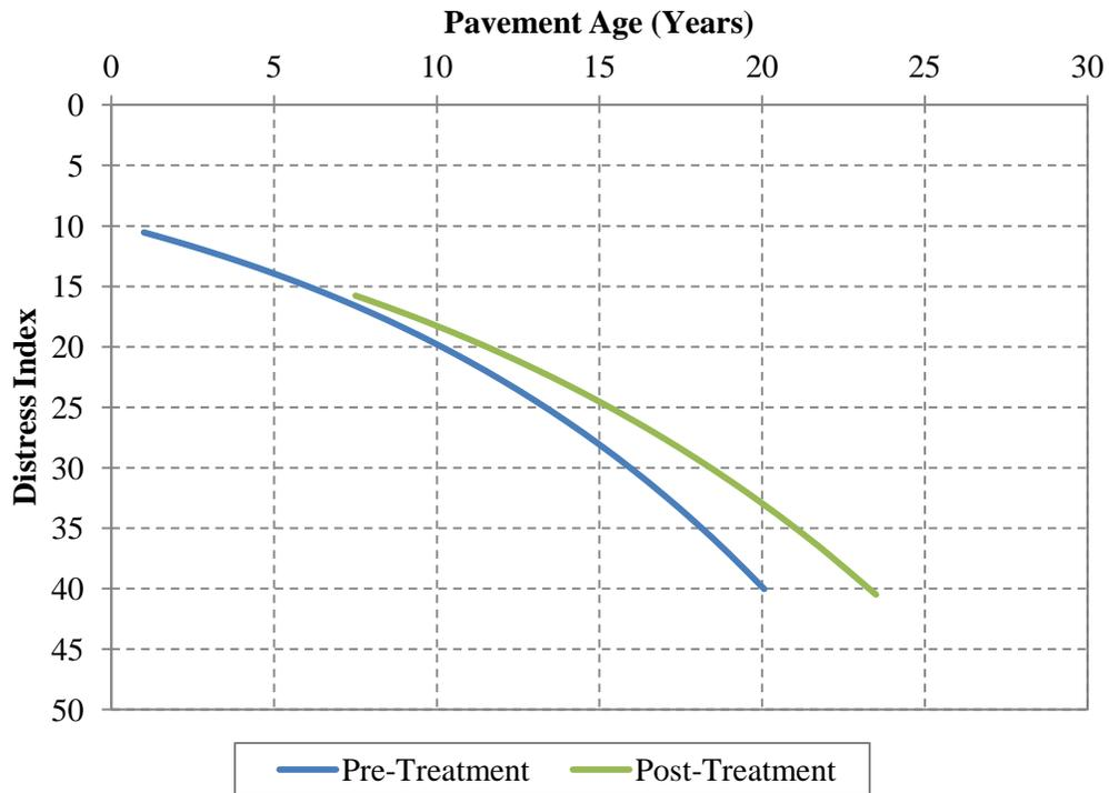
Figure 4.42. Pre- and post-treatment pavement performance – HMA overlay on composite pavement (all zones).
