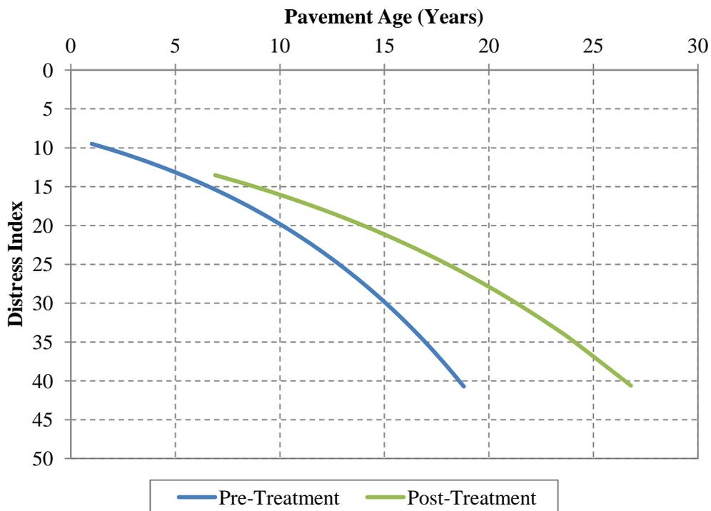
Figure 5.3. Pre- and post-treatment pavement performance – first CPM treatments on flexible pavements (all zones).
