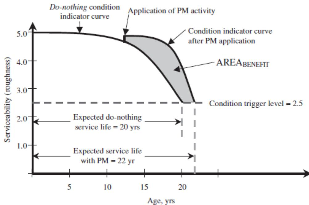
Figure 2.1. Illustration of benefit associated with a preventive maintenance treatment (Peshkin et al. 2004).
