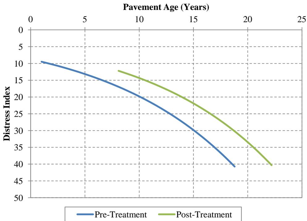
Figure 4.14. Pre- and post-treatment pavement performance – double microsurfacing on flexible pavement (all zones).
