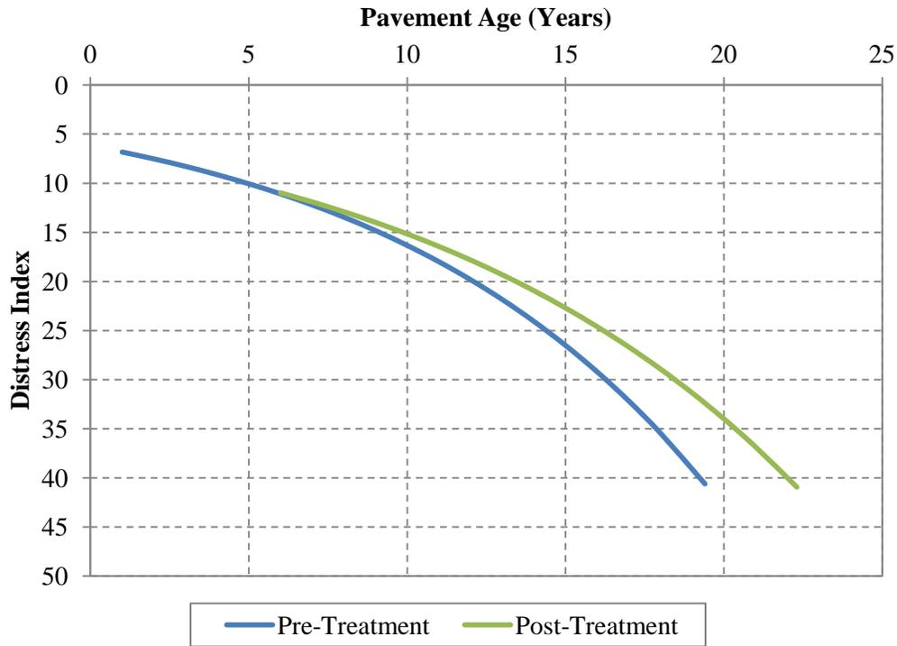
Figure 4.24. Pre- and post-treatment pavement performance – HMA crack treatment on flexible pavement (Zone 1).
