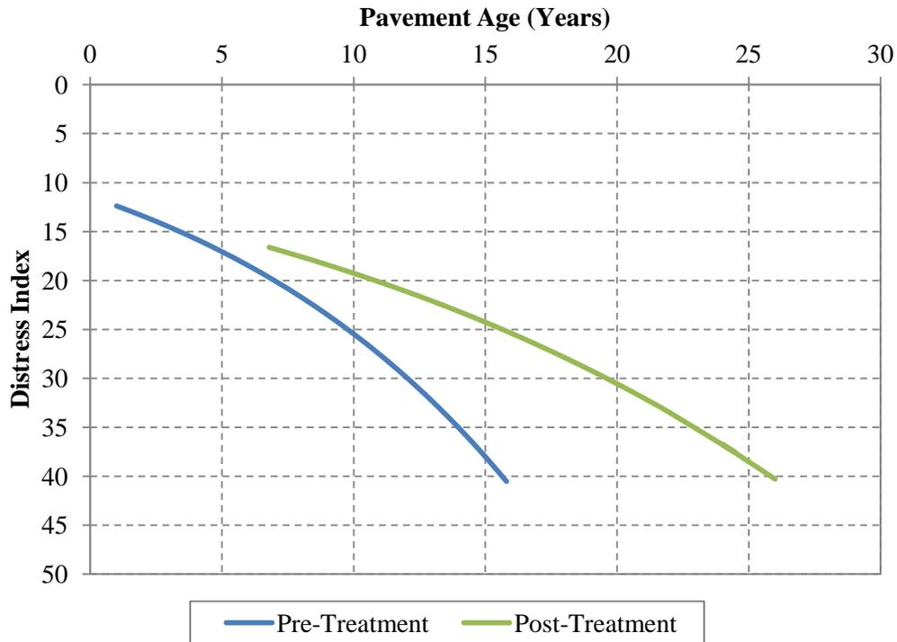
Figure 5.5. Pre- and post-treatment pavement performance – first CPM treatments on flexible pavements (Zone 2).
