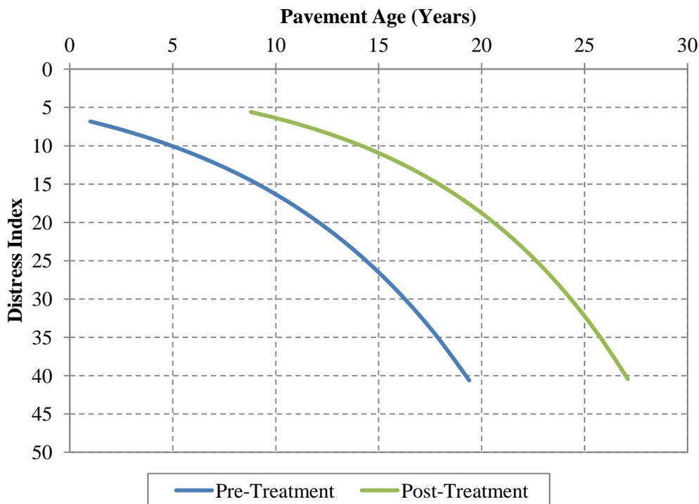
Figure 4.15. Pre- and post-treatment pavement performance – double microsurfacing on flexible pavement (Zone 1).
