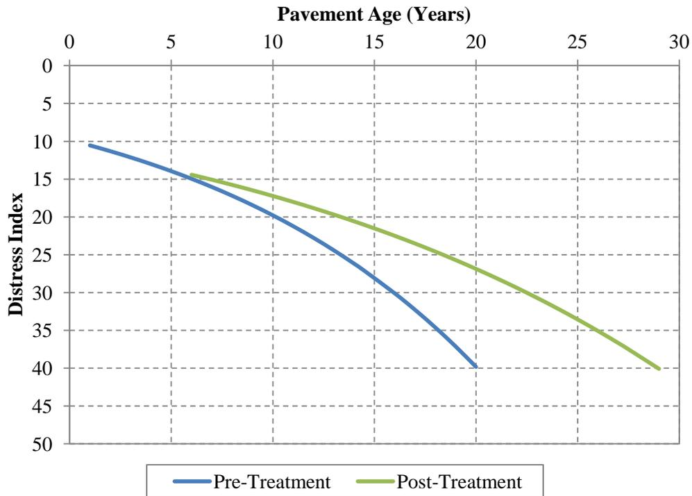
Figure 5.6. Pre- and post-treatment pavement performance – first CPM treatments on composite pavements (all zones).
