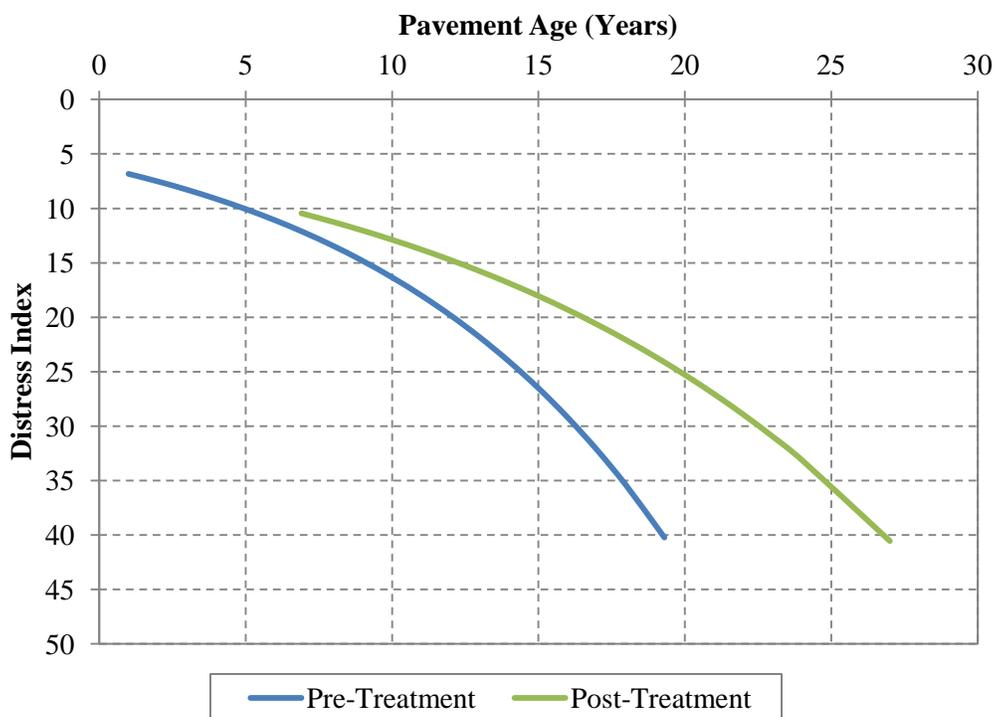
Figure 5.4. Pre- and post-treatment pavement performance – first CPM treatments on flexible pavements (Zone 1).
