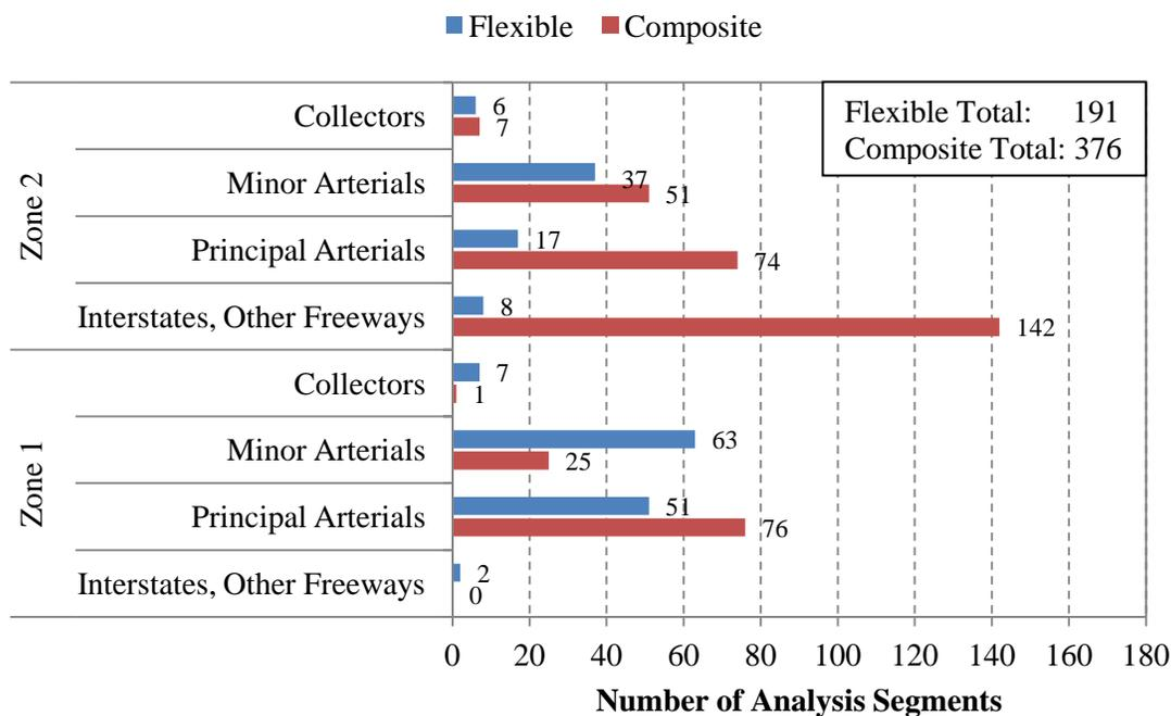
Figure 3.16. Number of HMA Mill OL segments used in the analysis (post-first treatment).
