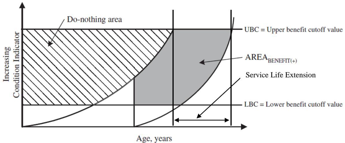
Figure 4.1. Illustration of pavement service life extension and benefit area (Peshkin et al. 2004).
