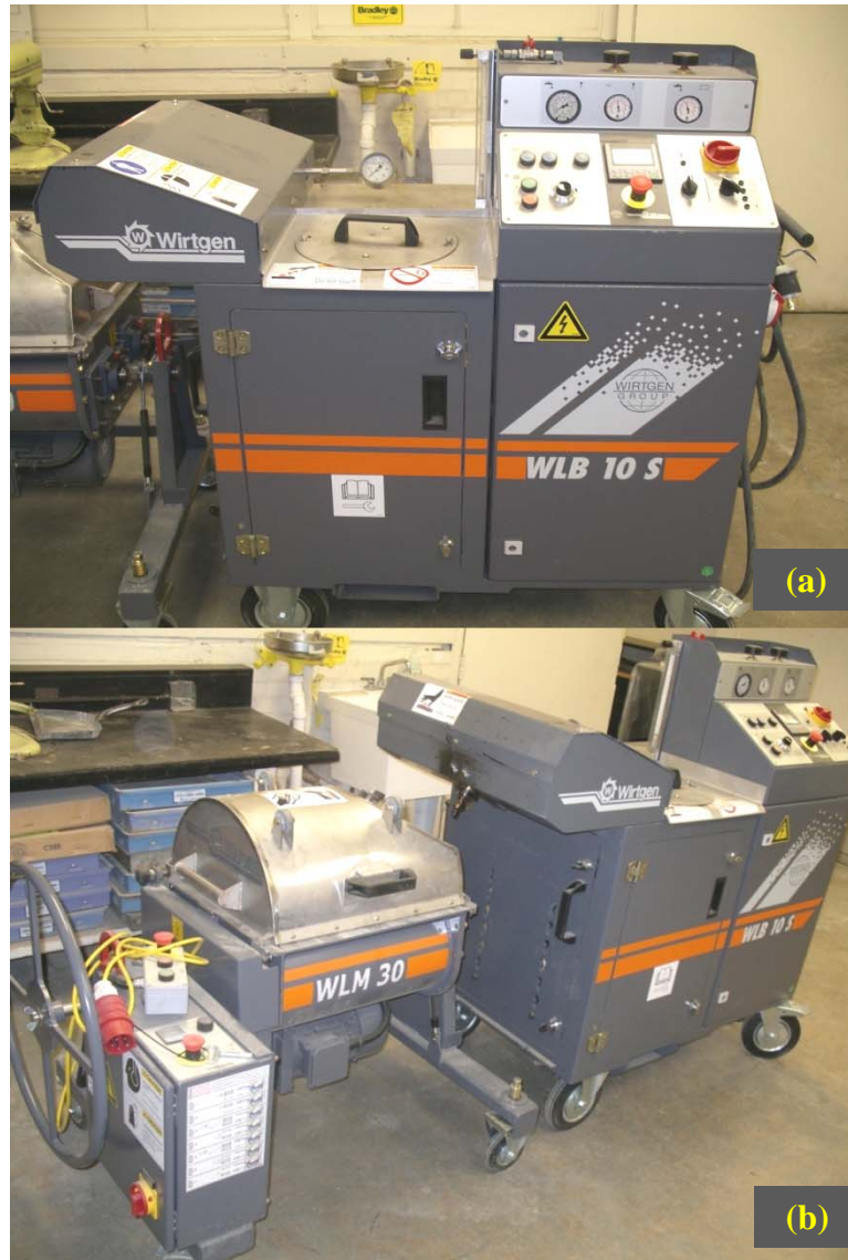
Figure 4.a) Wirtgen WLB 10S laboratory-scale foamed asphalt plant, b) WLM 30 laboratory-scale pugmill mixer.
