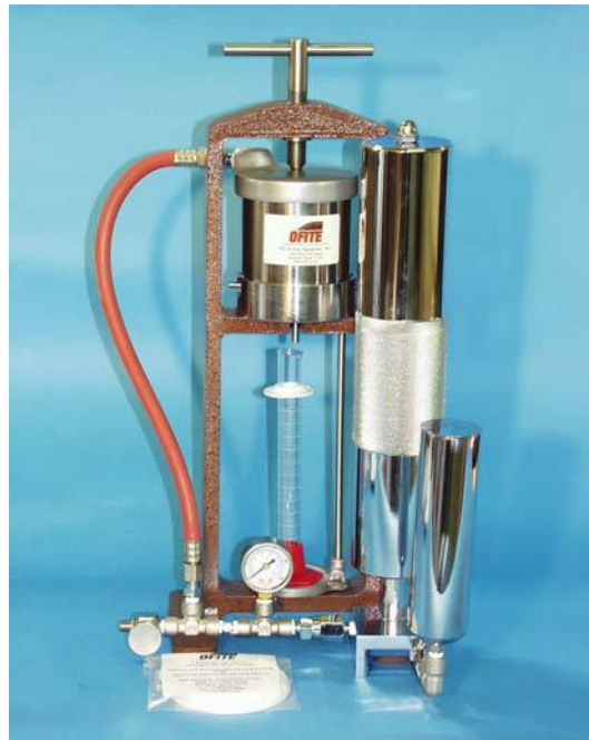
Figure 3.1 Components of the API filter press with dead-weight system (Ofite, 2011).
