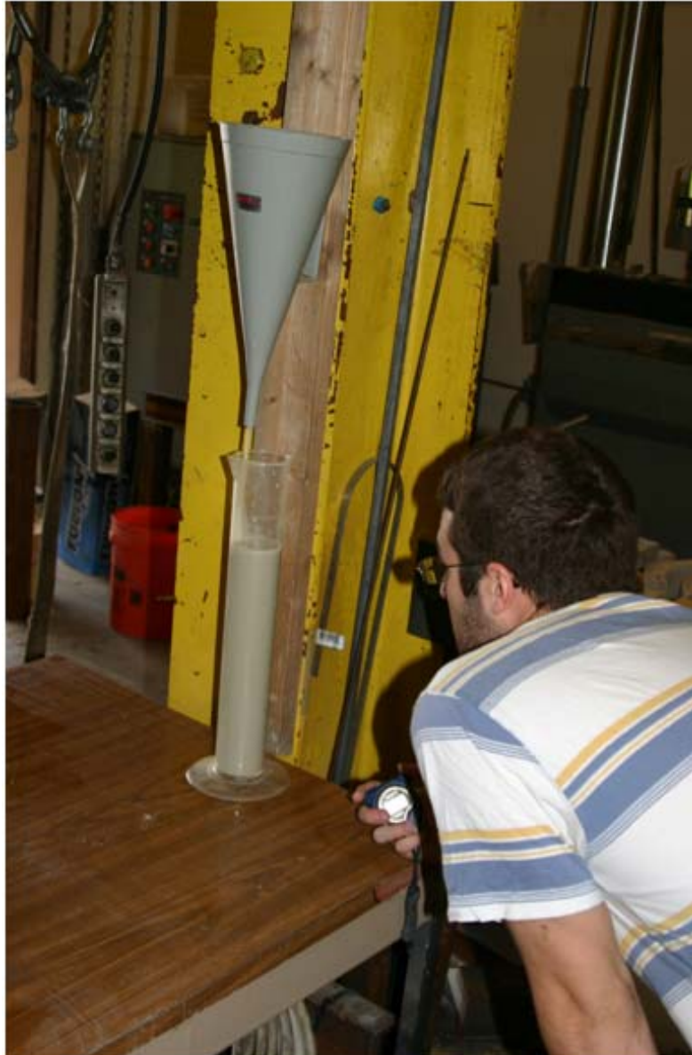
Figure 3.5 Viscosity measurements using a 1000 ml beaker marked precisely at the one quart volume.
