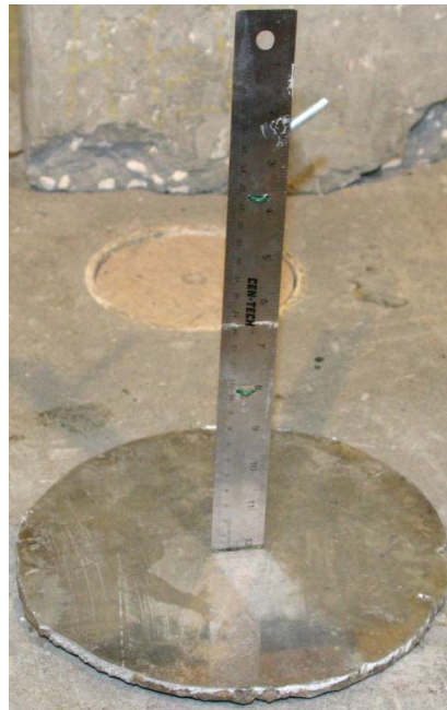
Figure 4.43 Bucket sampler false bottom with accumulation ruler.
