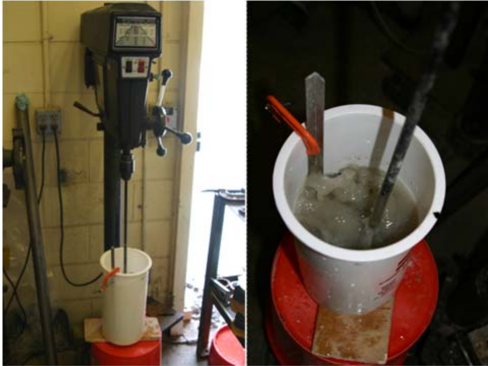
Figure 3.3 Slurry Mixing Setup
