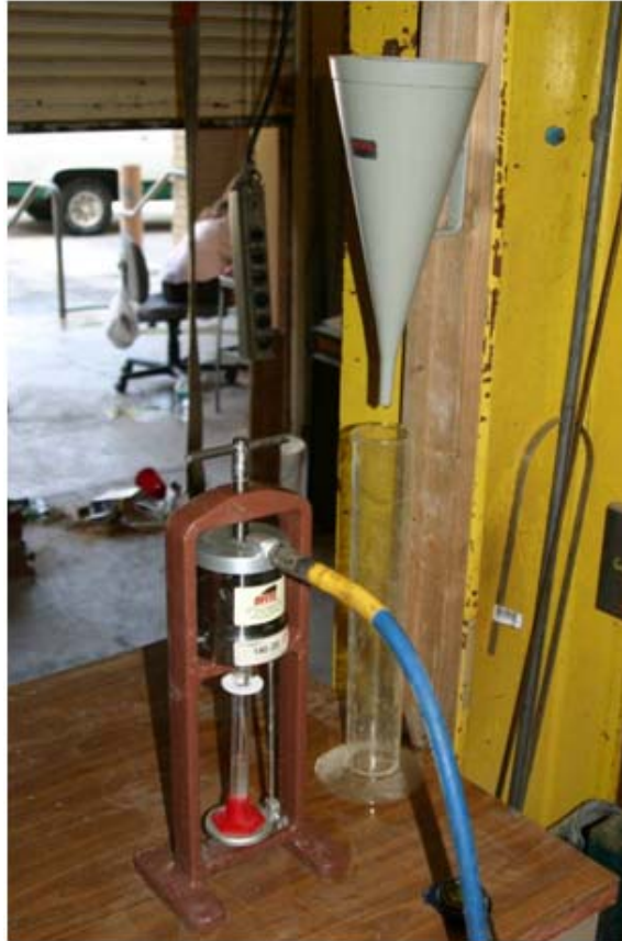
Figure 3.2 API filter press test in progress using a constant air pressure source.
