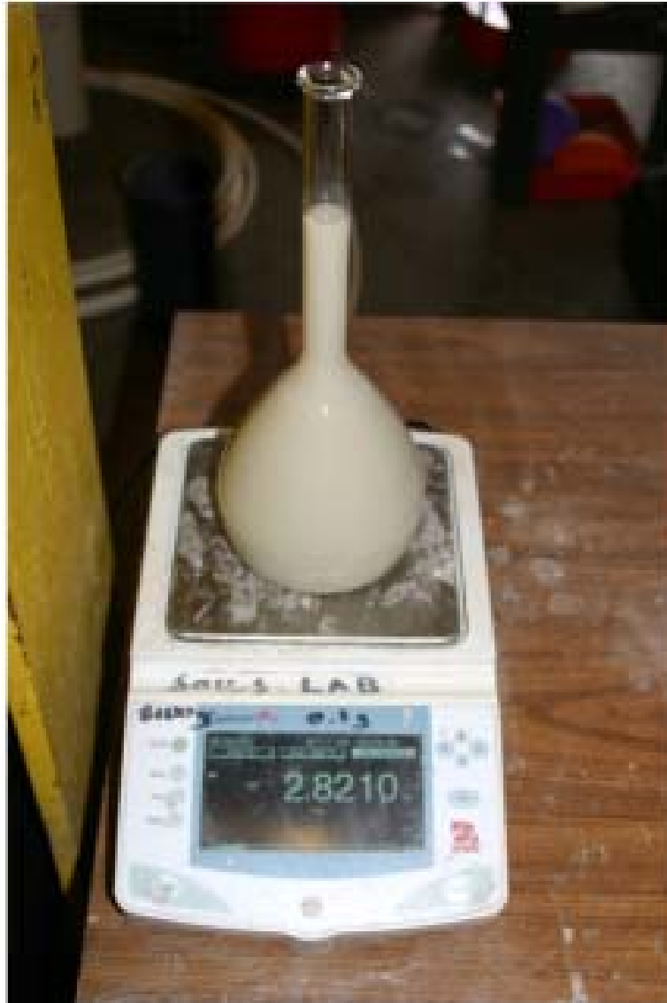
Figure 3.6 Density measurements with a digital scale and a volumetric flask.
