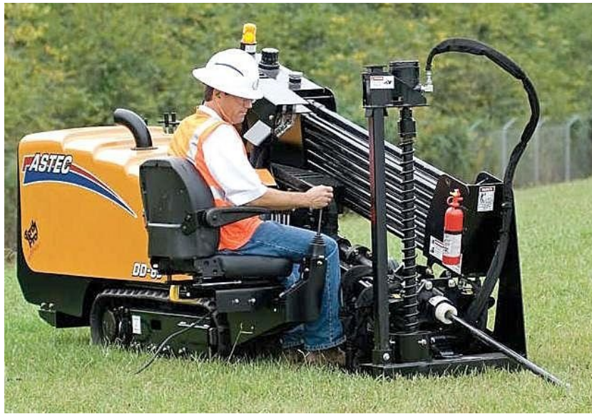
Figure 2.5 Horizontal directional drilling rig (Astec Industries, 2011).
