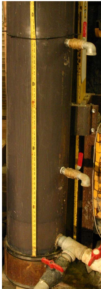
Figure 4.14 Sand content ports on transparent PVC column.
