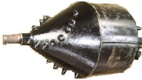
Figure 2.6 Horizontal directional drilling back reaming device (Wuxi Drilling Tools Factory, 2011).
