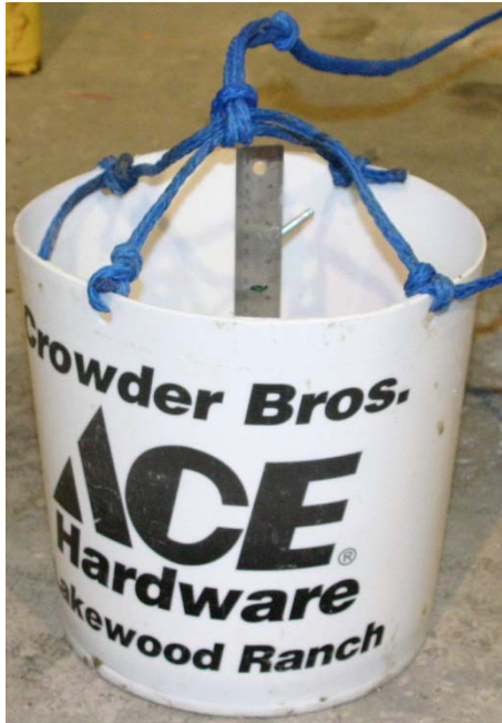
Figure 4.44 Bucket sampler with removable false bottom.
