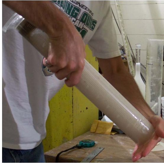
Figure 4.49 Agitation of sand and slurry solution.
