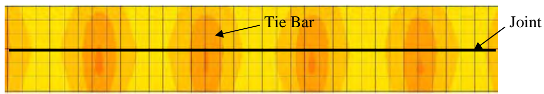
Figure 30. Scan of a typical Category I joint at the I-70 mile post 308.2 site.
