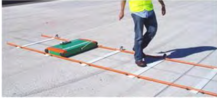
Figure 13. Pulling the MIT Scan device along the rail system.
