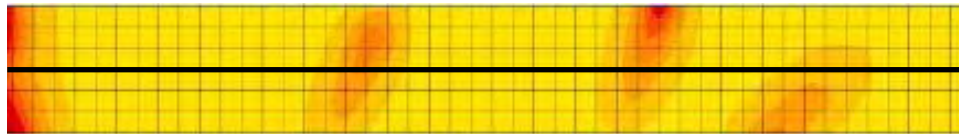
Figure 33. Scan of a typical Category II joint at the I-70 mile post 316 site.
