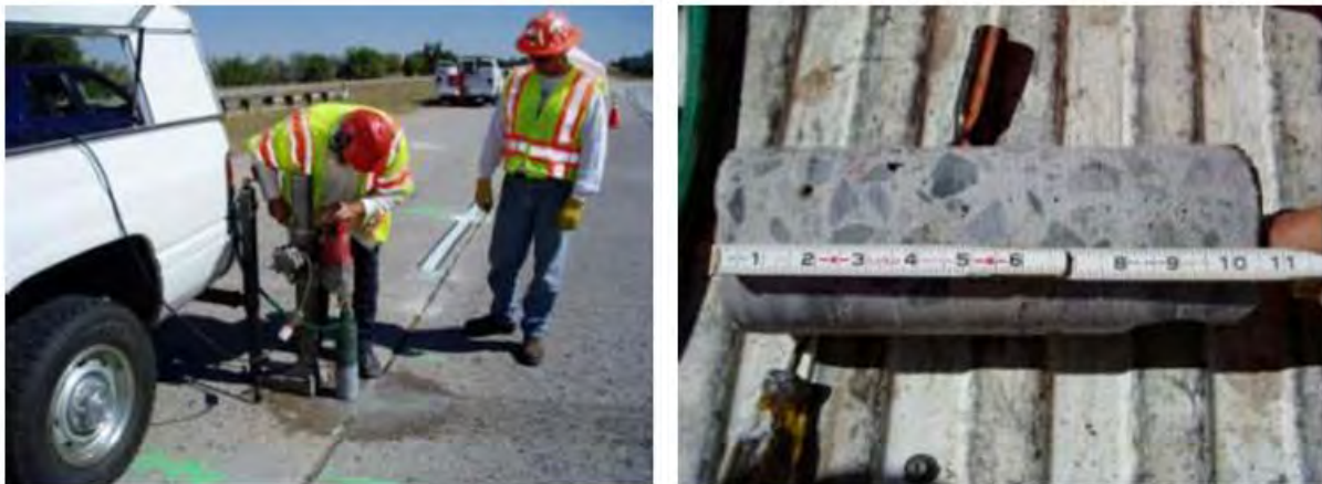
Figure 24. Cutting core sample (left) and the 10.5-in. core (right) from Test Joint A.
