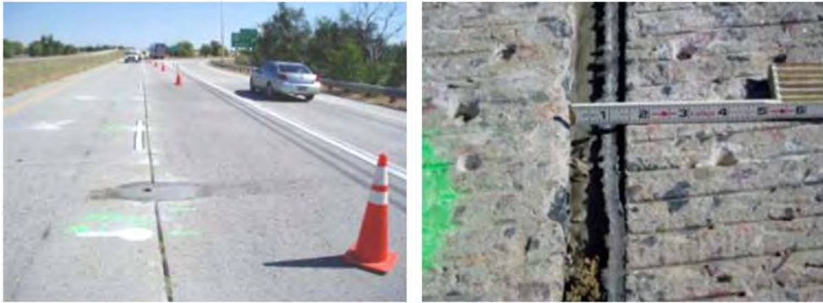
Figure 23. Test Joints A, B, and C (left) and close-up of Test Joint A (right).
