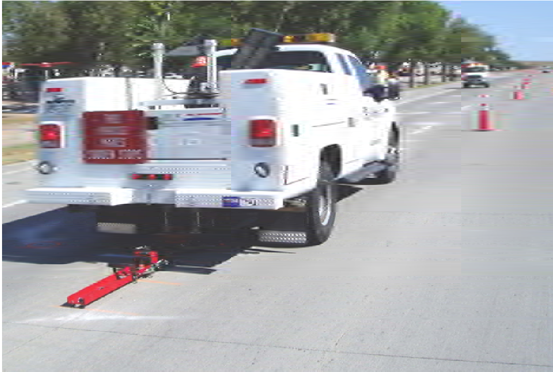
Figure 11. FWD configured for longitudinal joint LTE testing.
