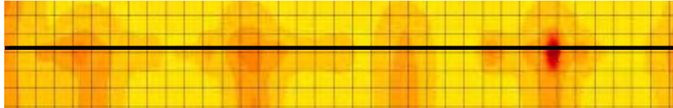
Figure 41. Scan of a typical poorly performing joint at the I-225 mile post 10.5 site.
