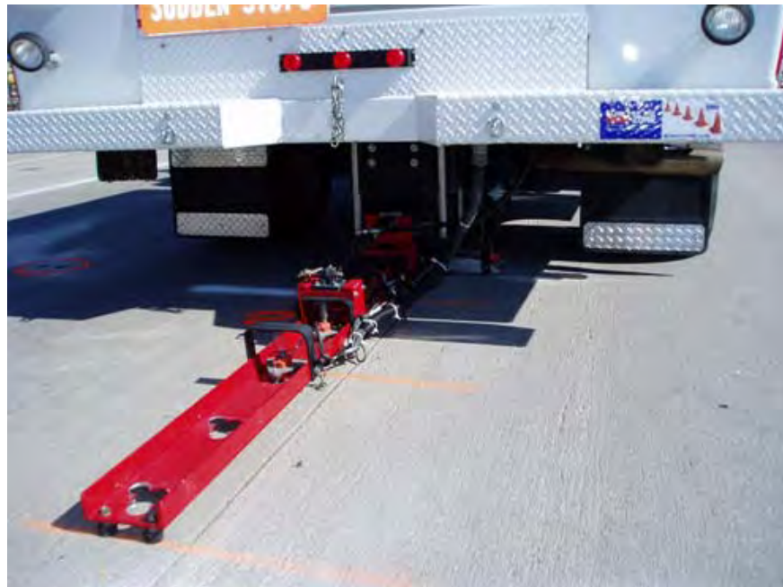
Figure 12. Close-up of FWD load plate and side sensor.
