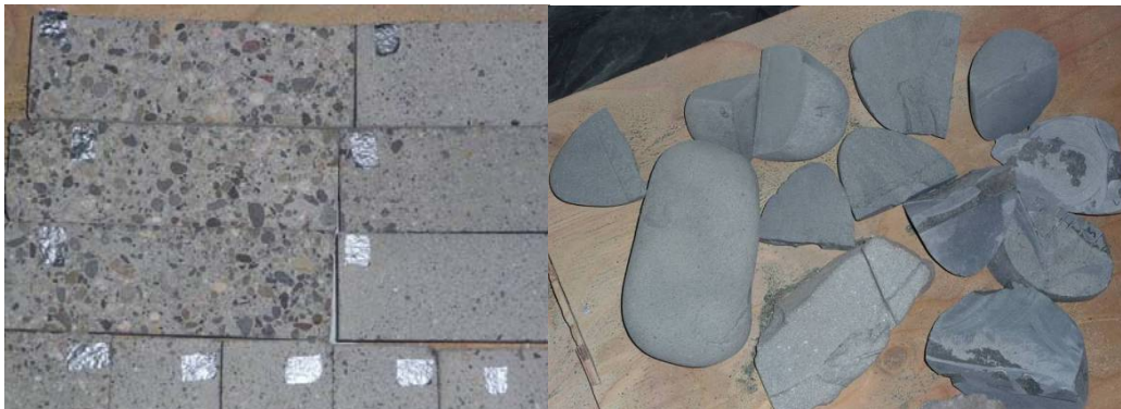
Figure 4.11: PCC samples (left) and rock samples (right) after profiling and before arc-spraying.
