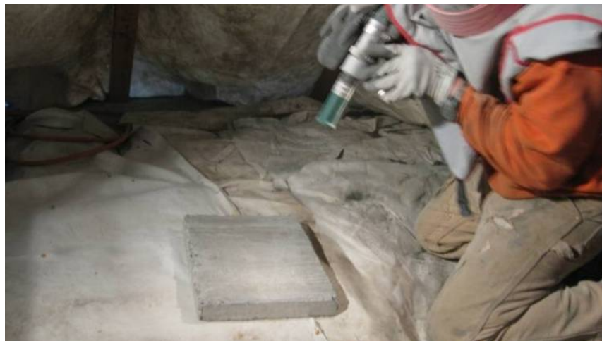
Figure 4.26: Great Western worker profiling a concrete test sample.
