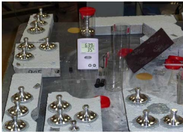
Figure 4.8: NETL samples with dollies epoxied in place ready for testing.
