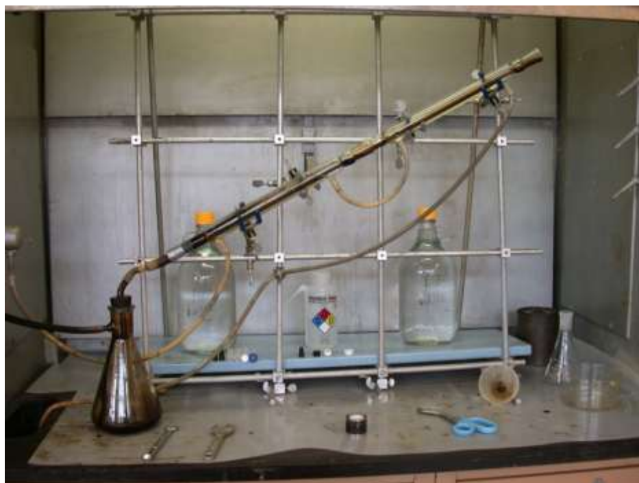
Fig. 18 - Secondary Collection Flask with Water-Cooled Condenser
