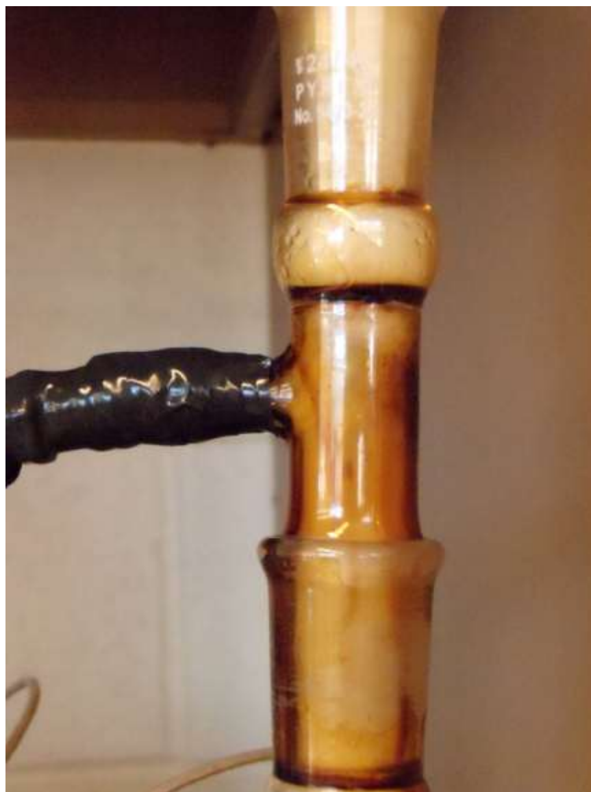
Fig. 24 - Off Products Collecting in Glass Fittings Above the First Collection Flask
