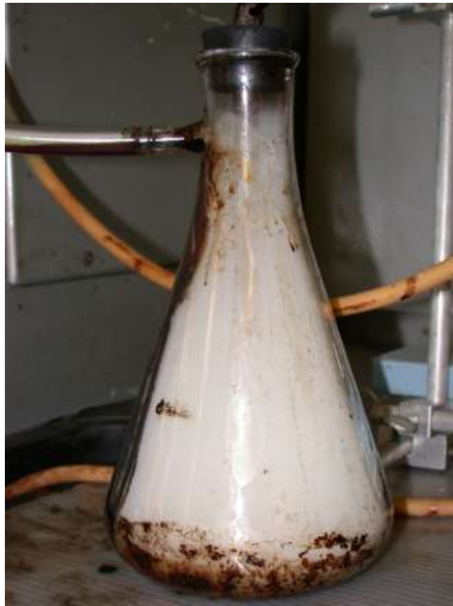
Fig. 19 - Secondary Collection Flask Filled with Dense Off Gas During the Initial Steps of Carbonization
