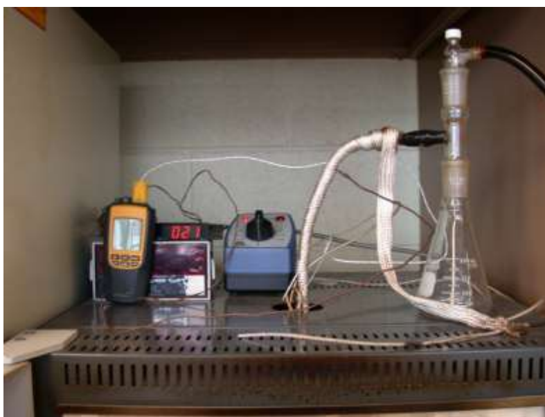
Fig. 17 - Heated Off Gas Piping and Thermocouples to Regulate Discharge Temperature
