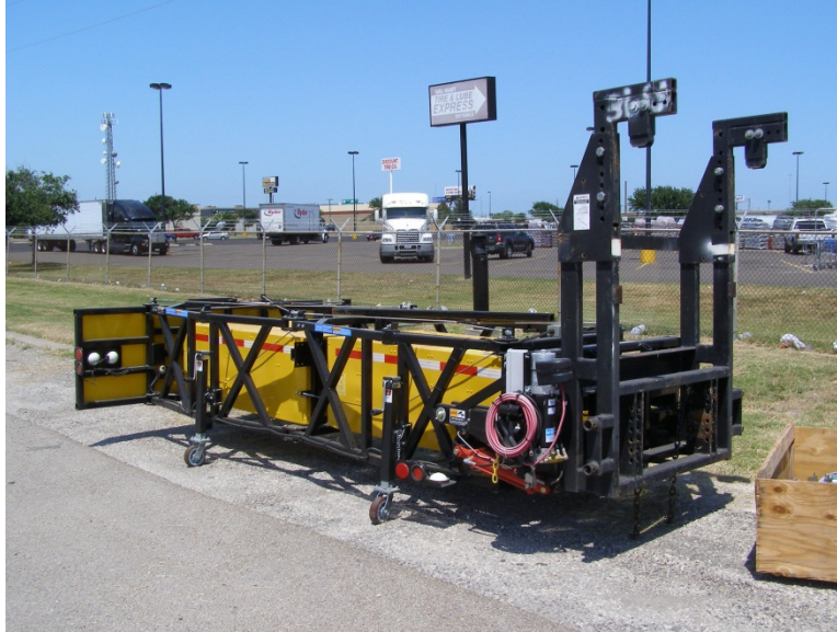
Figure 7. Safe-Stop Truck-Mounted Attenuator Tailgate Mount and Hydraulic Controls.
