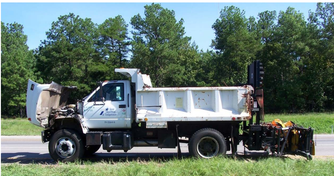
Figure 23. Post-Impact View of Arrow Panel on a Safe-Stop Truck-Mounted Attenuator.
