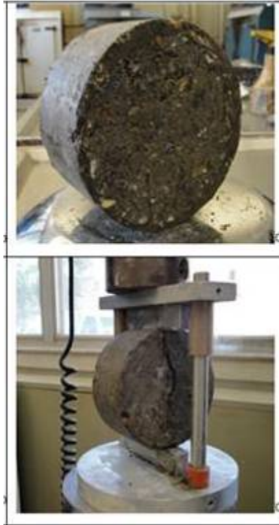
Figure 4.16. Tex-226-F, Indirect Tensile Strength (IDT) Test.
