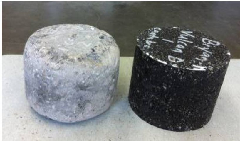
Figure 4.20. Lab Molded LRA Specimen Before and After Cantabro Test.
