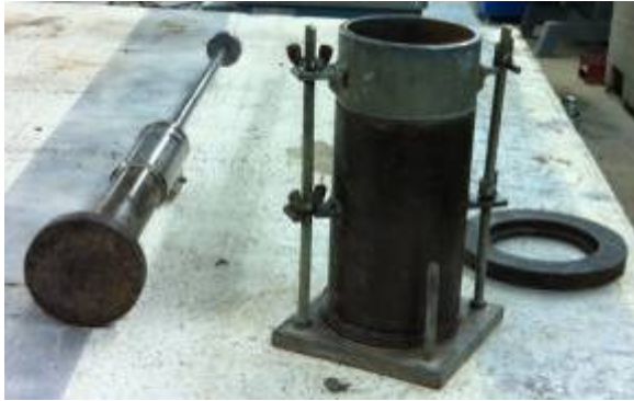
(a) Compaction Mold and Marshall Hammer
