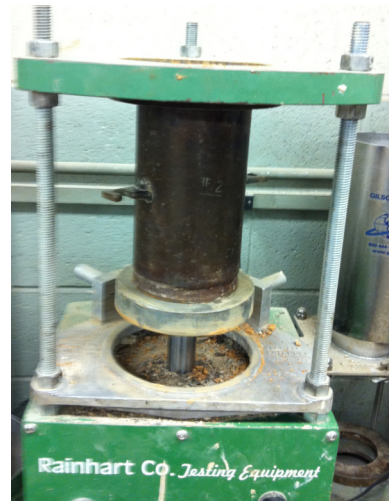
(b) TTI Specimen Extraction Process
