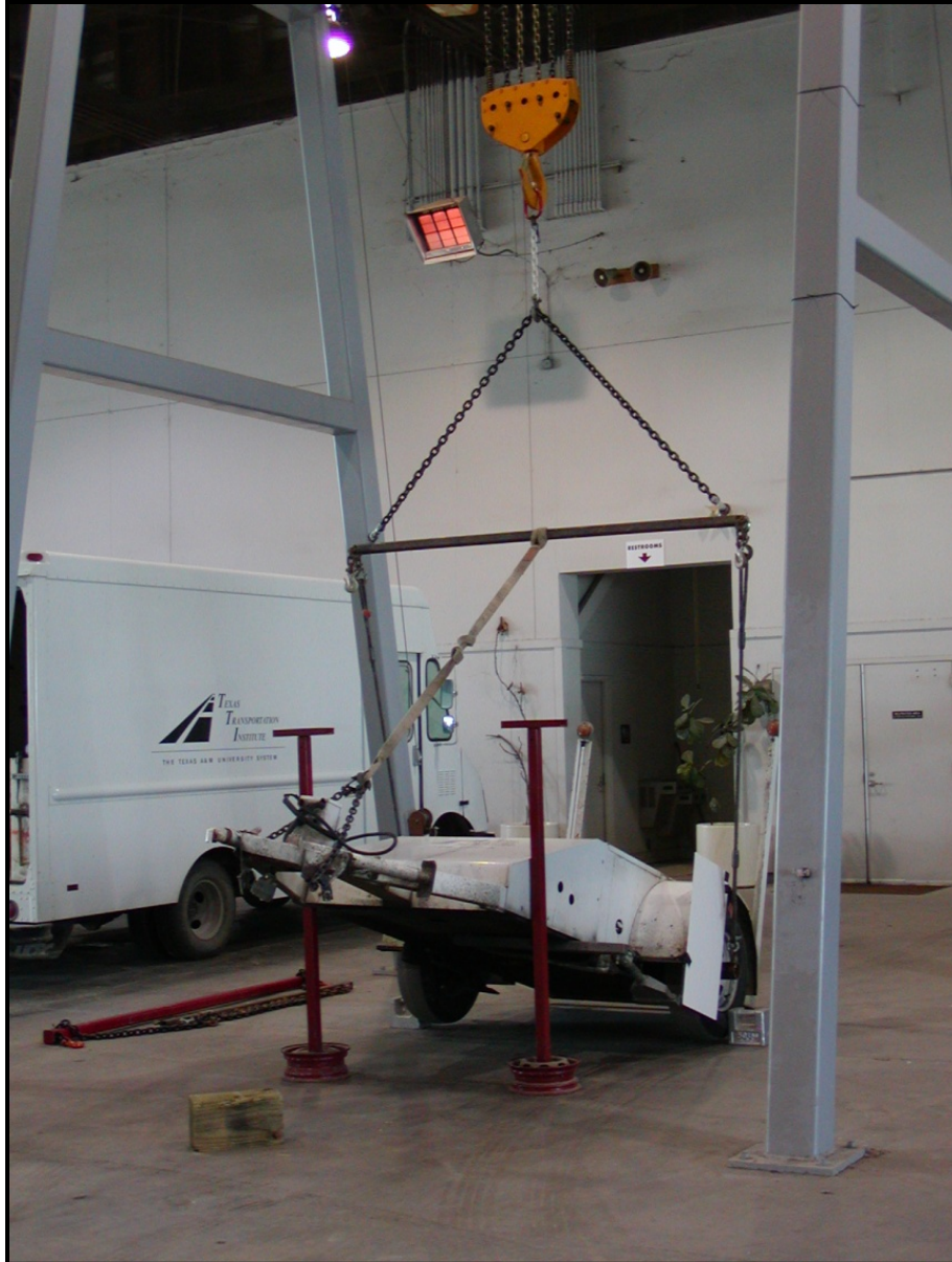
Figure 21. Measurement of the TxDOT E274 Trailer Center-of-Gravity.
