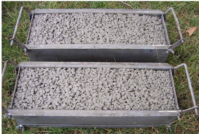
Figure 36. Fresh concrete with no curing compound
