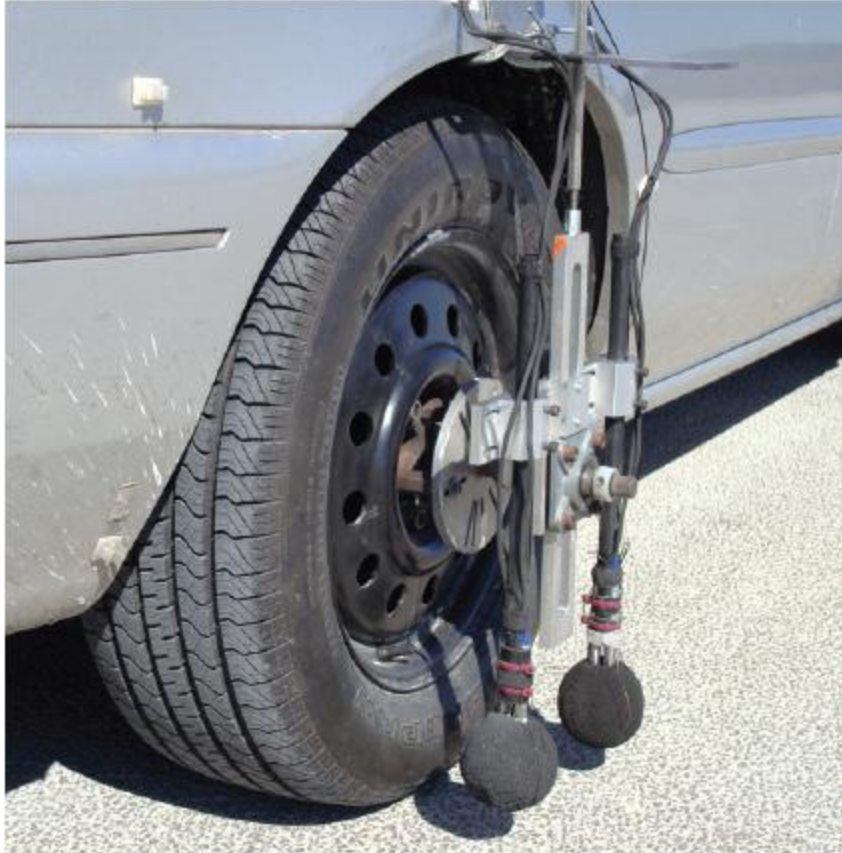
Figure 77. OBSI configuration with dual sound intensity probes (Rasmussen et al. 2011)
