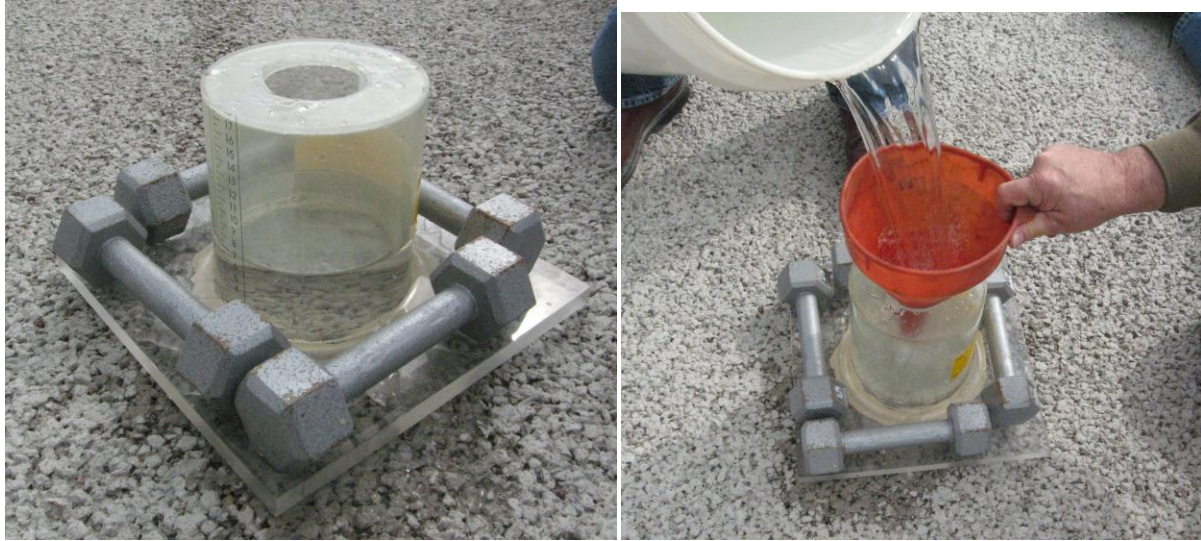
Figure 74. NCAT infiltration test device (2009)
