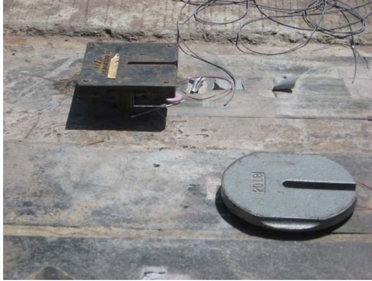
FIGURE 12 Weights Applied on Top of Each Installed Strain Gauge.
