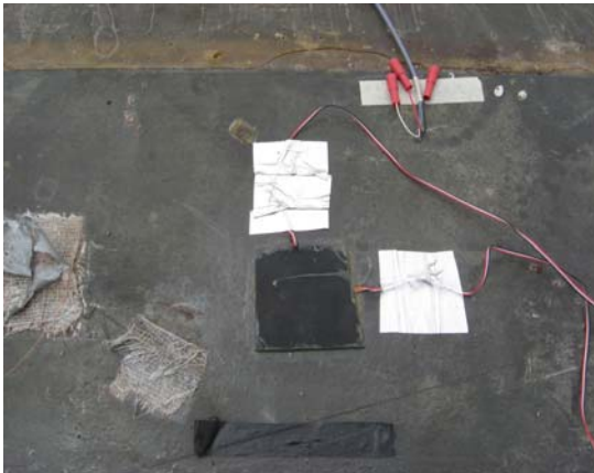
FIGURE 13 Covered Strain Gauges Attached to the FRP Sheets.
