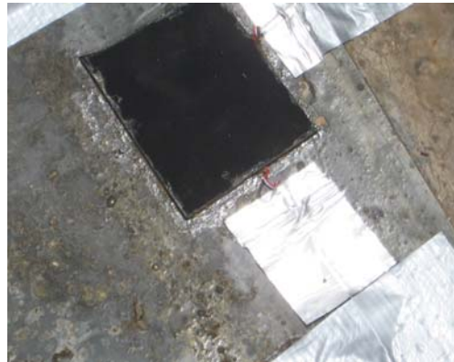
FIGURE 13 Covered Strain Gauges Attached to the FRP Sheets.
