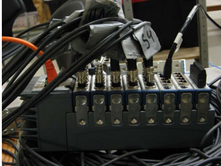
FIGURE 9 SDA System Showing the Analogue Modules Integrated on the SDA System by National Instrument.
