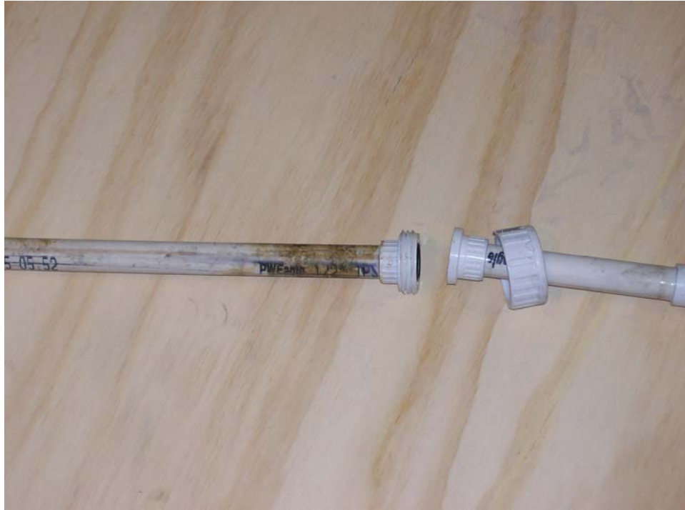
FIGURE A3 Compression connection.
