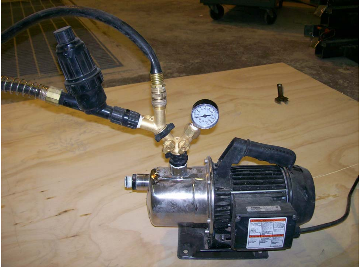
FIGURE A8 Pump with pressure gauge.
