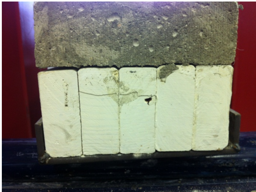
Figure 3.4 Typical block-shear failure (Specimen F11)
