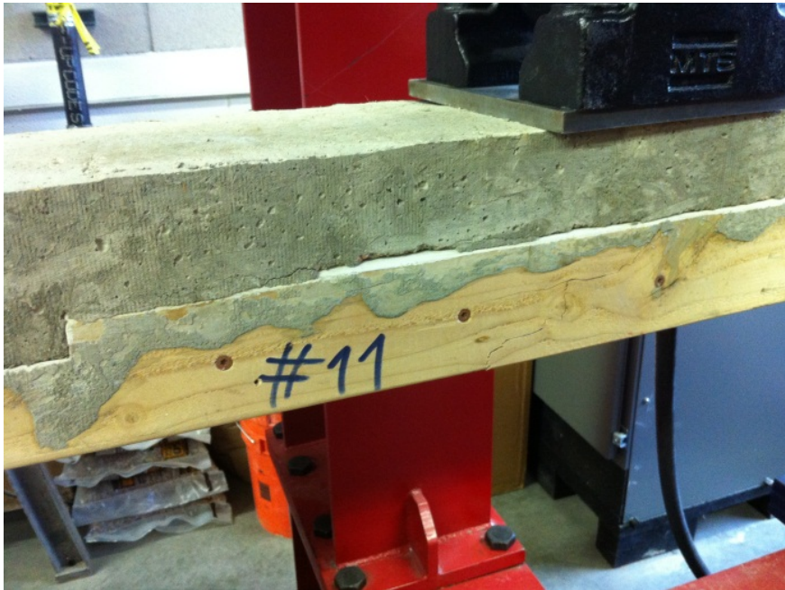
Figure 3.5 Typical tension failure (Specimen F11)
