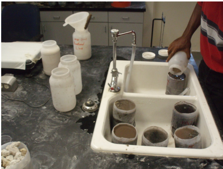
Figure 13: Half Gallon containers being loaded with sediments
