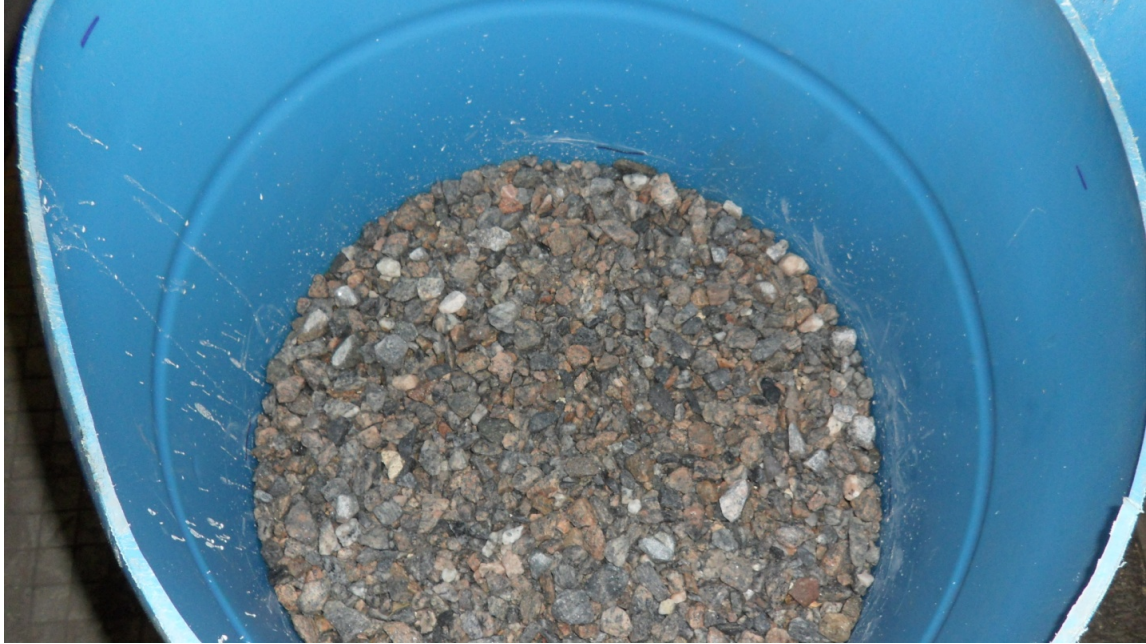
Figure 23: 5 Inches of #4 Stone Compacted
