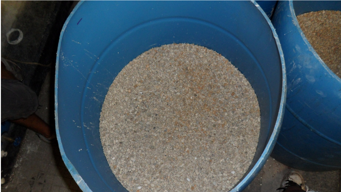
Figure 25: 2 inches of #89 Limerock
