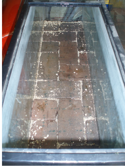
Figure 14: Brick paver (surface layer component) tested in large glass aquarium (12" x 19" x 47")
