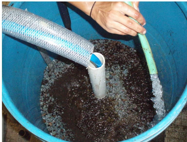
Figure 37: Washing loaded sediments into pores while pumping infiltrated water out through well pipe
