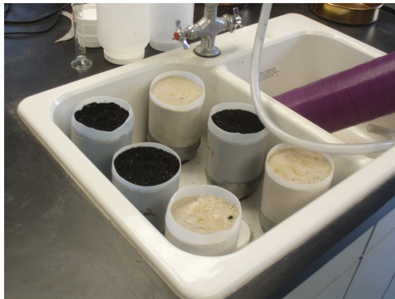
Figure 17: Half Gallon Jars draining by gravity
