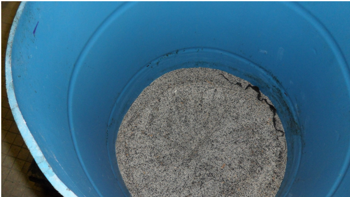
Figure 22: 4 Inches of Bold&Gold™ Pollution Control Media Installed
