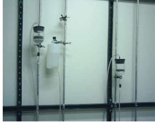
4.1(a) Hanging Column Test Setup
