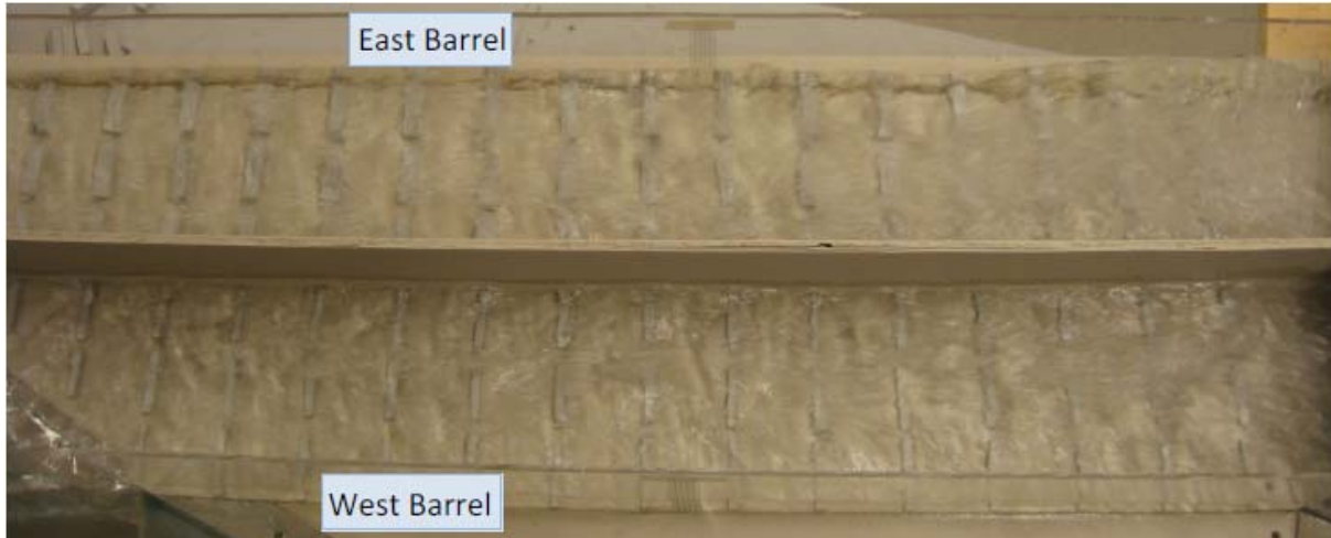
FIGURE 7: Second Model with Coarser Roughness Elements Added to East Barrel
