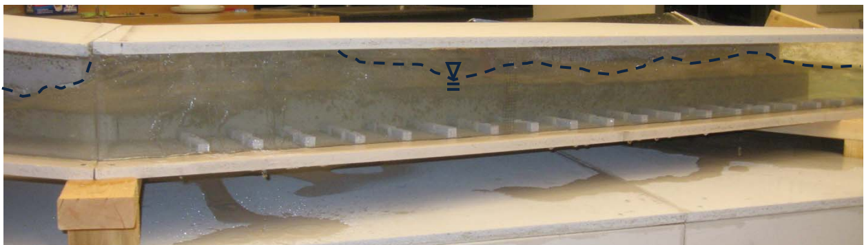
FIGURE 8: Second Model East Barrel Conveying 100-year Flow
