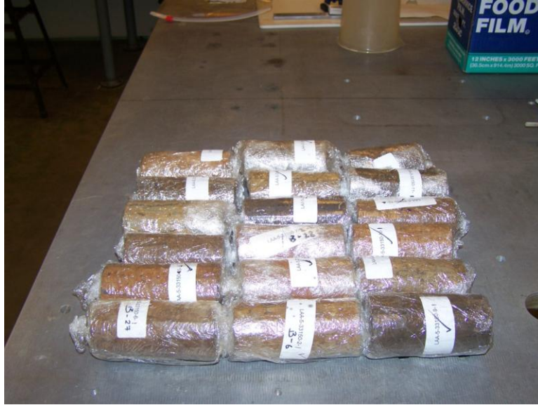
Figure 5 – All 18 In-Situ Specimens after Shear Testing
