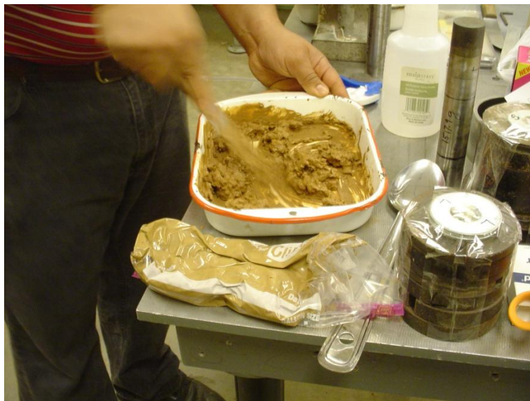
Figure 6 – Slurry Processing of Specimen
