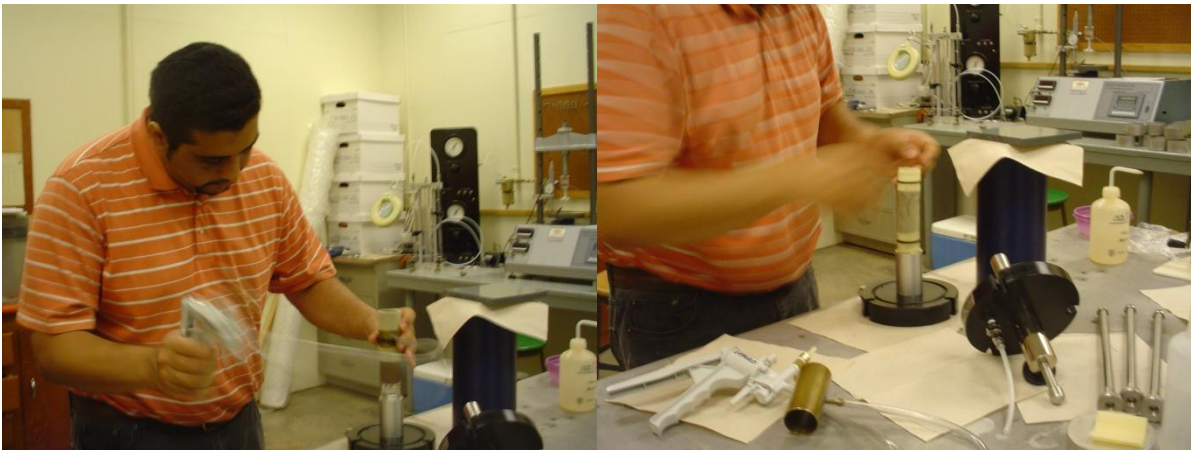
Figure 12 – Installing Membrane on Specimen
