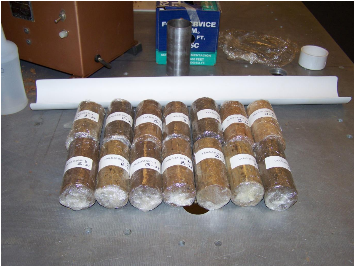
Figure 2 – Selected Specimens Trimmed in Length and Diameter
