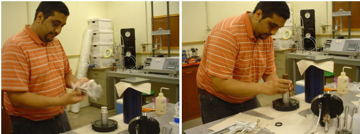
Figure 10 – Mounting Specimen on Triaxial Base
