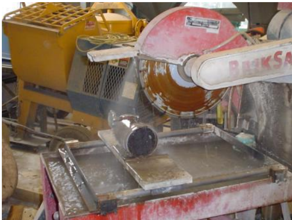
Figure 18. Sample being sawed to obtain parallel faces.
