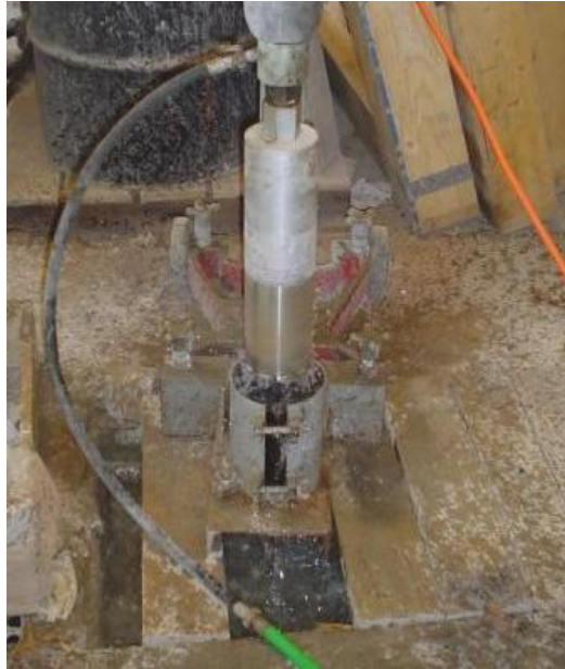
Figure 17. Sample being cored to required test diameter.
