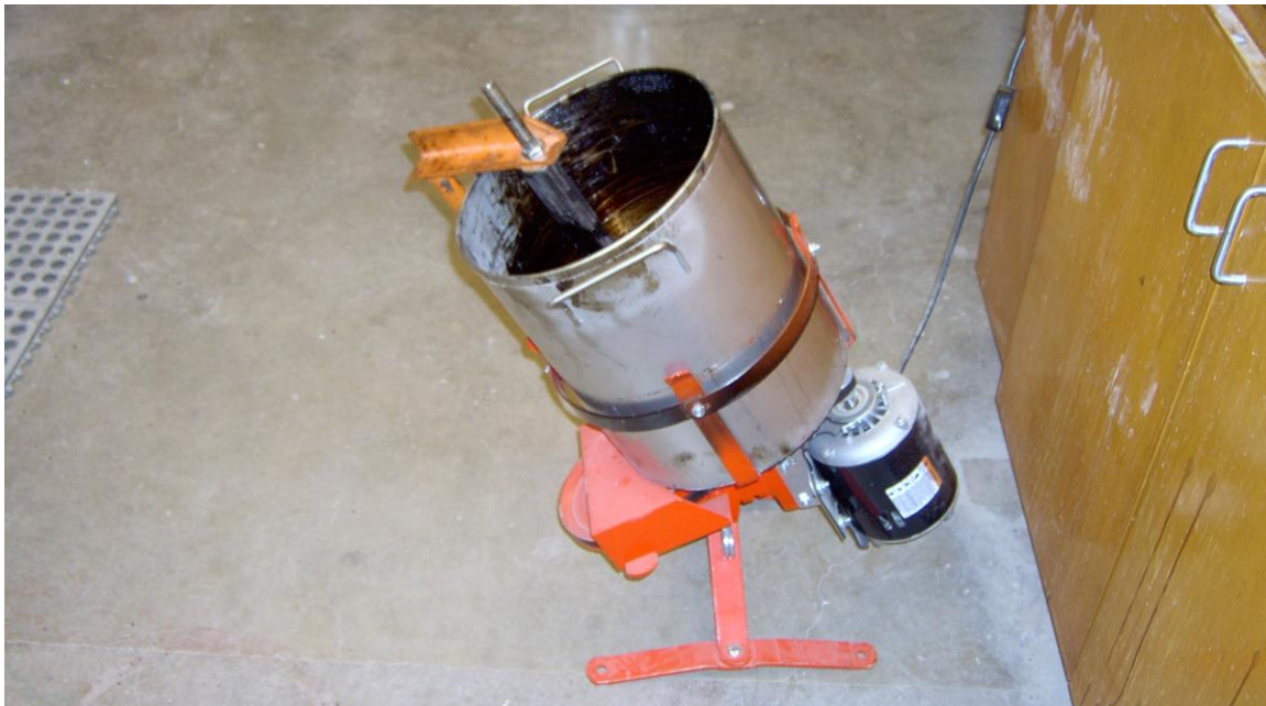
Figure 5. Bucket mixer used for mixing samples.
