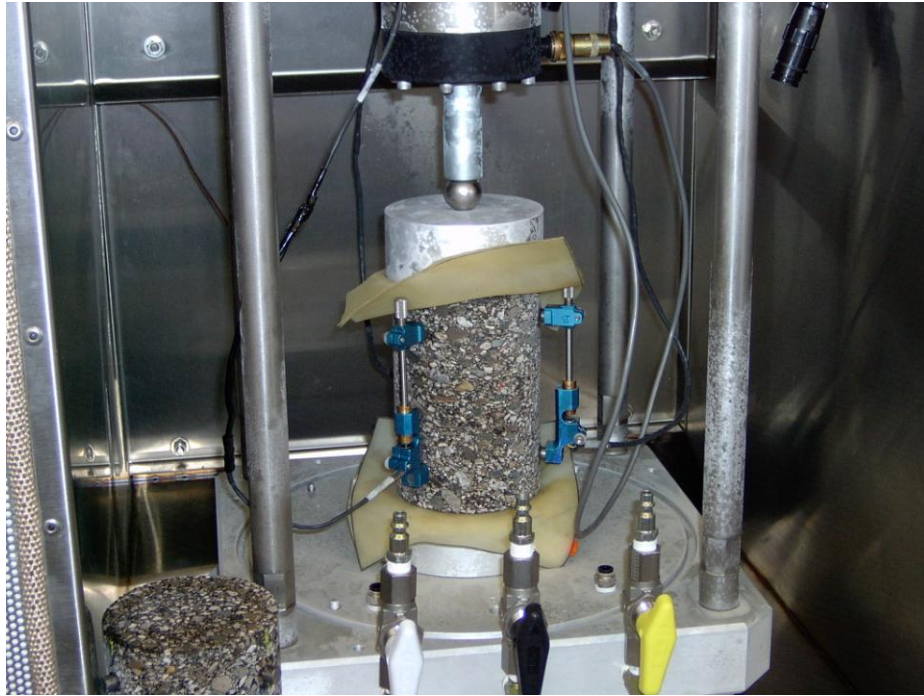
Figure 20. HMA sample ready for dynamic modulus testing.
