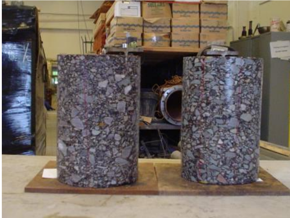
Figure 19. Test specimens for dynamic modulus testing.
