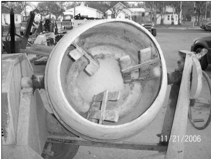
Figure 4.9 The Concrete Mixer Used for Preparing the SCC Laboratory Batches
