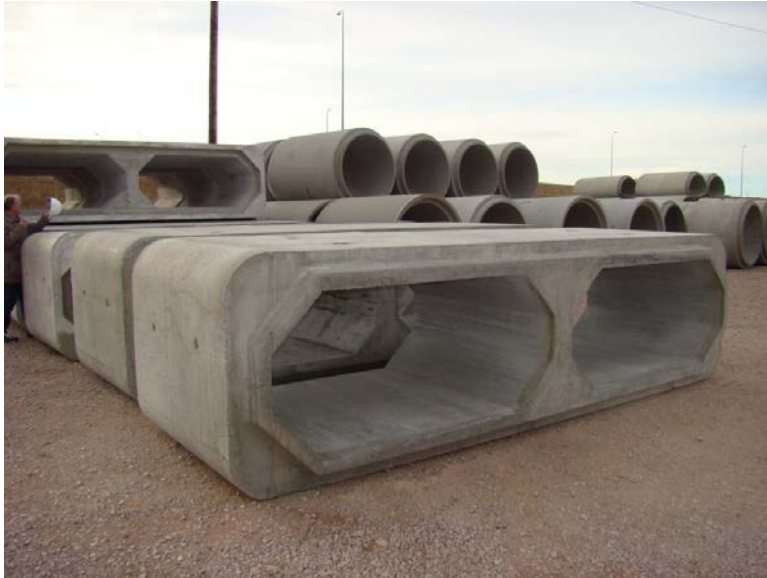
Figure 5.3 Completed SCC Box Culvert Units
