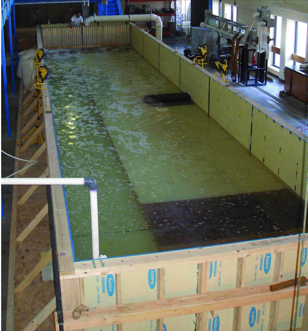
Figure 5.1 The water-sediment recirculating flume facility used for the experiments.
