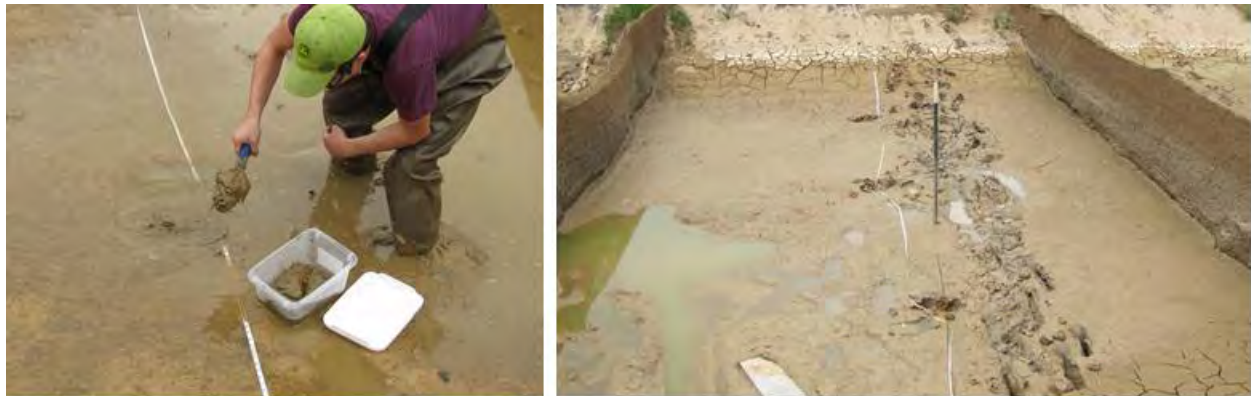
Figure 3.8: Sediment samples being taken from basin 4.
