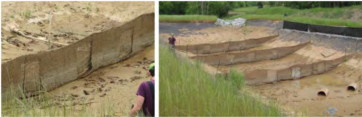
Figure 3.9: Three 4 ft 2 samples were taken from each baffle.
