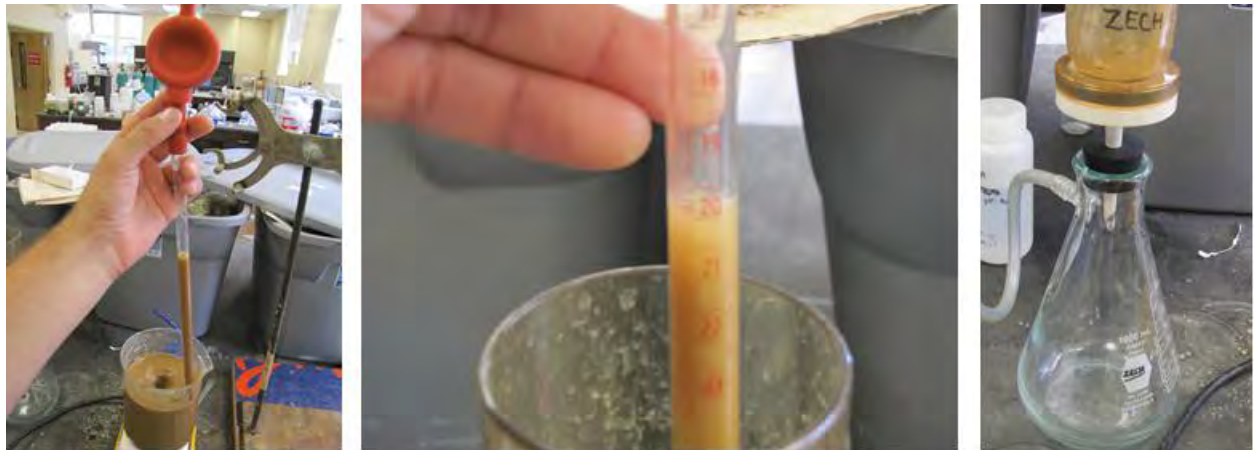
Figure 3.14: Drawing 20 mL of stormwater sample and running through vacuum filtration.
