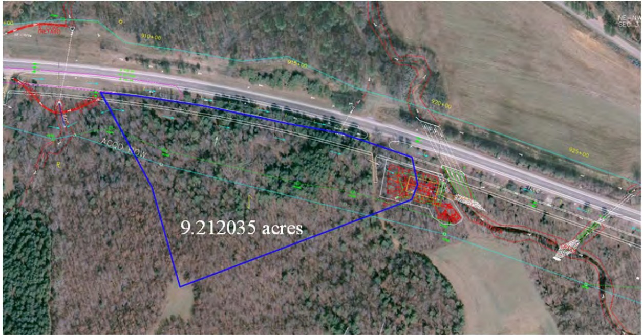
Figure 1.3: MicroStation overlay of sediment basin design and watershed area (aerial view of drainage area and sediment basin 4).
