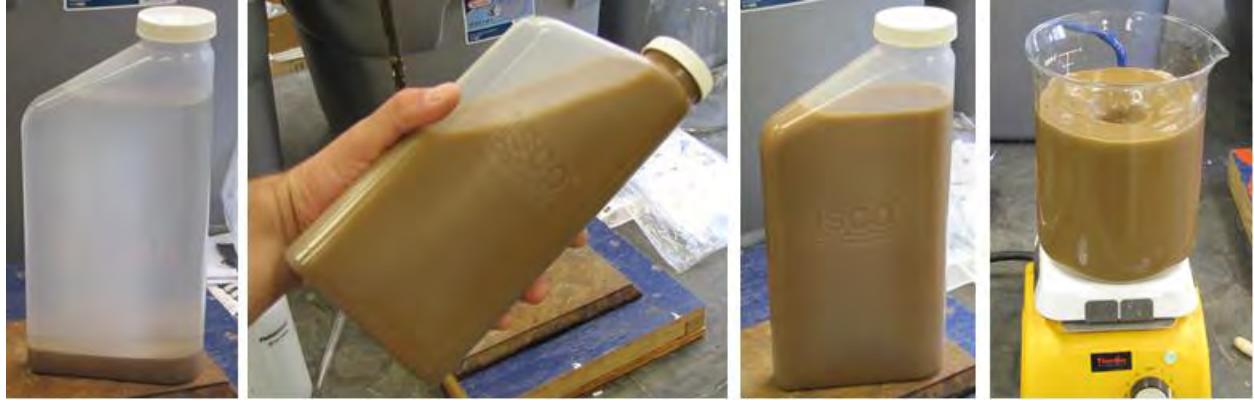
Figure 3.13: Ensuring sample is well mixed for sampling turbidity and TSS.
