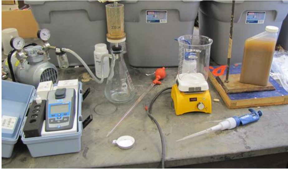
Figure 3.10: Turbidity and TSS laboratory analysis station.
